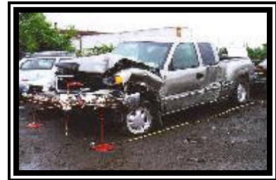
Figure 3. Frontal and left side damage to the 1999 GMC Sierra pickup truck.
