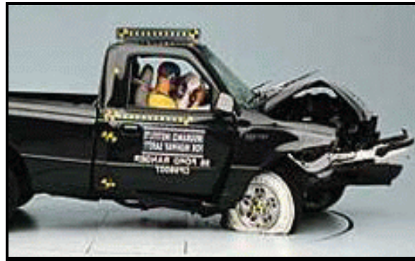
Figure 5. Adapted from IIHS photo depicting results of 40 mph frontal offset crash test with a 1998 Ford Ranger
