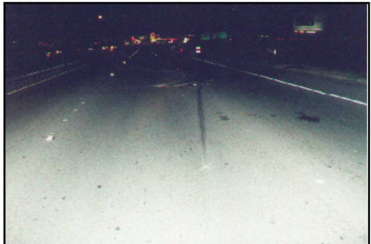
Figure 1. Pre-impact braking for Dodge pickup Point of impact in background—facing north.
