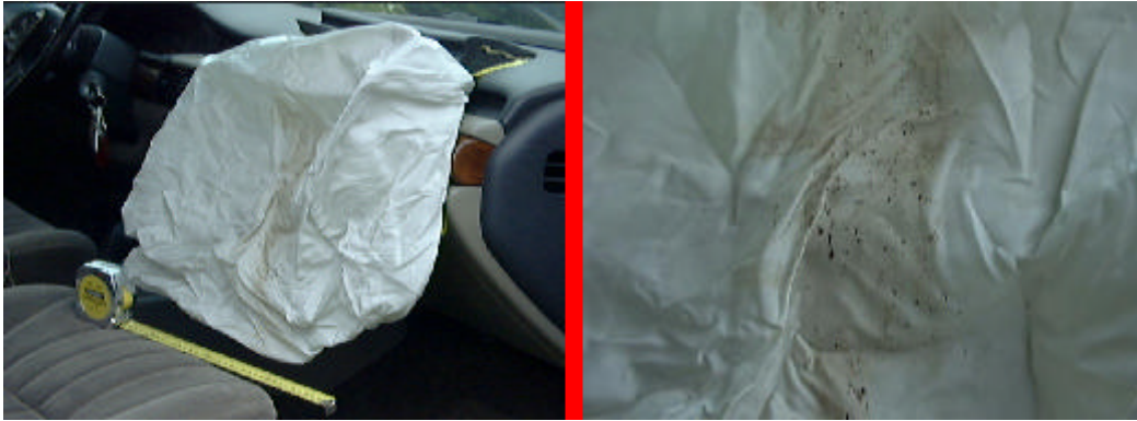
Figure 6 Overall and close-up view of the front right air bag showing the body tissue transfer related to contact with the child’s neck and facial area.
