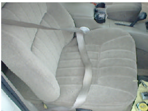
Figure 12 View of the front right continuous loop lap and torso restraint belt
