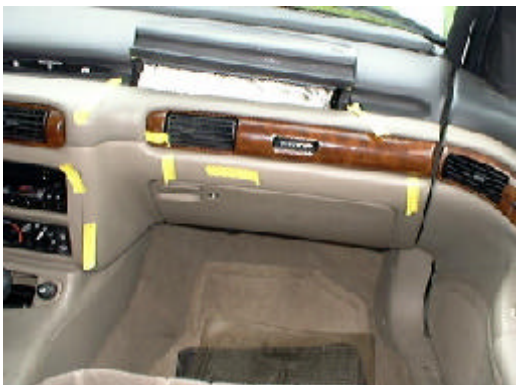
Figure 9 View of contact evidence along the front right instrument panel
