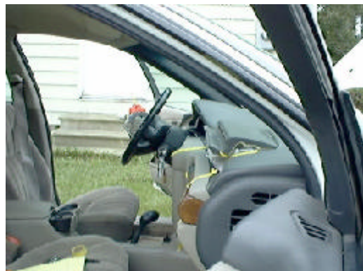
Figure 18 Lateral view of the right instrument panel highlighting the location of the front right air bag module cover to the leading edge of the instrument panel
