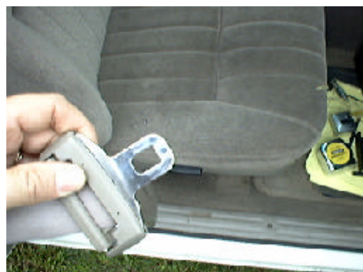
Figure 13 View of usage related score marks on the front right restraint belt latch plate
