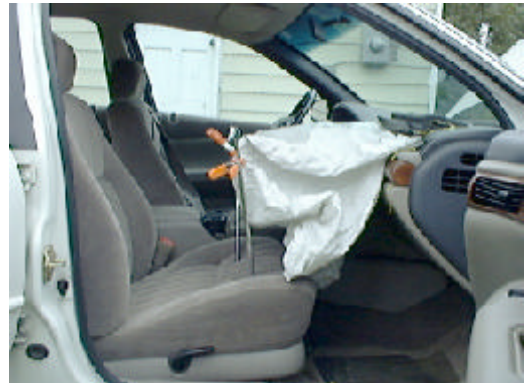
Figure 11 Lateral view of the front seat area showing the relative seat adjustment location and front right air bag excursion
