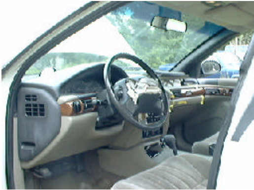
Figure 15 View of the front left instrument panel and air bag module cover
