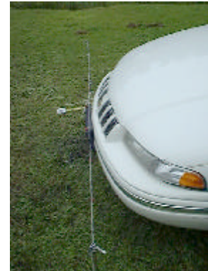
Figure 8 Lateral view of the frontal plane showing the extent of rearward displacement
