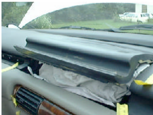
Figure 17 View of the front right air bag module cover (artifacts shown in the photograph along the leading edge were related to post crash activities)
