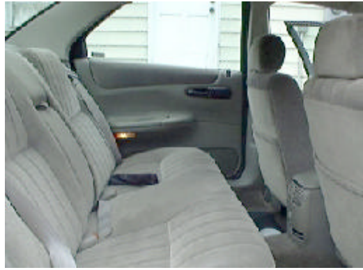
Figure 14 View of the rear seat area of the Chrysler showing the availability of the outboard lap and torso belts and the non availability of the center lap restraint belt
