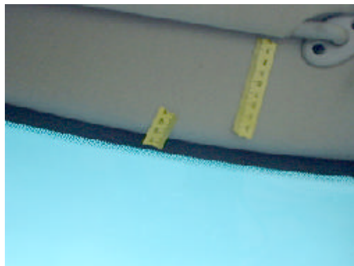
Figure 10 View of scattered tissue transfer along the right windshield header area
