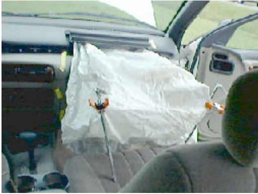
Figure 19 View of the front right air bag showing the relationship between the air bag excursion and the leading edge of the seat cushion
