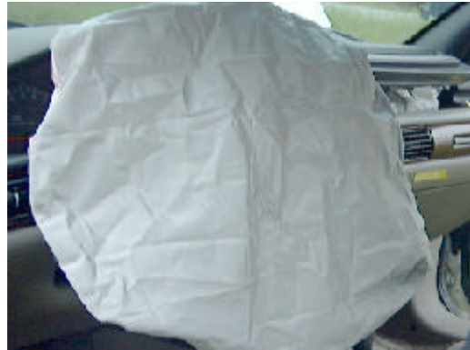
Figure 16 View of the front left air bag
