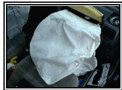
Figure 9. Vertically oriented tissue transfer on the front right air bag.
