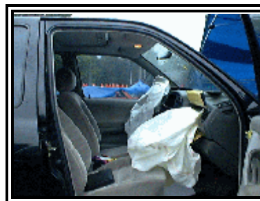
Figure 12. Occupant trajectory and deployment path of the front right air bag.
