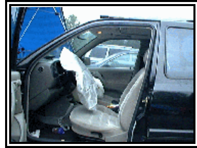
Figure 6. Overall view of the driver's seated position and the deployed front left air bag.
