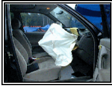
Figure 7. View of the deployed front right passenger air bag.
