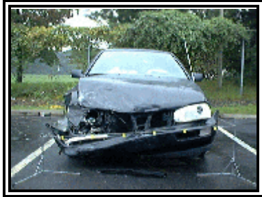
Figure 3. Frontal damage pattern to the Volkswagen Golf.
