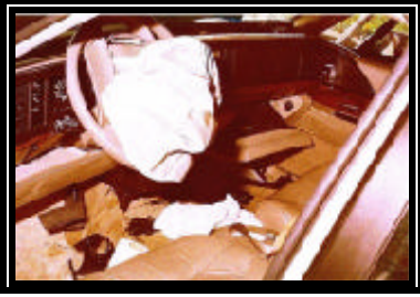
Figure 6. Interior view showing damage to the knee bolster and steering column
