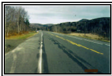
Figure 2. Northbound approach for the tractor/semi-trailer prior to steering inputs showing skid marks from power unit and trailer
