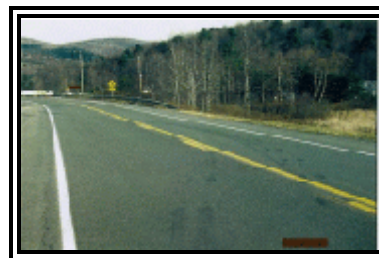
Figure 3. Northbound approach for the tractor/semi-trailer showing skid marks from attempted avoidance maneuvers
