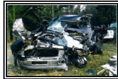
Figure 8. Frontal view of exterior damage to the Dodge pickup truck
