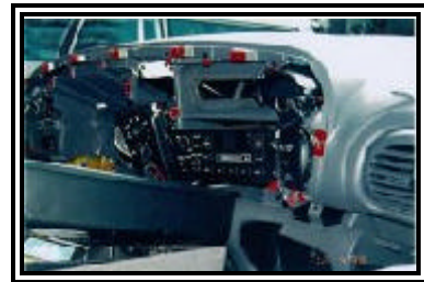
Figure 11. Instrument panel showing deformation and front right passenger's air bag cut off switch
