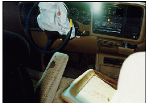
Figure 12: Case vehicle's driver seating area showing compressed steering wheel, driver's blood stained right armrest, and distorted center console cover (case photo #22)
