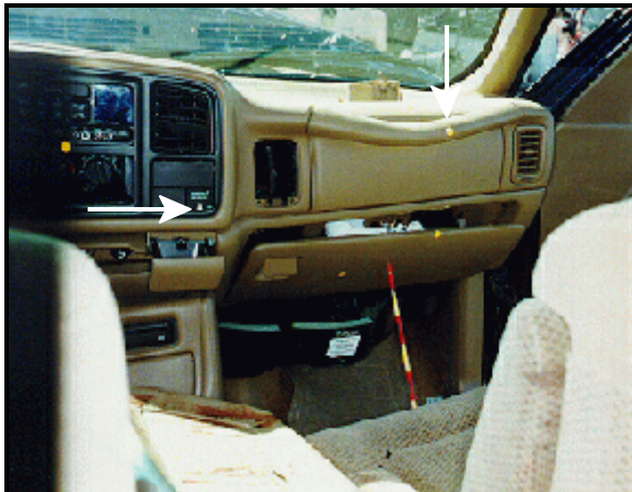
Figure 13: Case vehicle's front right seating area showing suspected occupant contacts to glove box door and oblong hand rail atop of front right air bag module; Note: arrows highlight rail contact and air bag cutoff switch (case photo #25)
