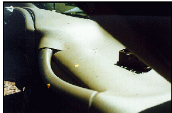
Figure 14: Close-up of contact evidence on oblong hand rail atop of case vehicle's front right air bag module (case photo #27)
