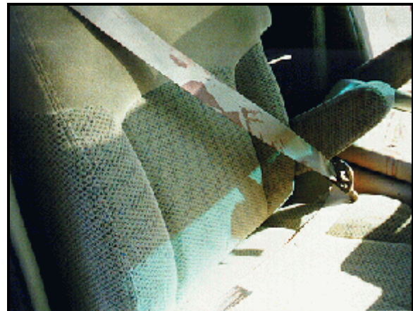
Figure 16: Case vehicle's front right safety belt showing blood stains on torso portion of webbing (case photo #31)
