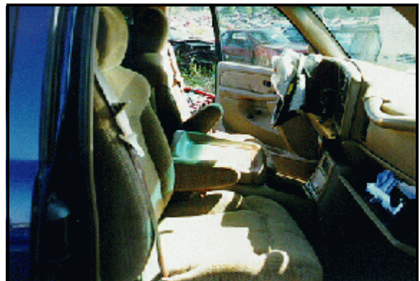
Figure 11: Case vehicle's front seating area showing steering column compressed against instrument panel and distorted center console cover (case photo #26)
