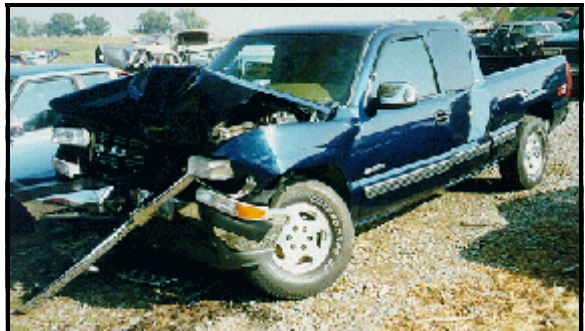
Figure 6: Case vehicle's frontal damage viewed from left of front; Note: induced damage to left fender and left side of extended cab (case photo #08)
