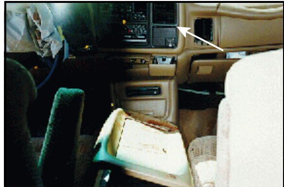
Figure 5: Case vehicle's center instrument panel showing passenger air bag activation switch (arrow) in "off" position; Note: distorted center console's cover (case photo #23)
