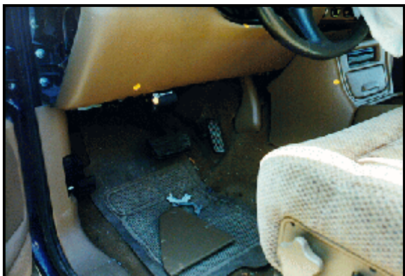
Figure 7: Evidence of occupant contact on case vehicle's left knee bolster and center instrument panel (case photo #19)
