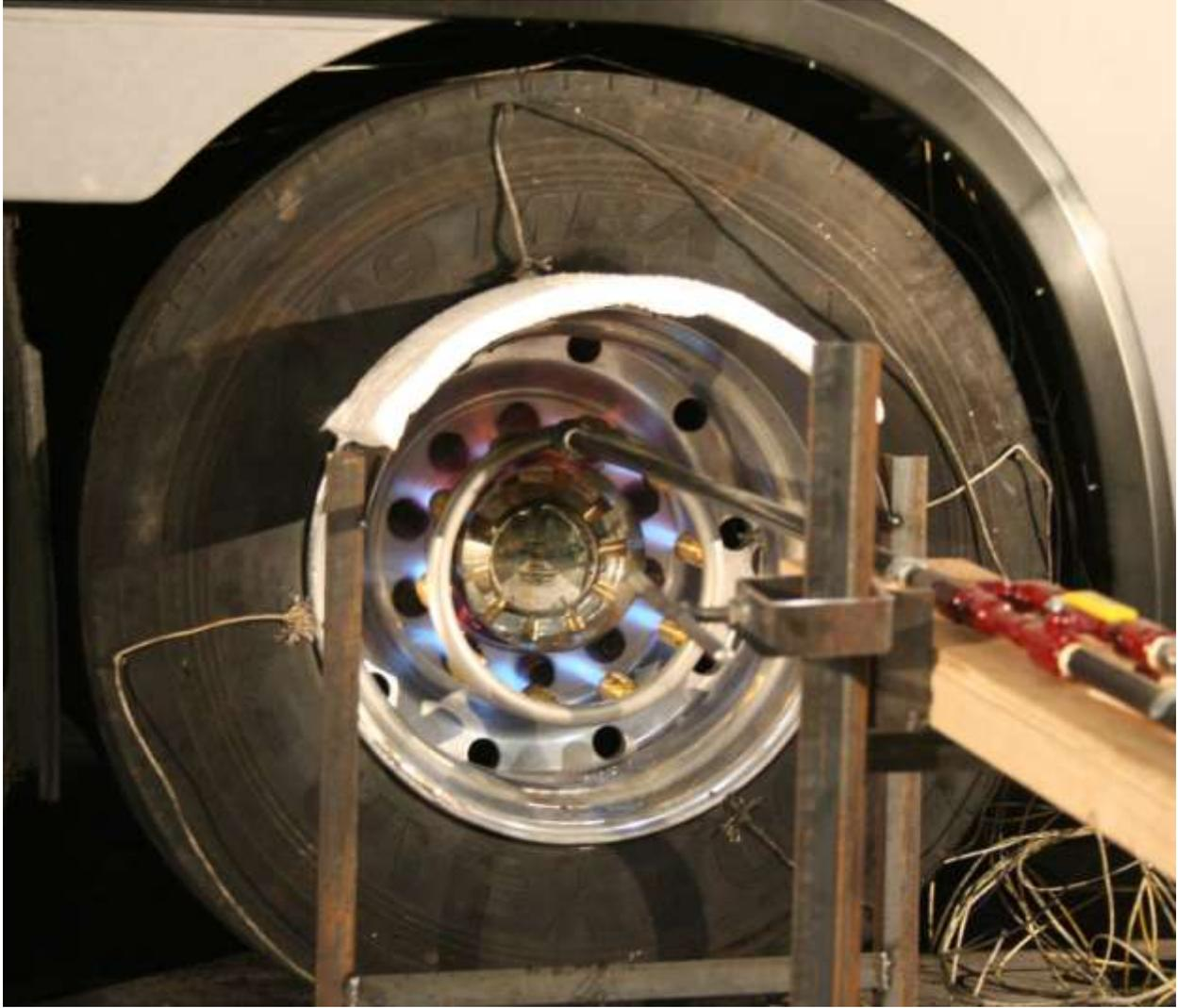
**Figure 112 Close up view of burner near beginning of drive axle wheel heating penetration experiment.**
