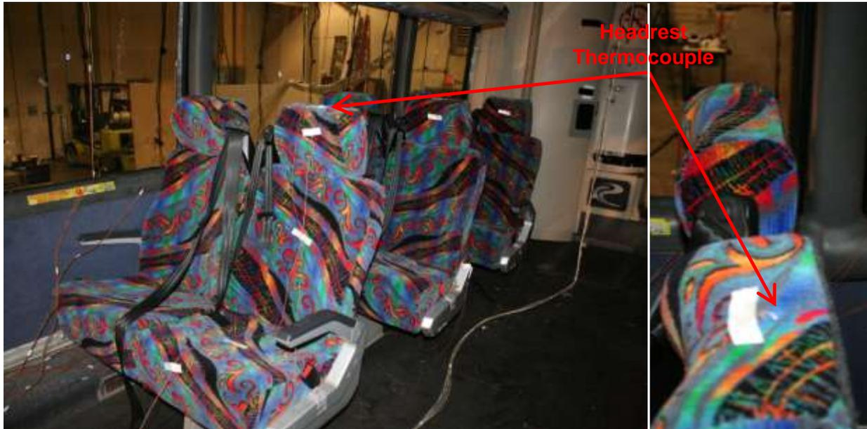
**Figure 20** Two photographs showing the three pairs of seats installed for the tenability experiments. The right photograph shows one of the thermocouples installed on the top of an aisle seat headrest.
