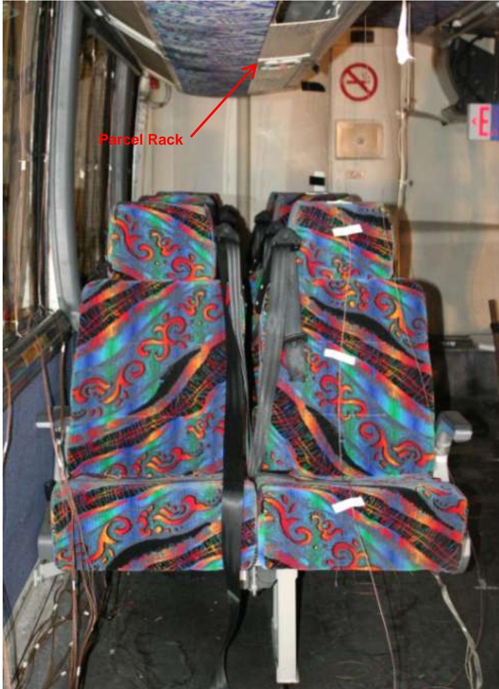
**Figure 14 A** photograph of the seats and parcel rack installed for the tenability experiment.
