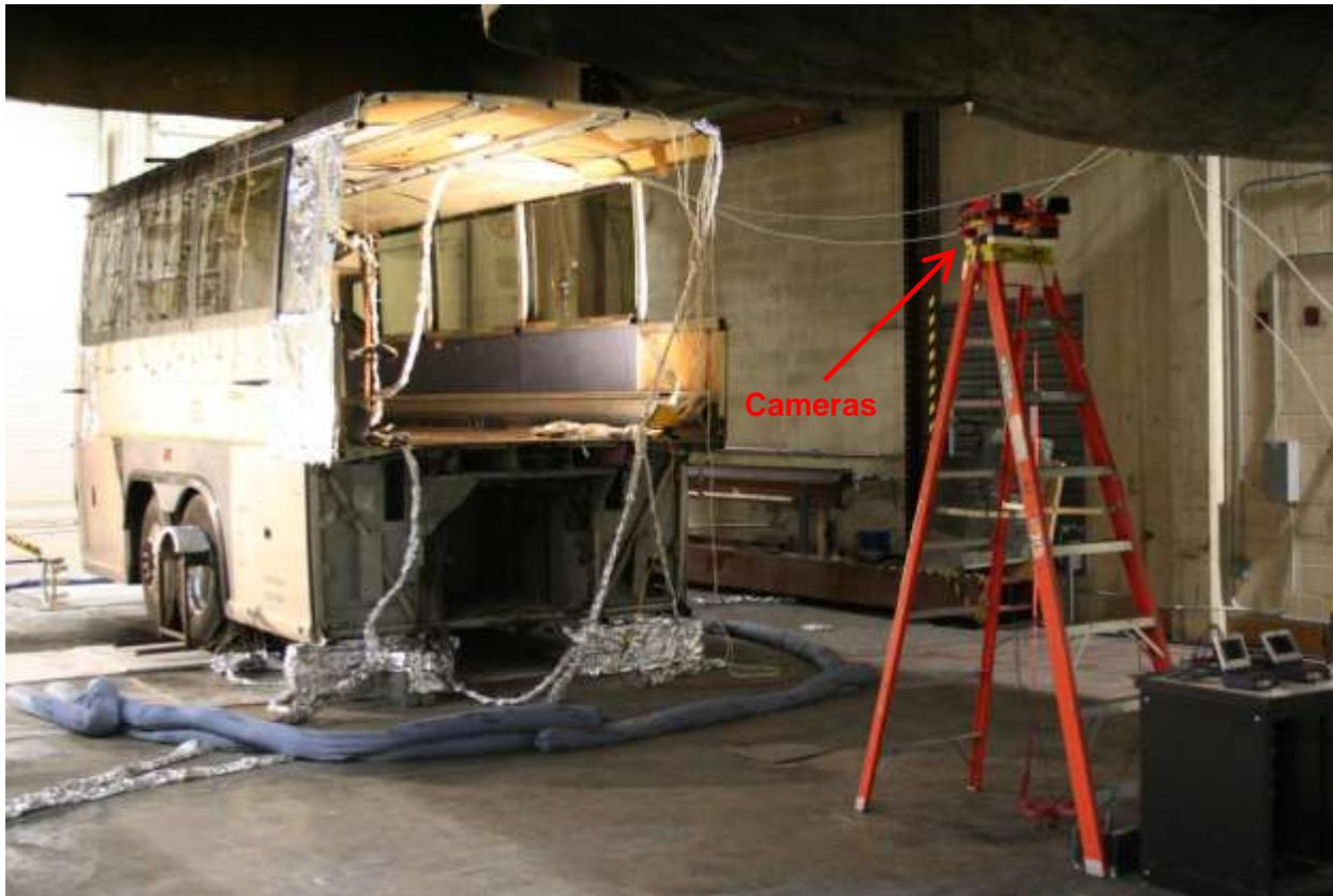
**Figure 29** Photograph of the two IR cameras viewing the open end of the motorcoach for penetration and hardening experiments. One camera was set to IR and the other to visual mode for comparison.
