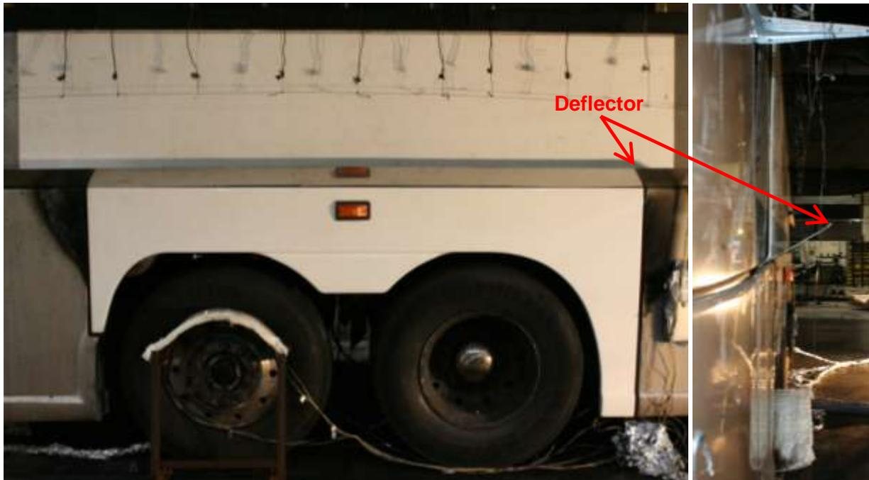
**Figure 11** Photographs of the deflector installed between the fender and exterior side panel. The left photo shows a view of the side of the motorcoach. The right photo shows an end view from the rear.
