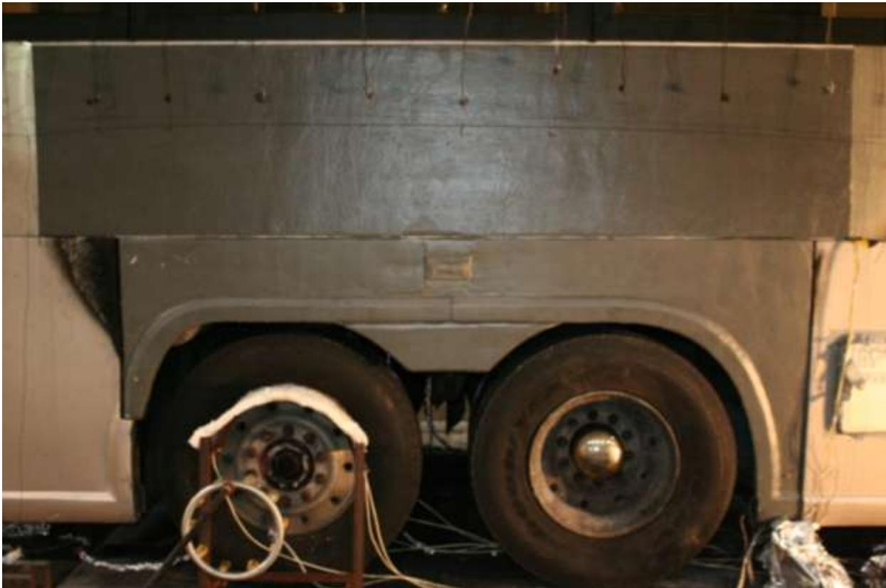
**Figure 9** A photograph of the fender and exterior side panel with an intumescent coating.
