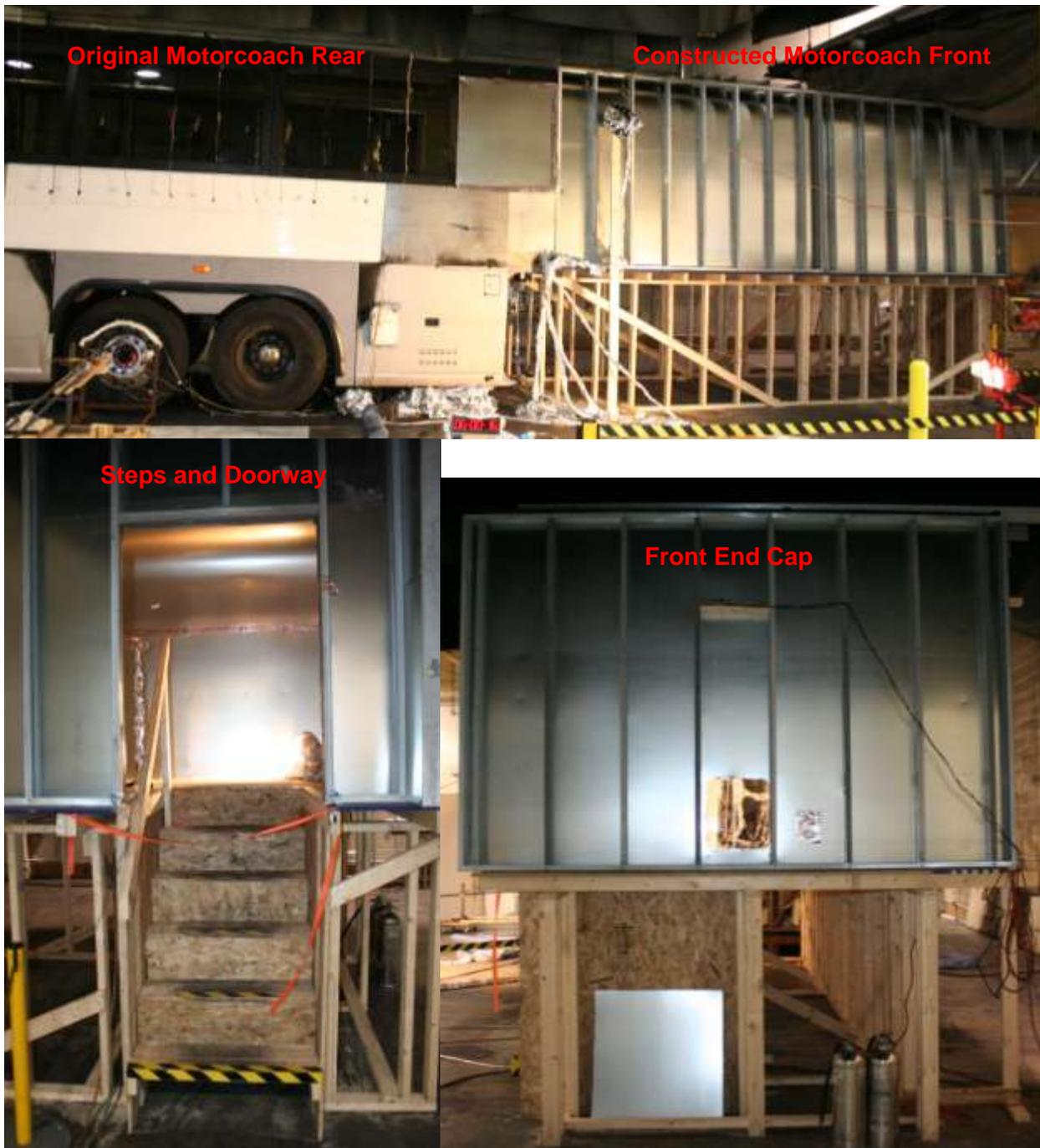
**Figure 13** Photographs of the motorcoach extension. The top photo shows most of the assembly of the original motorcoach rear half and added front extension. The bottom left photo shows the extension doorway and steps. The bottom right photo shows the front end with the window and visibility camera.
