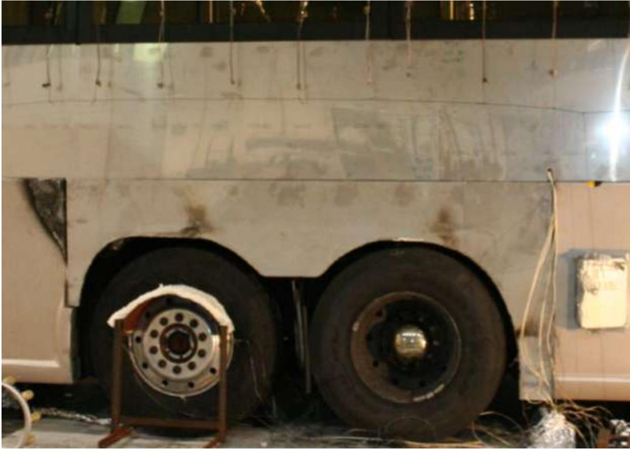
**Figure 7 A photograph of the fender and exterior side panel replaced with sheet metal.**
