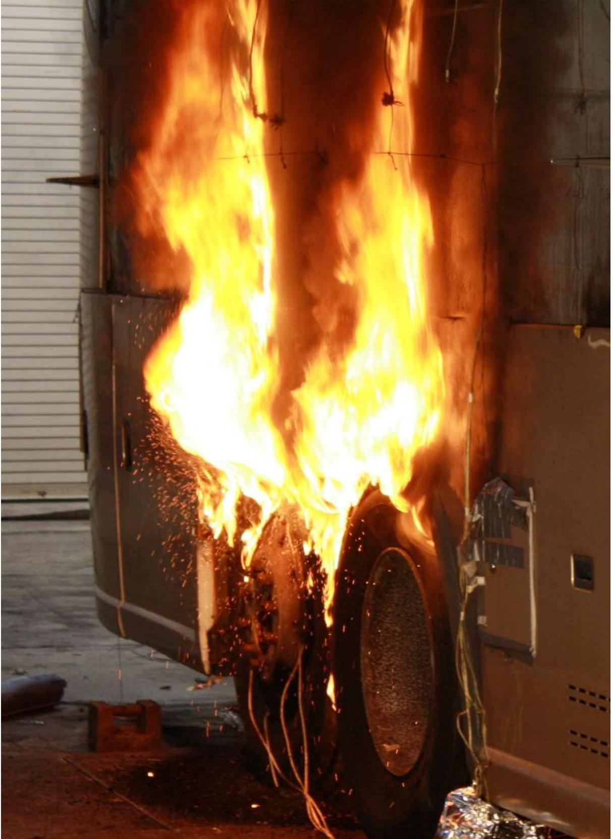
**Figure 75 Intumescent coating fire-hardening experiment about 28 min after burner removal.**
