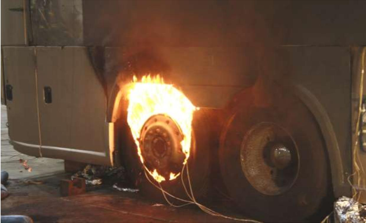
**Figure 72 Intumescent coating fire-hardening experiment about 4 min after burner removal.**
