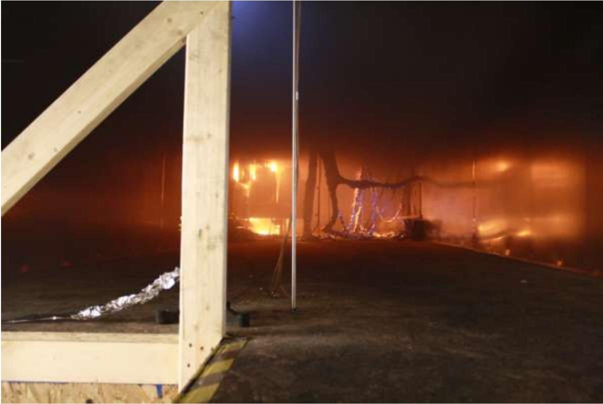
**Figure 87 Tenability experiment passenger compartment about 15 min after burner removal.**
