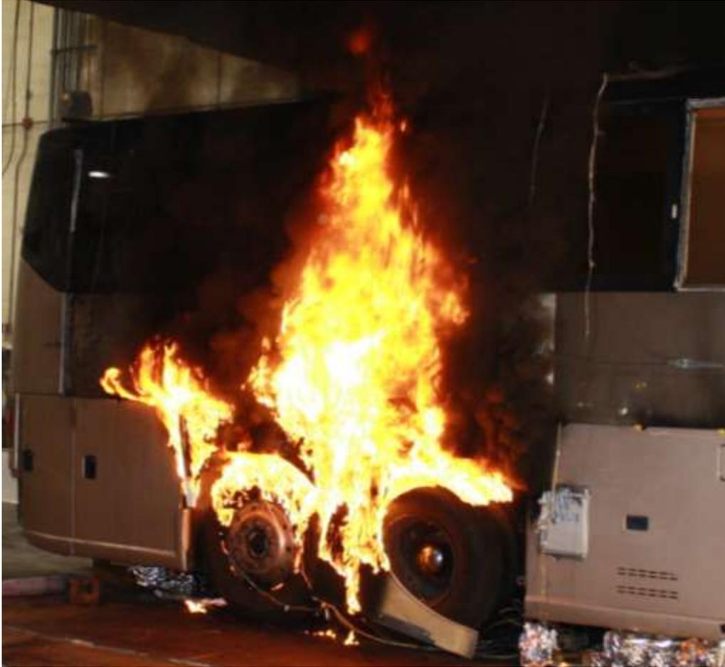
**Figure 78 Steel deflector fire-hardening experiment about 8 min after burner removal.**
