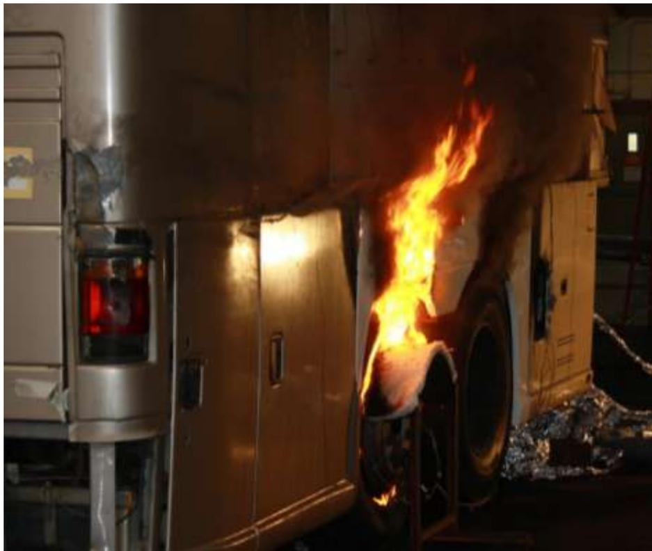
**Figure 77 Steel deflector fire-hardening experiment about 2 min after burner removal.**
