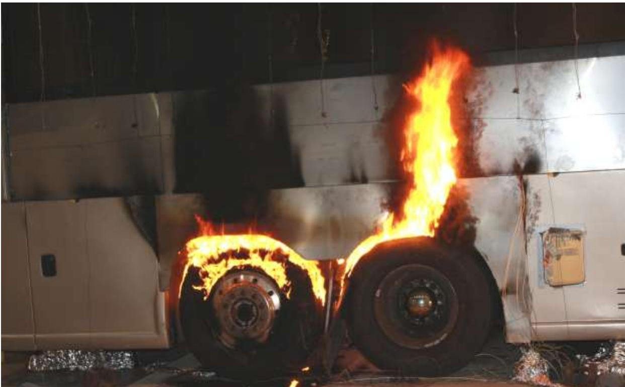
**Figure 71 Steel exterior panel fire-hardening experiment about 39 min after burner removal.**
