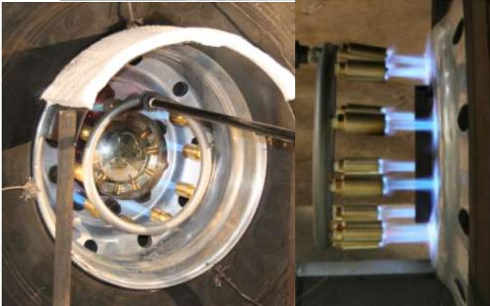
**Figure 5** The burner for heating the wheels. The top photograph shows the whole assembly including the burner ring, wheeled cart, and gas and air valves. The bottom right photograph shows the pre-mixed natural gas and air torches impinging on a tag axle wheel. The bottom left photograph shows the tire shield nested inside a drive axle wheel rim with an insulating cover to minimize convective and radiative heating to the tire from the shield.
