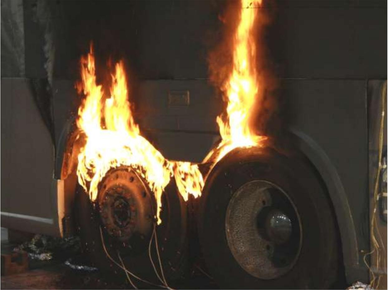
**Figure 74 Intumescent coating fire-hardening experiment about 19 min after burner removal.**
