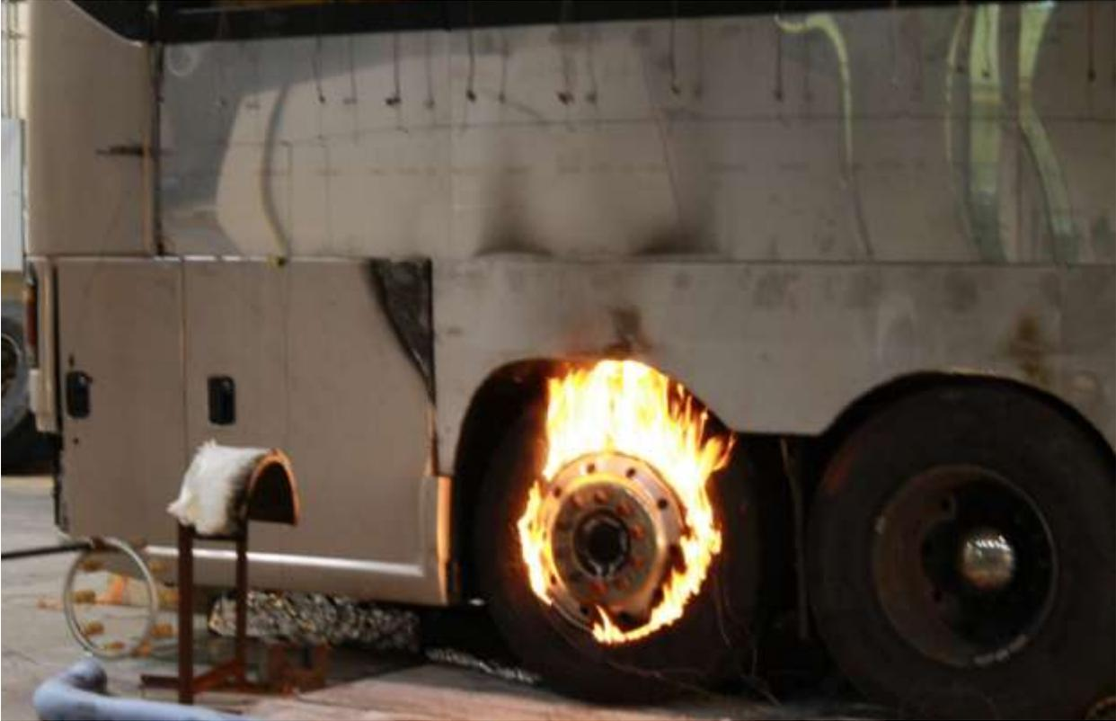
**Figure 70 Steel exterior panel fire-hardening experiment about 8 min after burner removal.**
