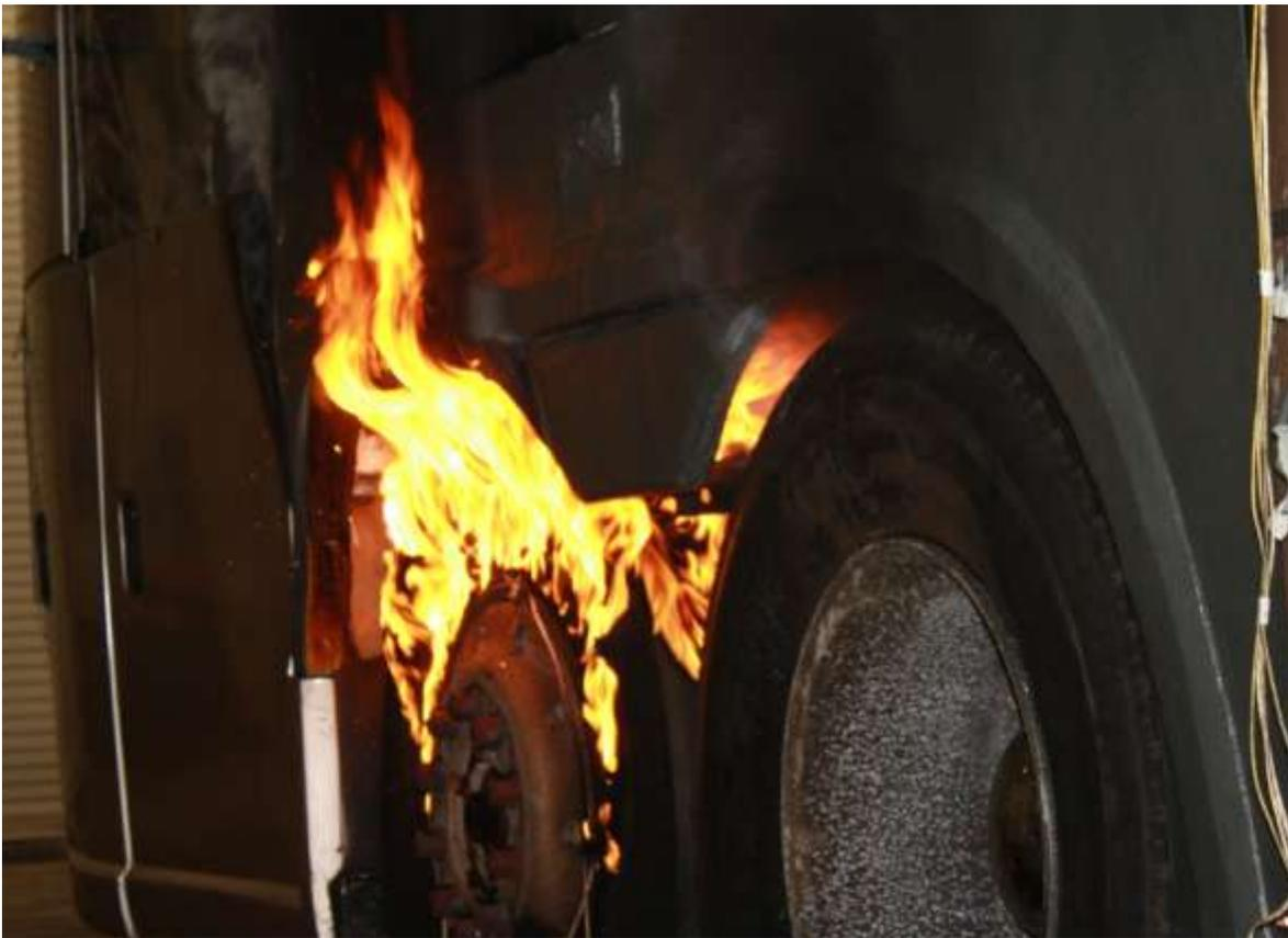
**Figure 73 Intumescent coating fire-hardening experiment about 6 min after burner removal.**
