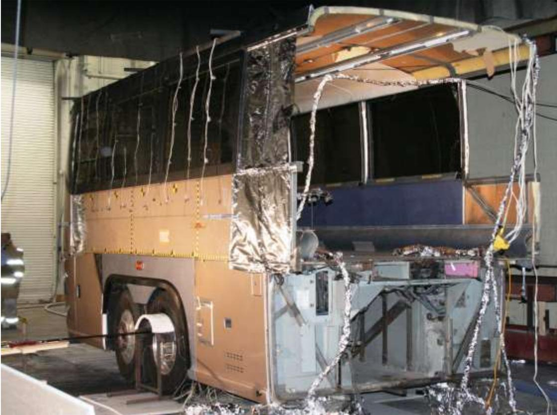
**Figure 110 Motorcoach ready for start of drive axle wheel heating penetration experiment.**
