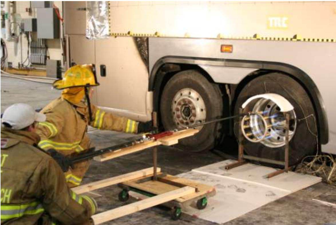
**Figure 111 Positioning of burner for drive axle wheel heating penetration experiment.**
