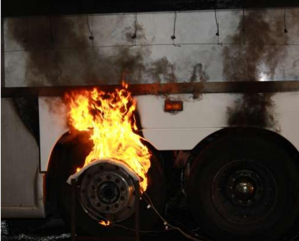
**Figure 76 Steel deflector fire-hardening experiment about 1 min after burner removal.**
