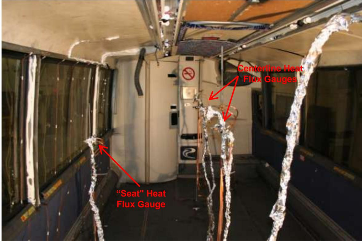
Figure 22 From the penetration experiments, a photograph of the interior of the motorcoach showing the locations of the heat flux gauges.
