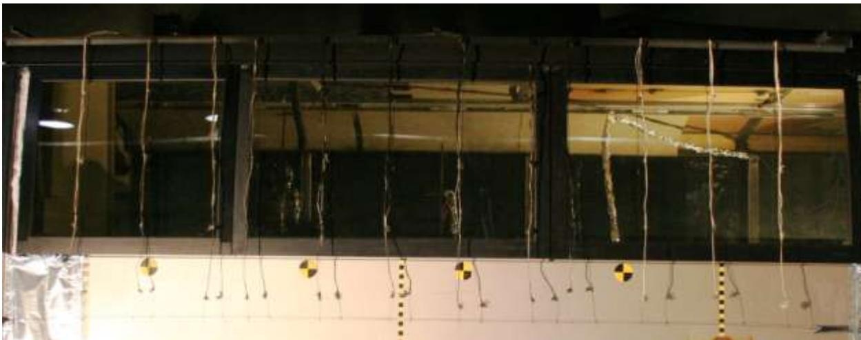
Figure 16 A schematic (top) and photograph (bottom) of the exterior grid of thermocouples on the motorcoach windows. The blue rectangles represent window outlines, red dots represent TCs, green areas represent window frames and post centerlines. Labels pertain to designations in the data file. The pattern of thermocouple labeling is shown in red with O for outside grid, the 1<sup>st</sup> number for column, and the 2<sup>nd</sup> number for row.
