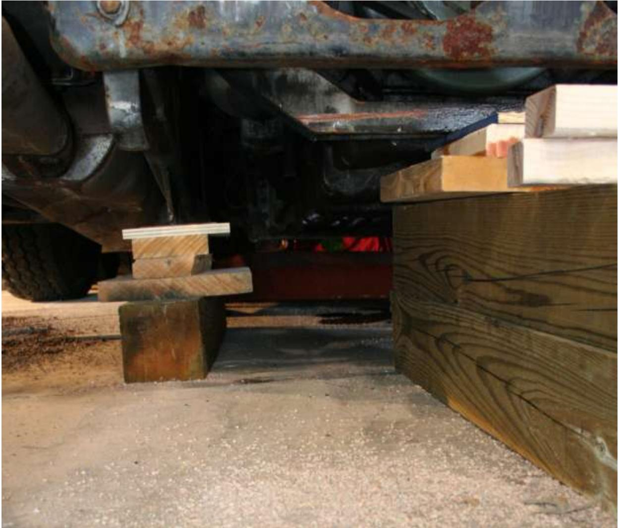
**Figure 2 A photograph of the cribbing supporting the motorcoach during testing.**
