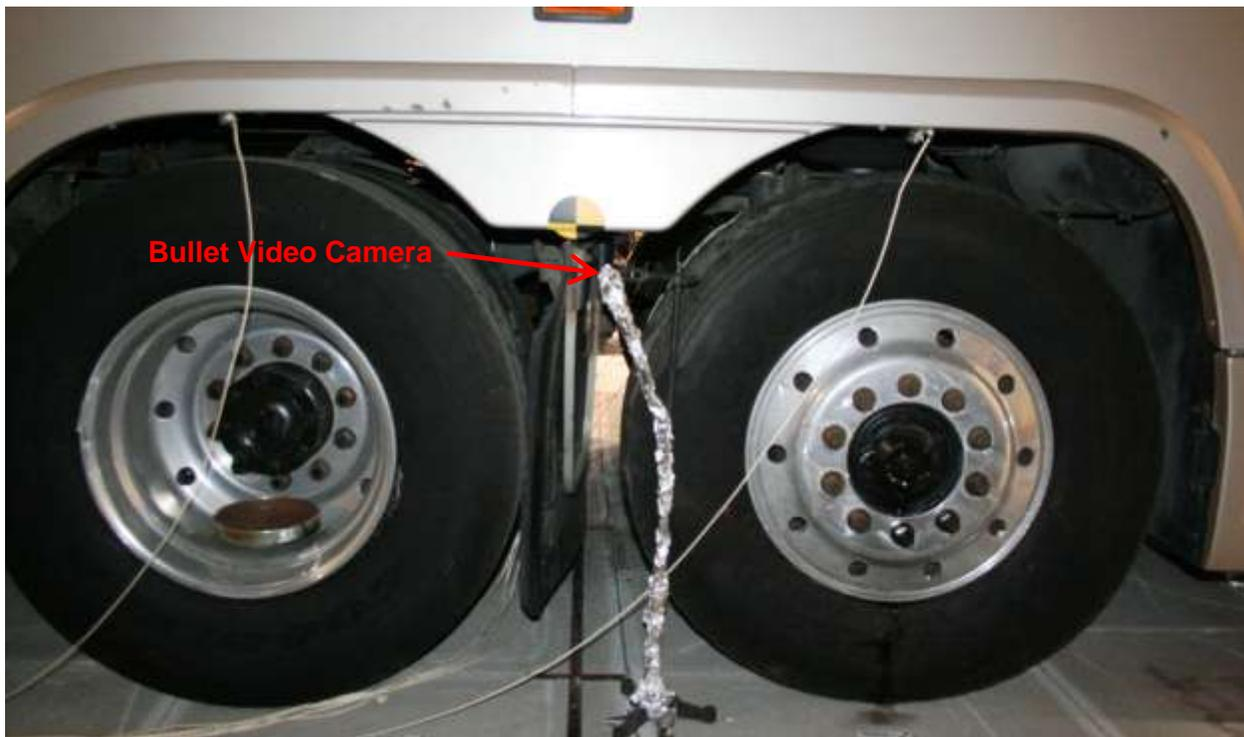
**Figure 30** A photograph of the bullet camera located between the two left (driver's) side axles.
