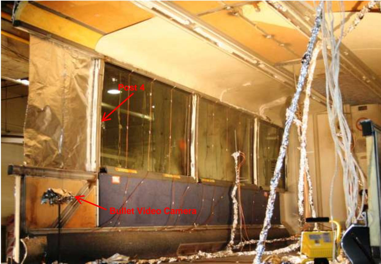
**Figure 31 A photograph showing the location of the passenger compartment bullet camera (lower left) and lighting (lower right) to provide better videos and photographs of the interior.**
