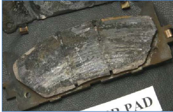
Figure 5: Left-front inboard brake pad; 2009 Lexus ES350 (ODI 10284881)
