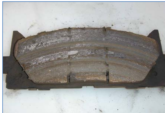
Figure 4: Left-front inboard brake pad; 2007 Lexus ES350 (ODI 10182245)
