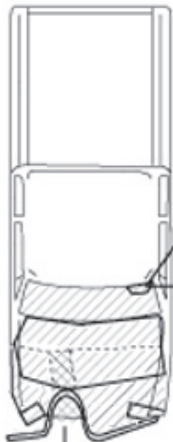
Tree branch damage 5 Max crush Impact #2
