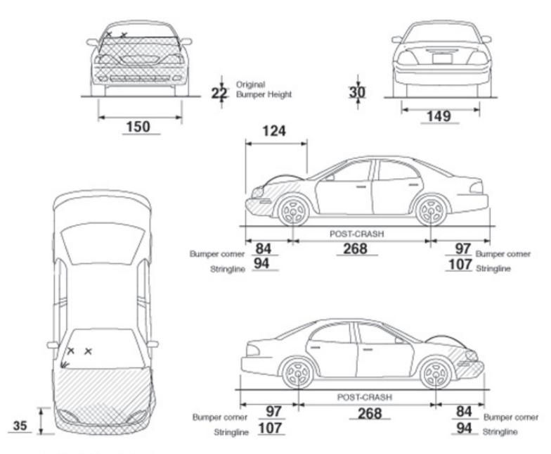
Max. crush to center of front bumper MEASUREMENTS IN CENTIMETERS
