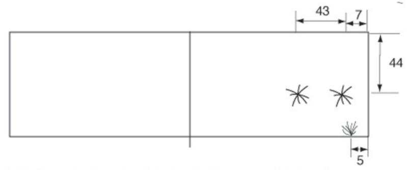
Windshield cracked on the right by dash-mounted airbag flap contact, and cracked on lower right by the rear edge of the hood
