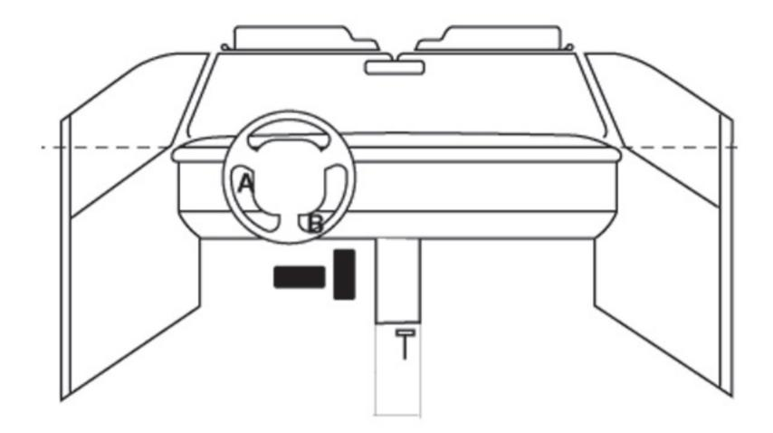
A = turn signal lever, broken off B = knee bolster, indented
