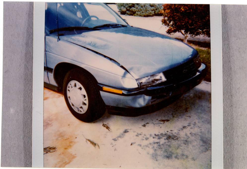
# 01 -- 1992 Florida TRC/IU: 92-04, Task: 0079 Corsica front-right damage
