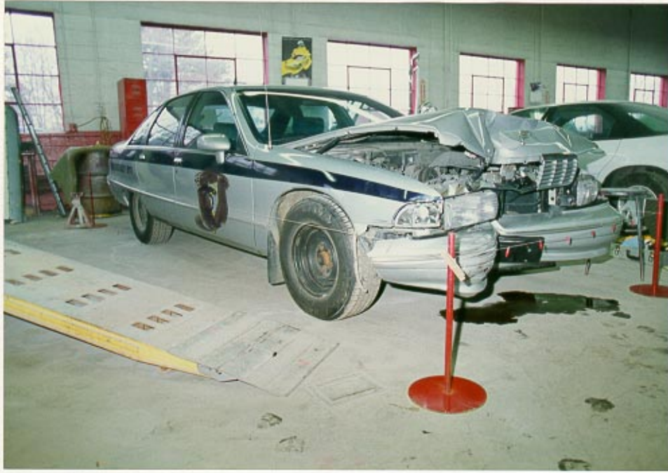
Right front three-quarter view and initial impact damage to the right front corner area
