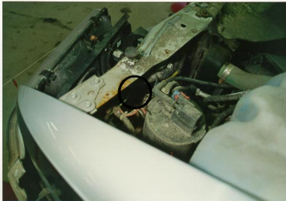
Left front air bag crash sensor mounted to the radiator support panel behind the headlamp assembly
