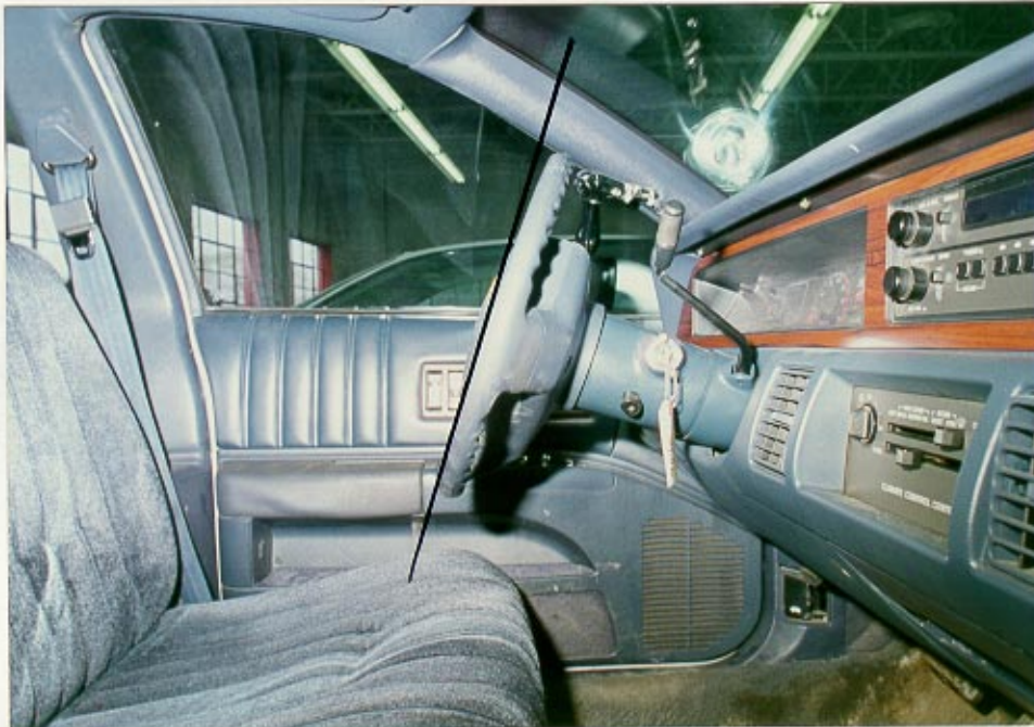
Perpendicular view of the steering wheel rim, 6.4mm (0.25") of upper rim displacement
