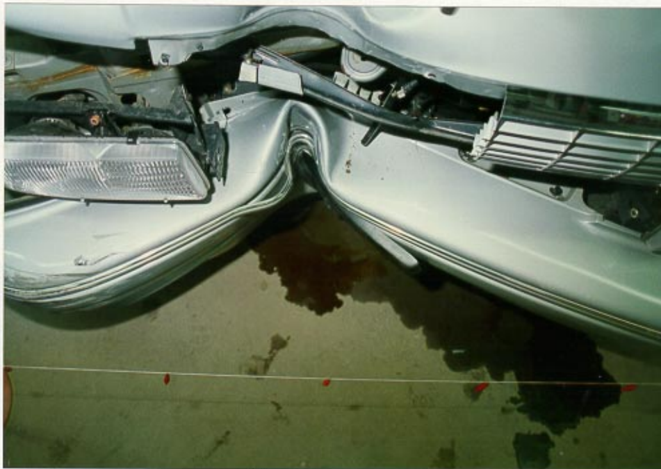
Pedestrian signal pole damage to the Caprice
