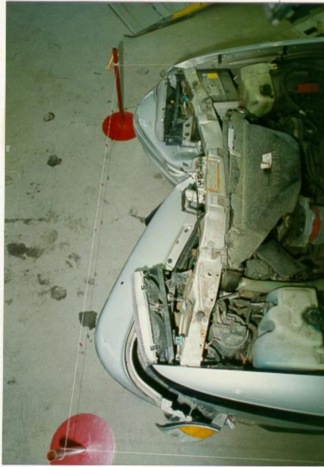
Overhead view of the pole impact damage to the bumper and radiator support panel
