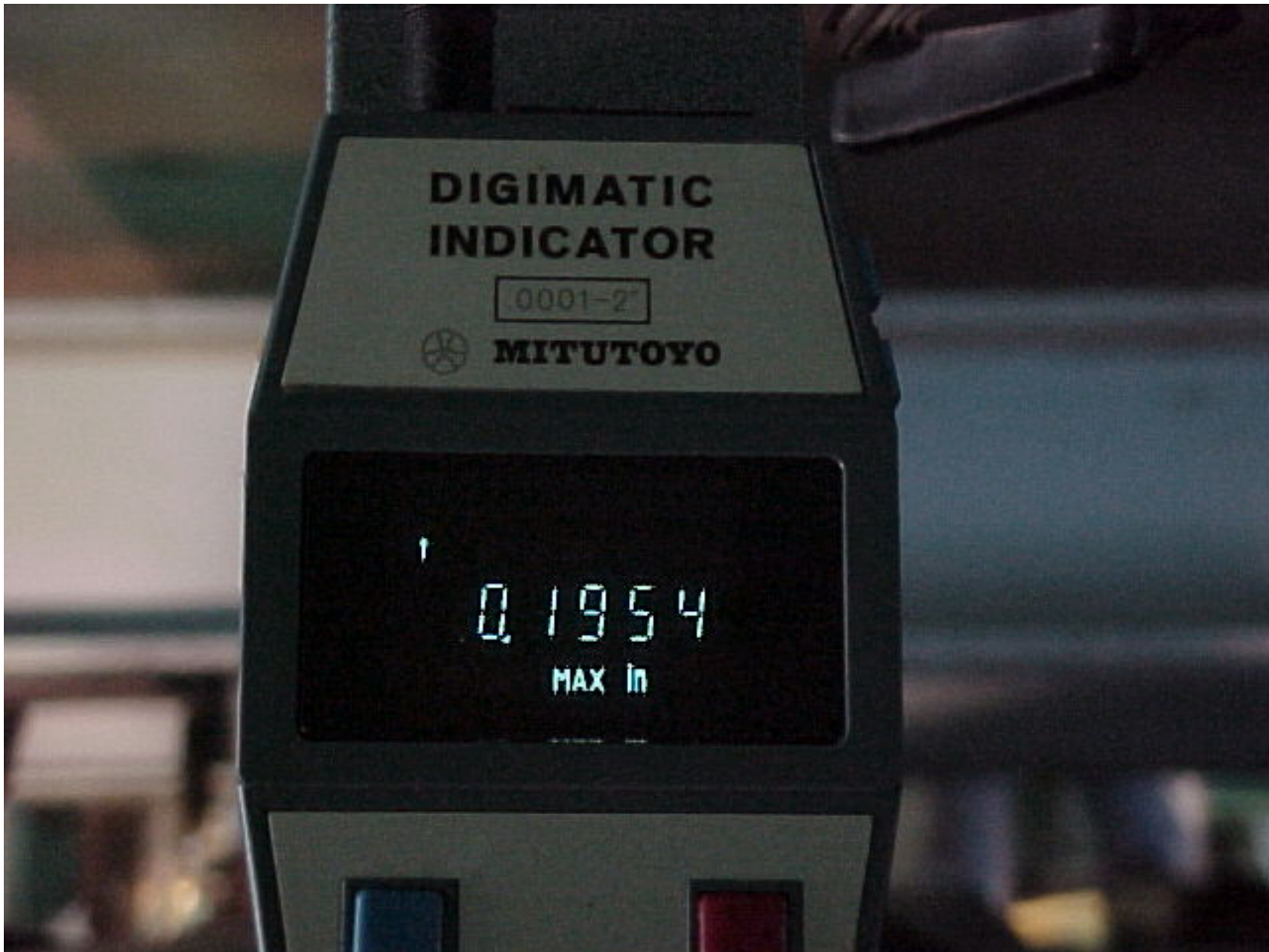
FIGURE 5.22 LEFT FRONT DISPLACEMENT AT FULL LOAD (INCHES)
