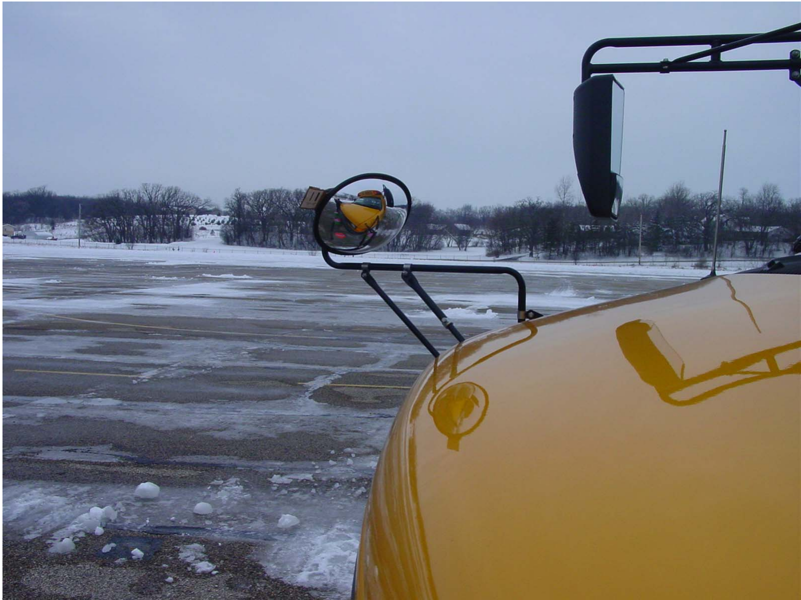
Right Front Cross View Mirror and Mounting
