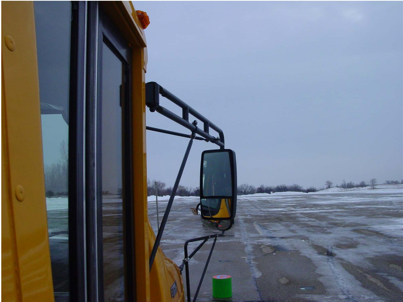
Passenger Side Rearview Mirror and Mounting
