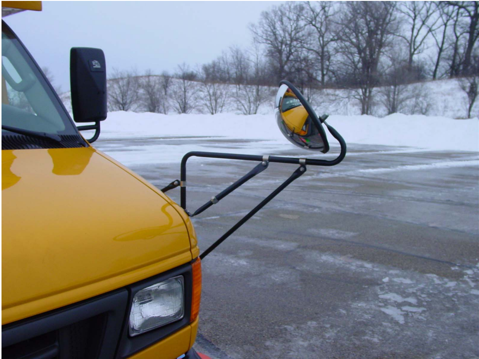
Left Front Cross View Mirror and Mounting
