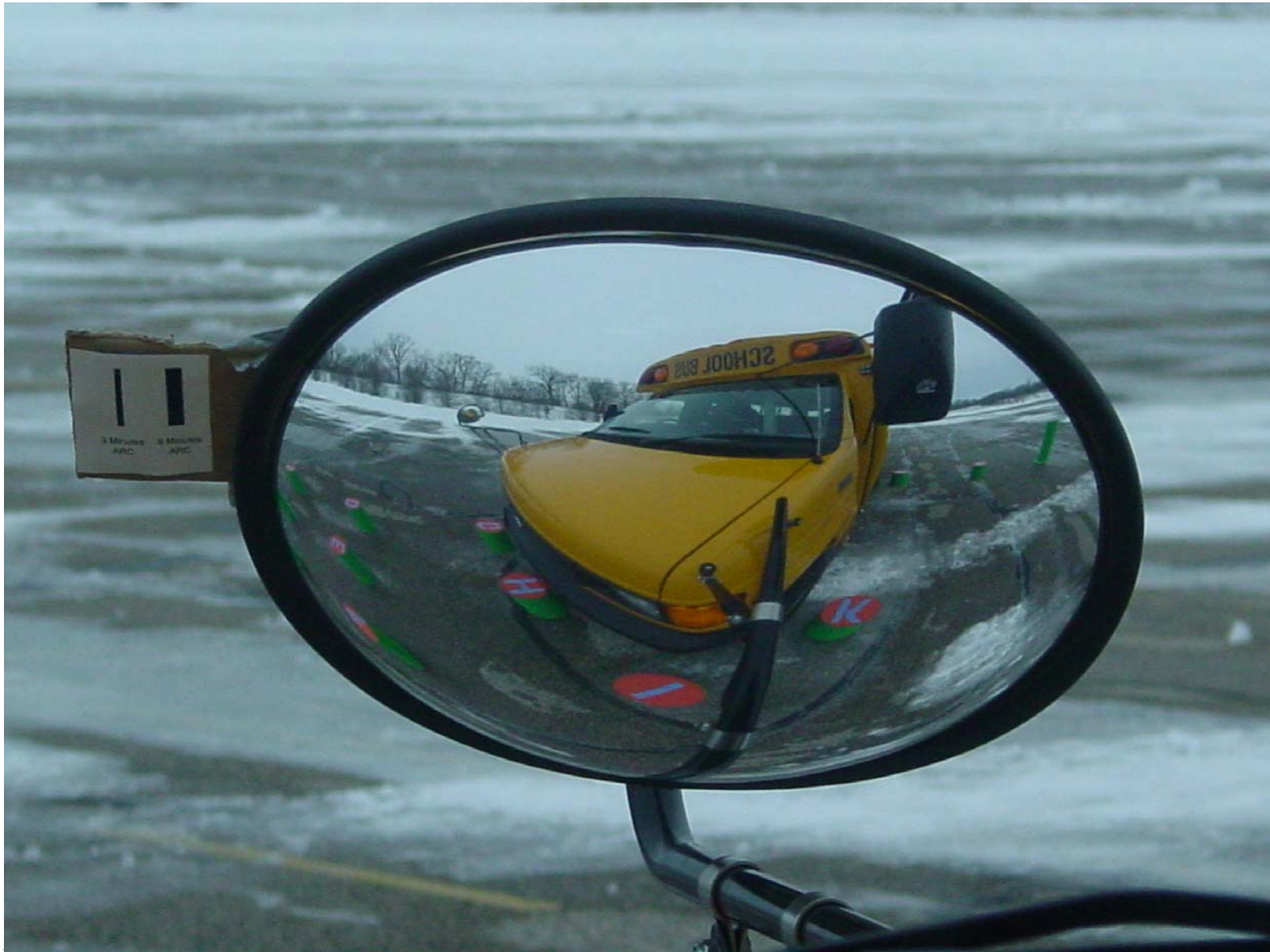
Mirror #2 System B Field of View
