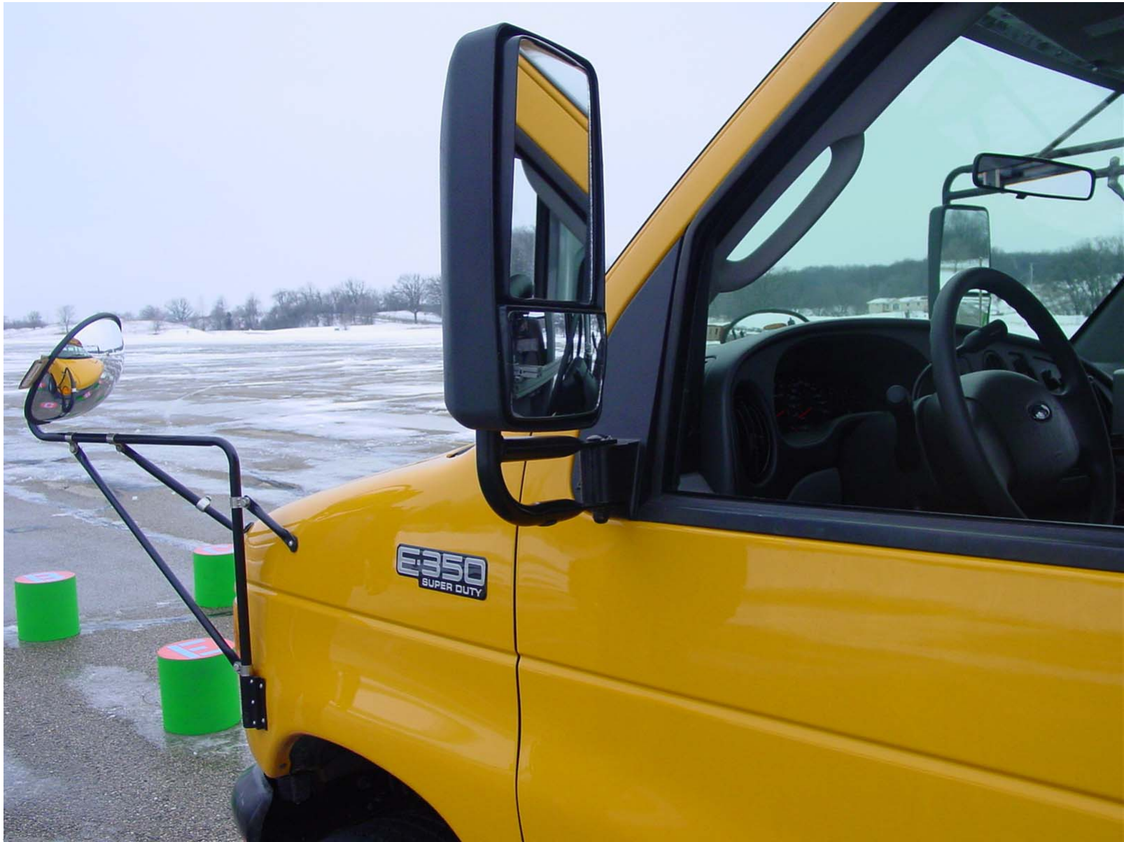
Driver Side Rearview Mirror and Mounting
