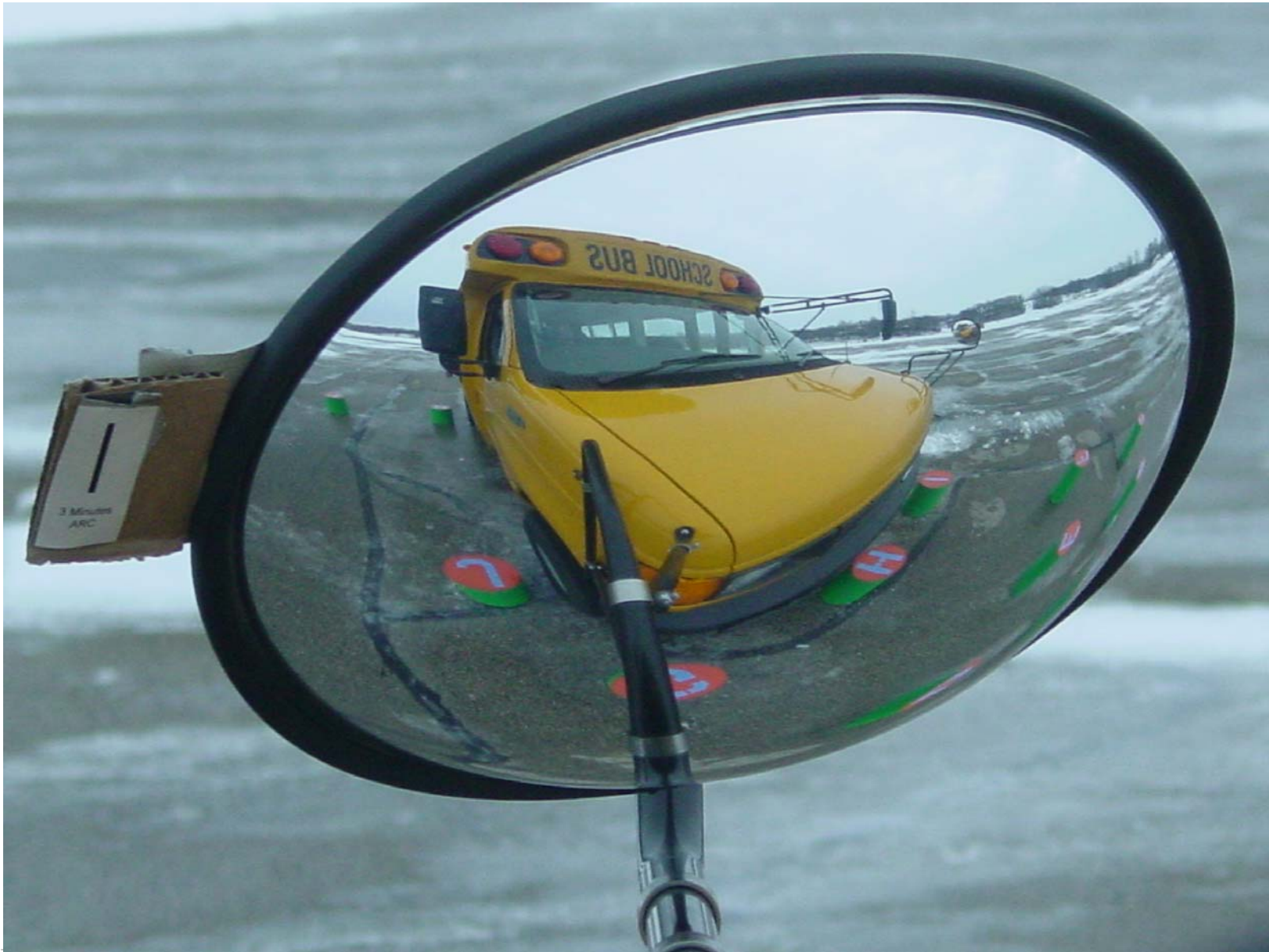
Mirror #1 System B Field of View
