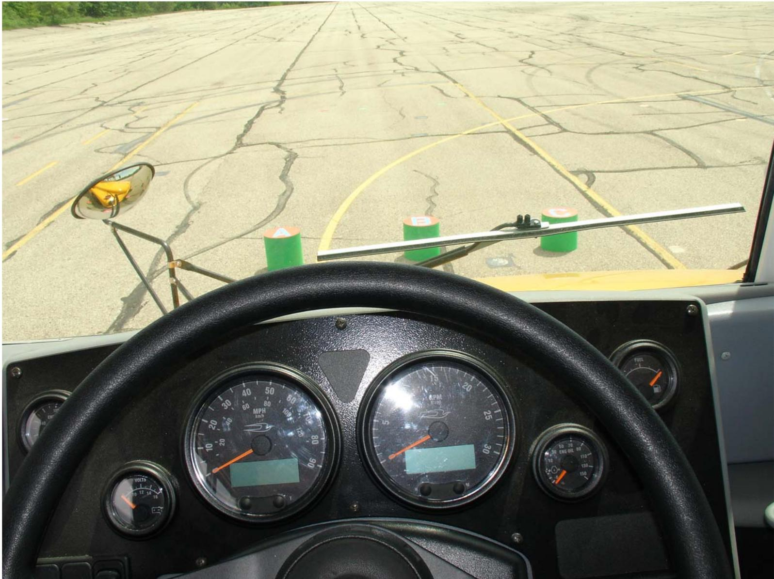
View of Cylinders using no Mirror System
