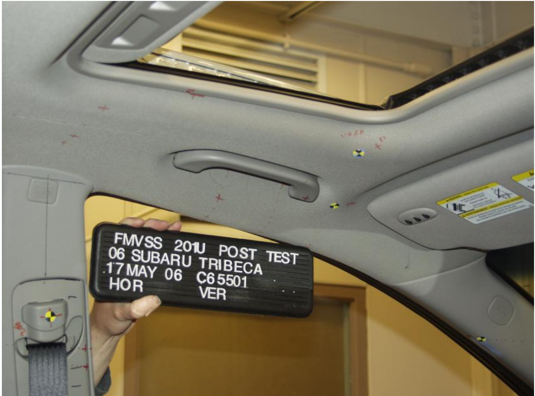
Figure A-21 : POST-TEST DRIVER SIDE SIDE RAIL
