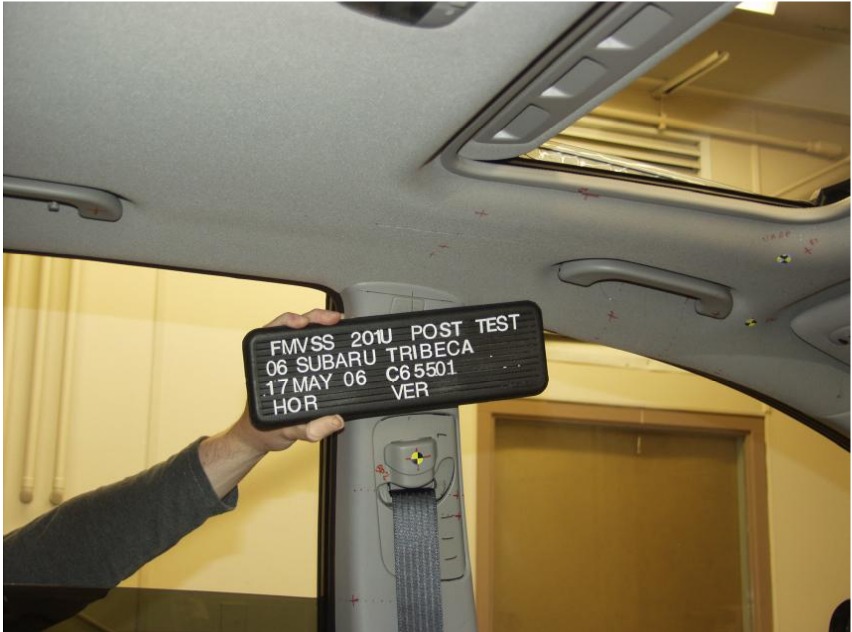
Figure A-22 : POST-TEST DRIVER SIDE B-PILLAR
