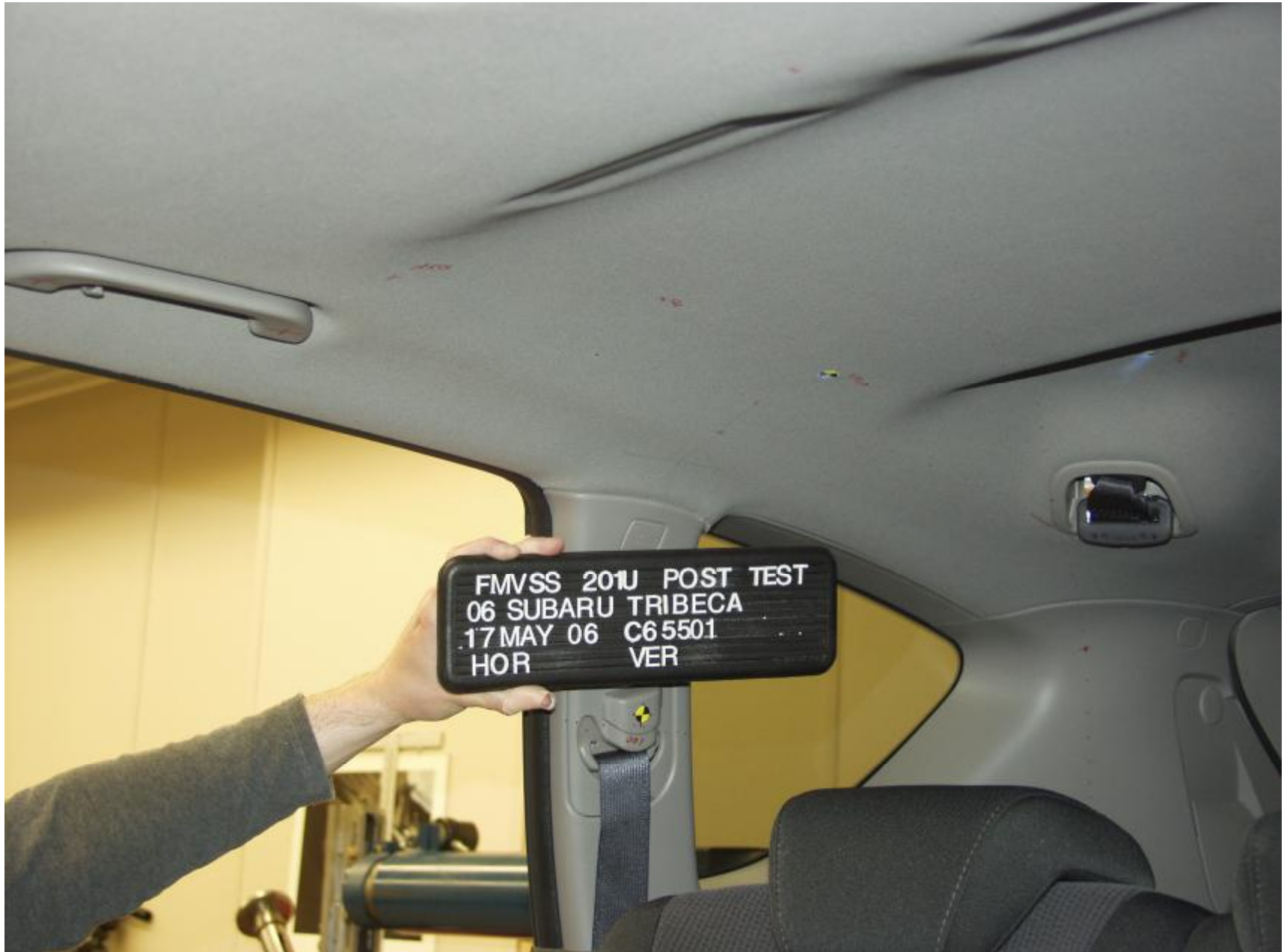
Figure A-30 : POST-TEST PASSENGER SIDE OTHER PILLAR
