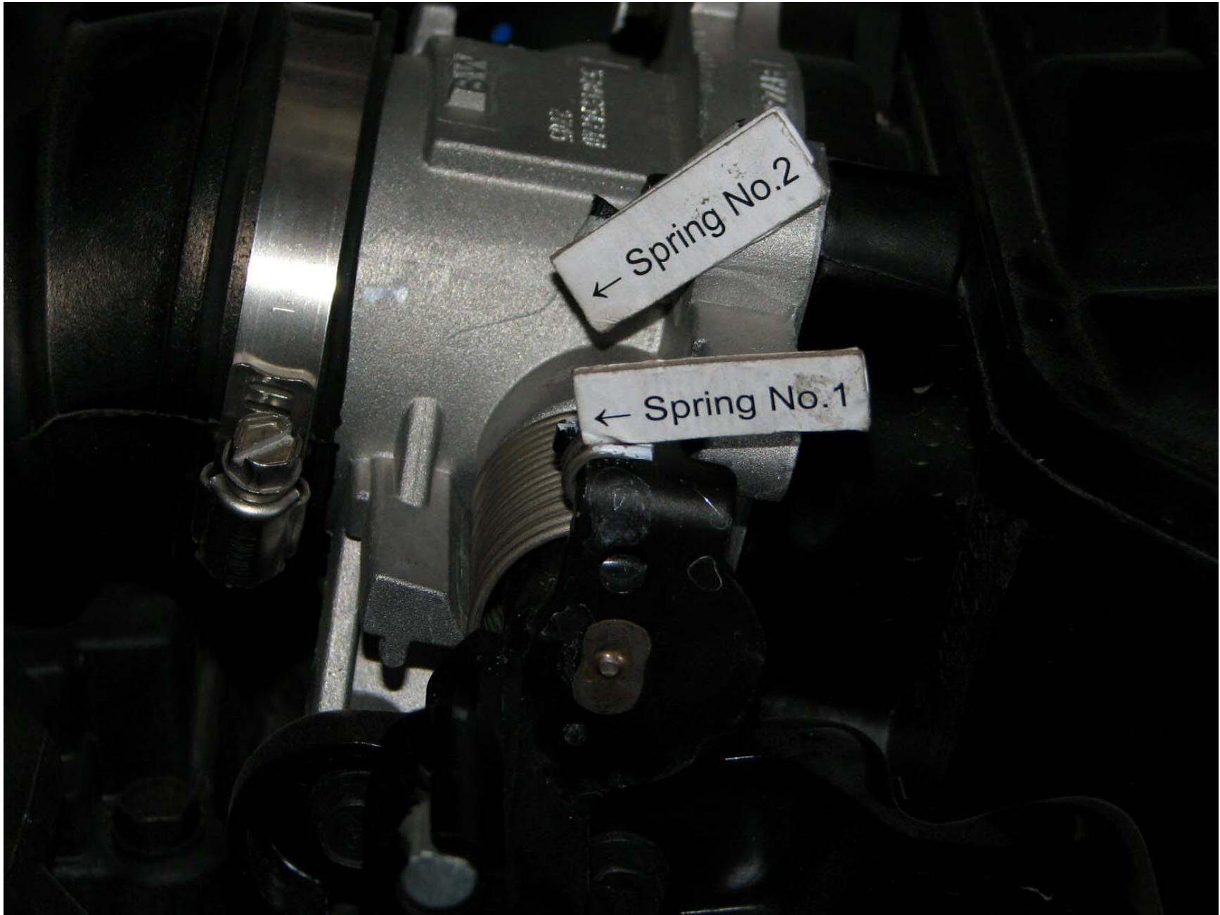
2006 JEEP WRANGLER Figure A-7: Spring 1 and 2 Located on Vehicle's Accelerator Control System (Throttle Body) NHTSA NO. C60303 FMVSS NO. 124
