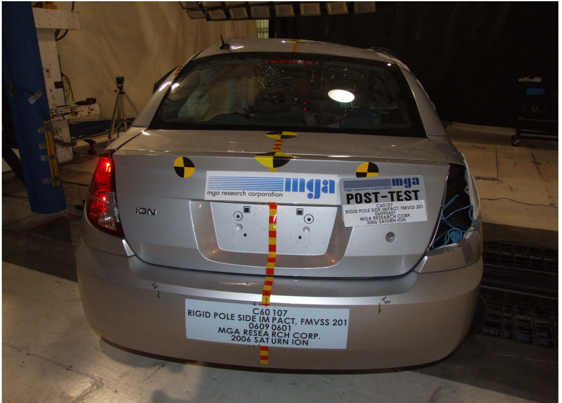
Post-Test Rear View of Test Vehicle
