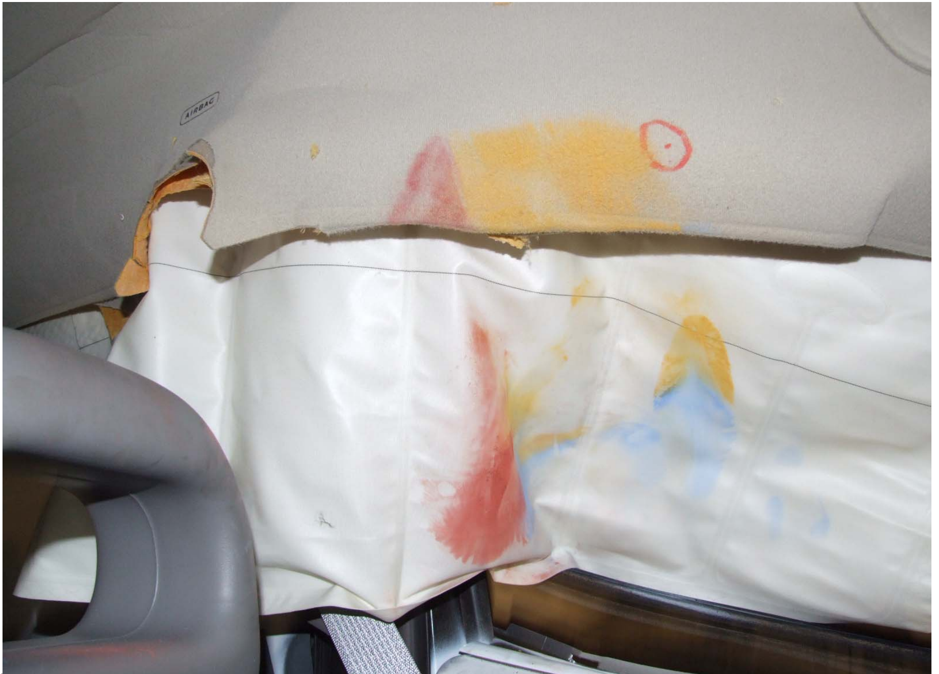
Post-Test Driver Dummy Head Contact
