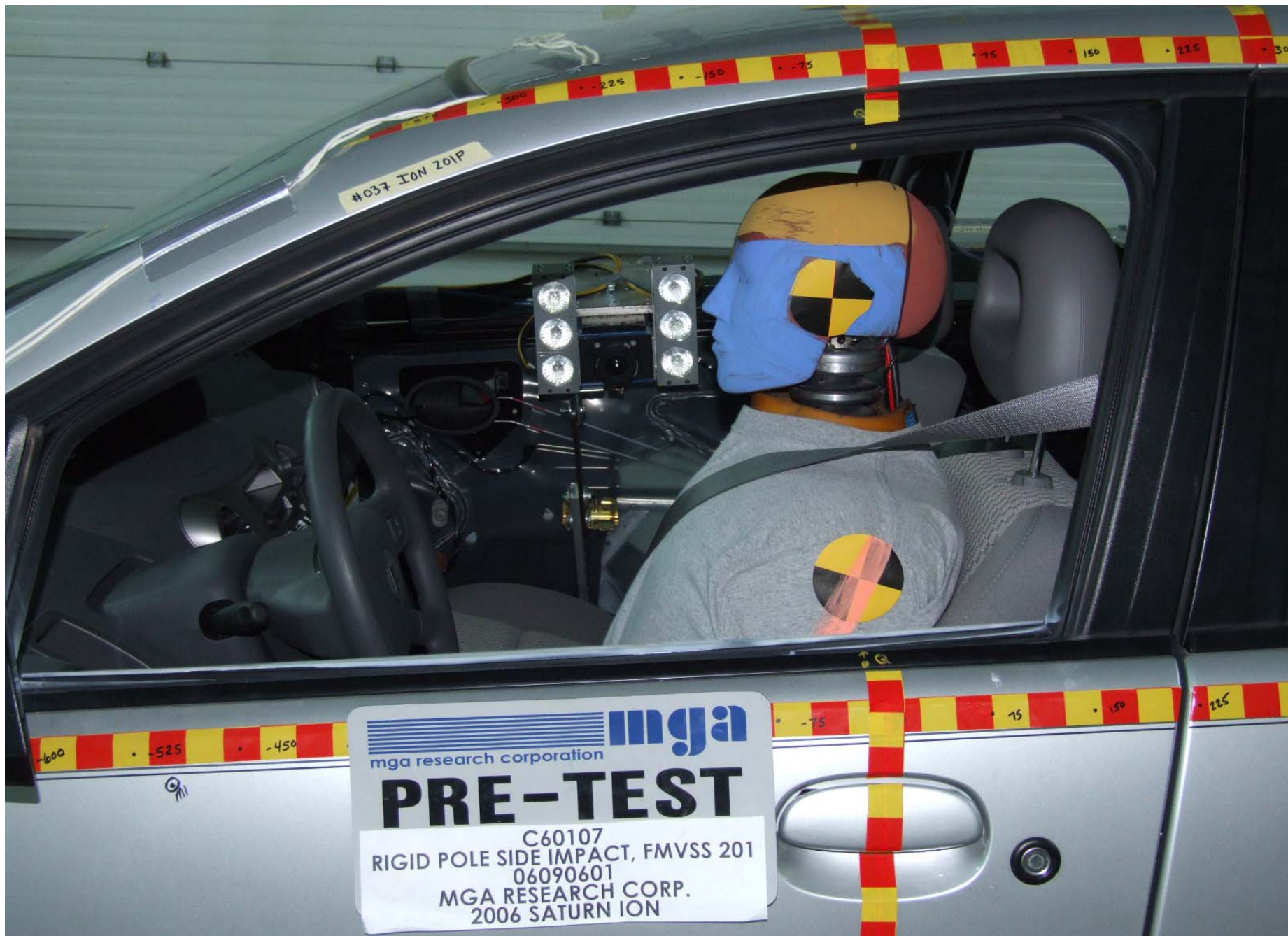
Pre-Test Driver Dummy Left Side View
