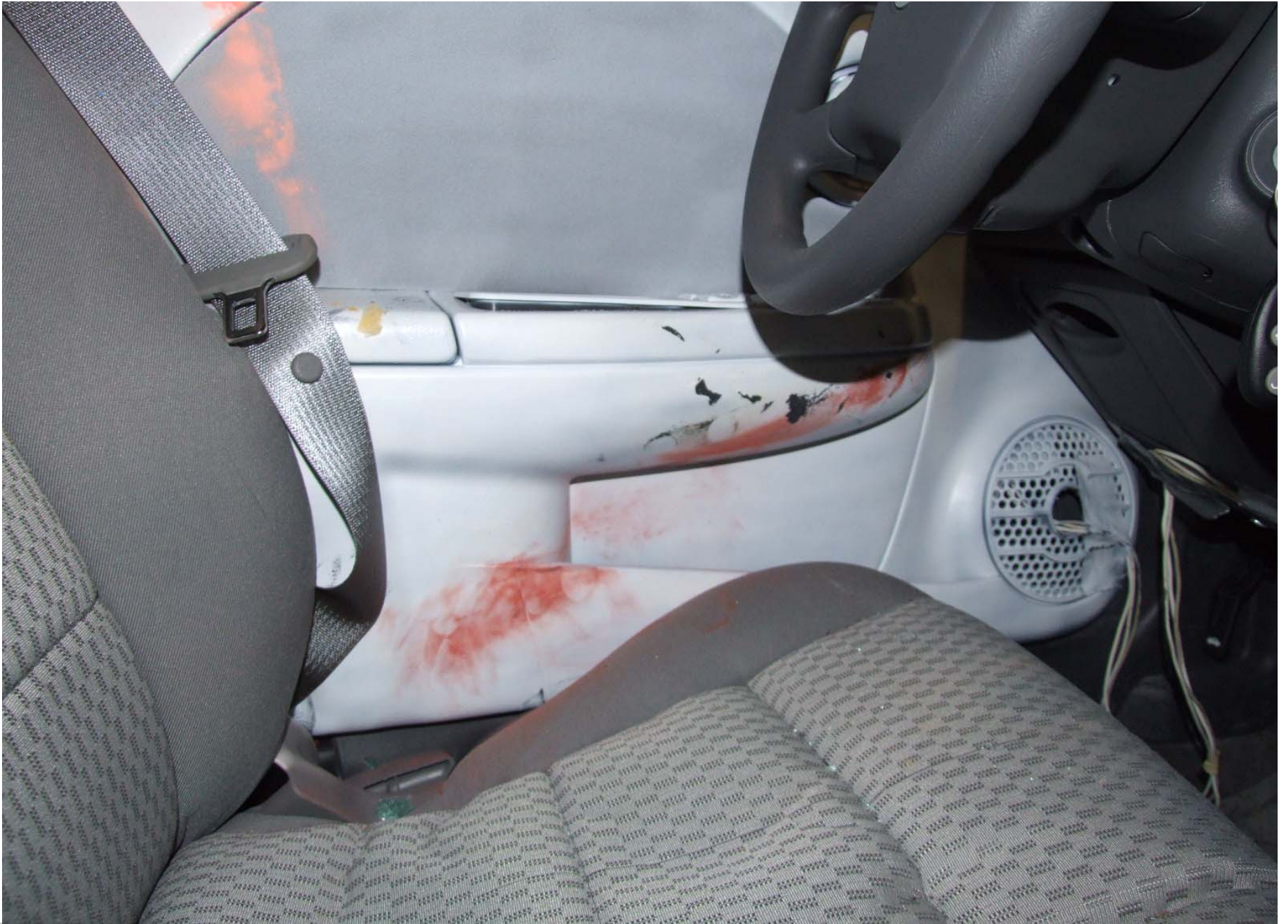
Post-Test Driver Dummy Thorax Contact
