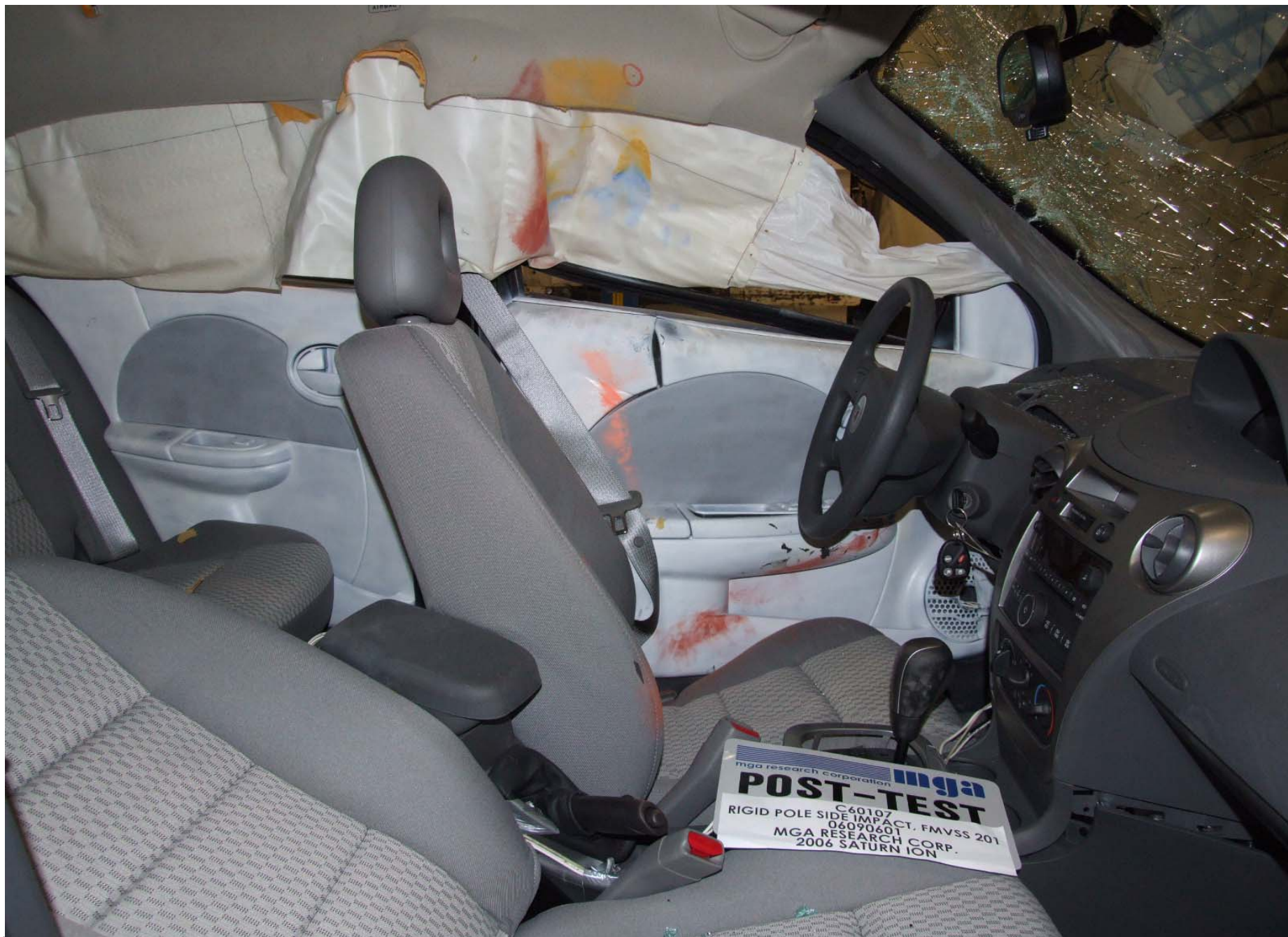
Post-Test Driver Dummy Contact
