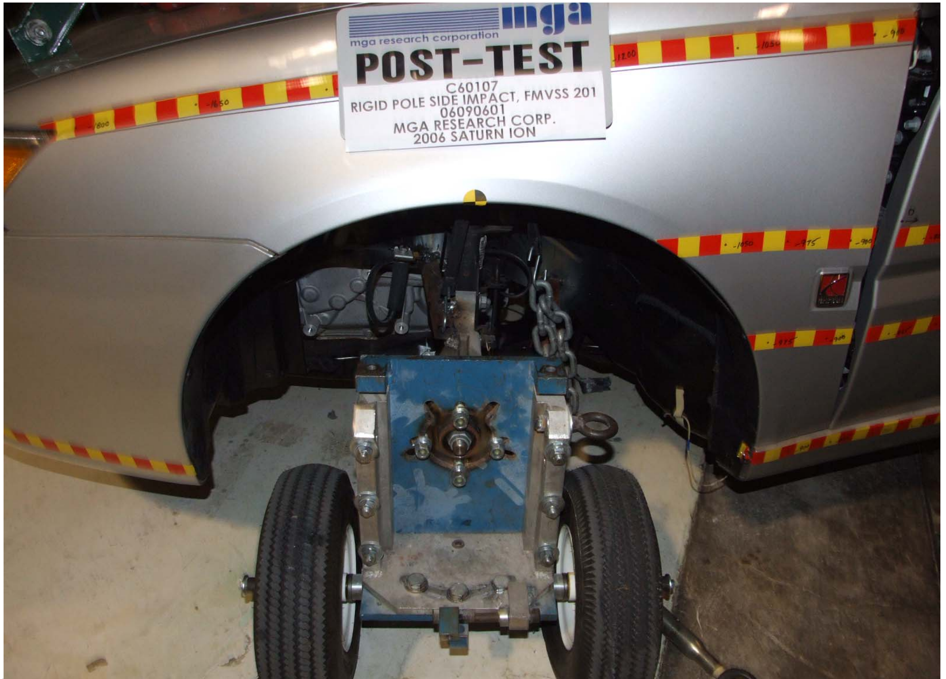
Post-Test Left Front Wheel Dolly
