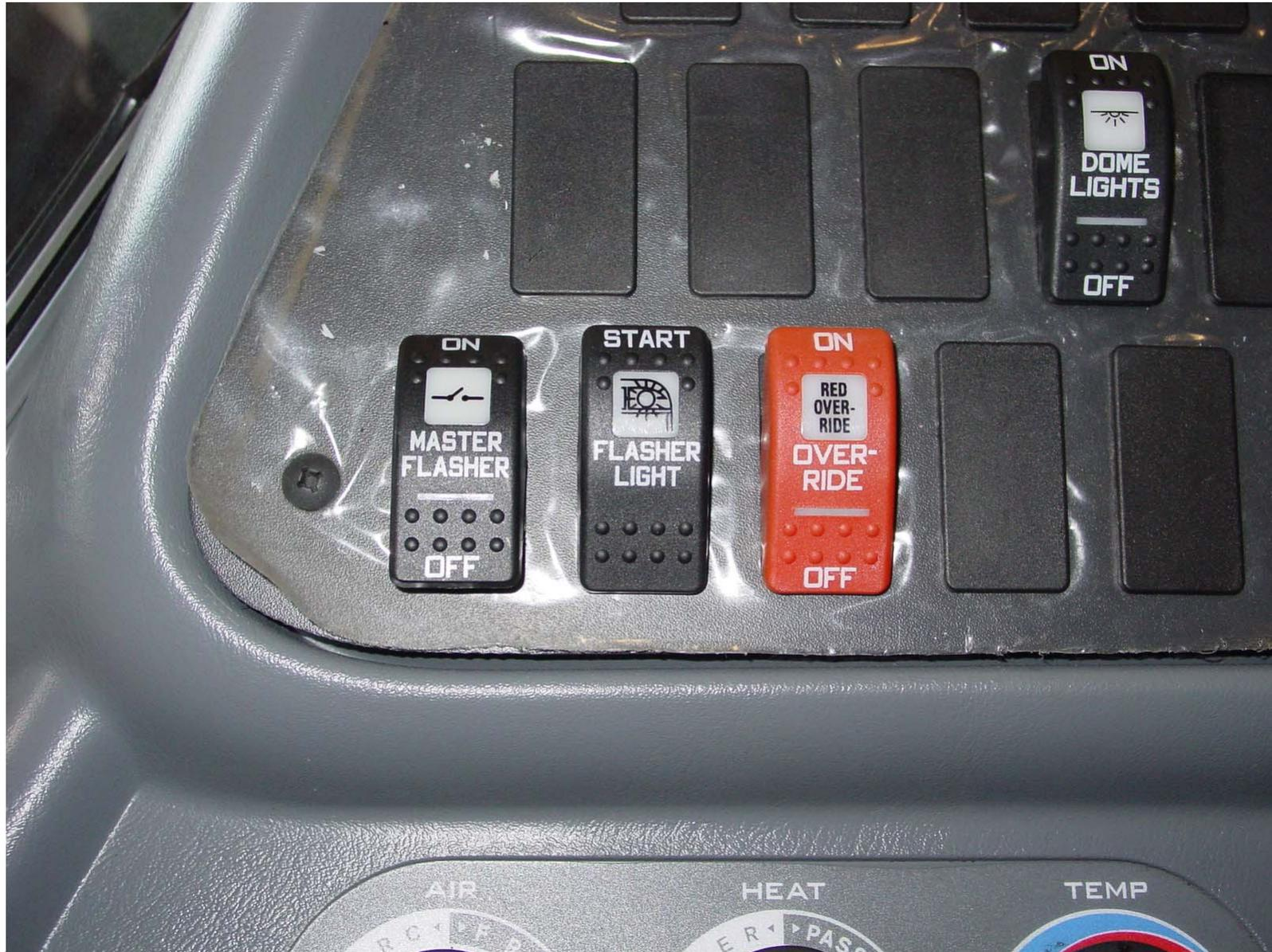
Photo 5 - Close Up View of the Switches That Allow Extension of the Stop Signal Arm(s)
