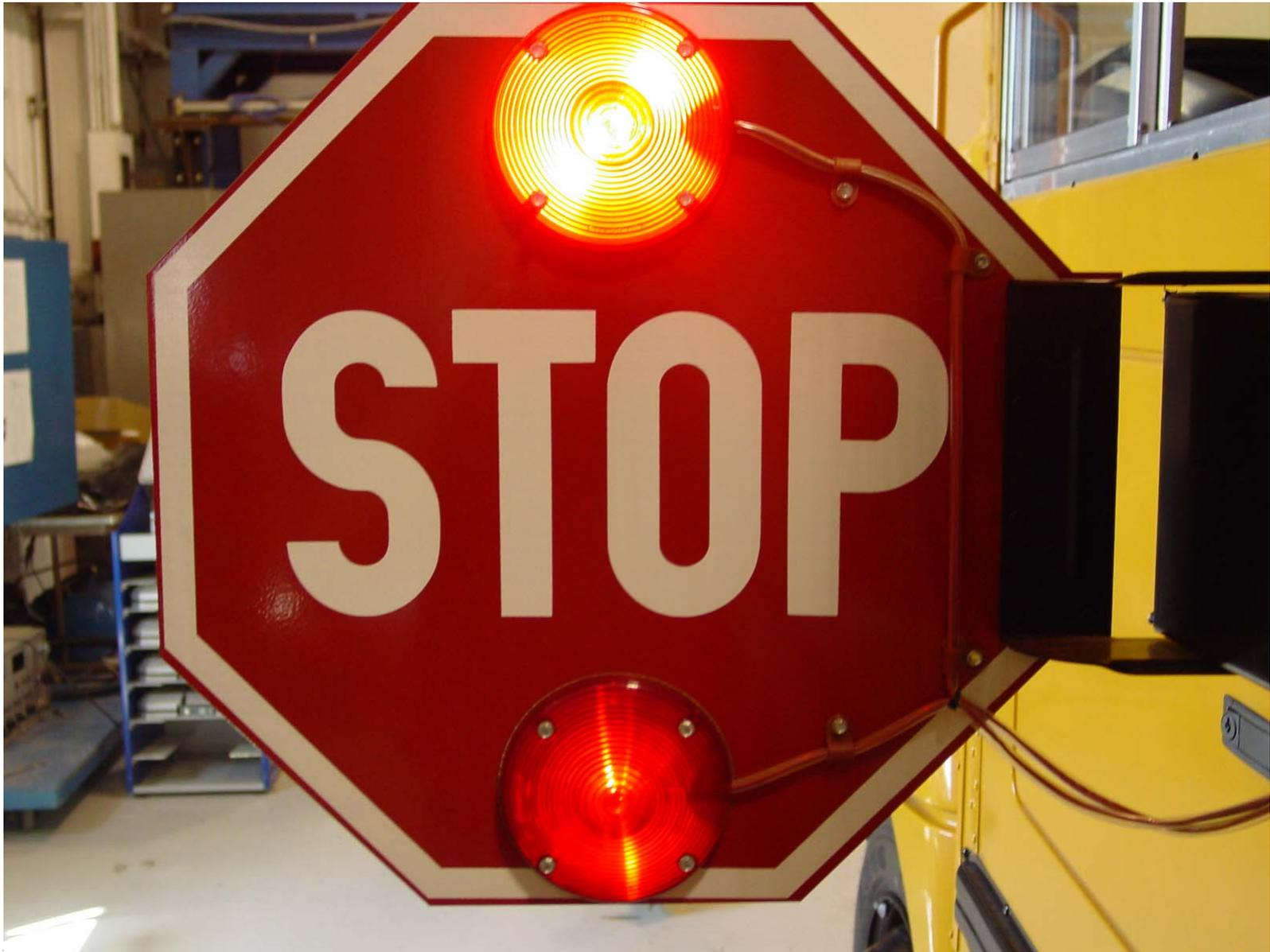
Photo 4 - Back Close Up View of Stop Signal Arm
