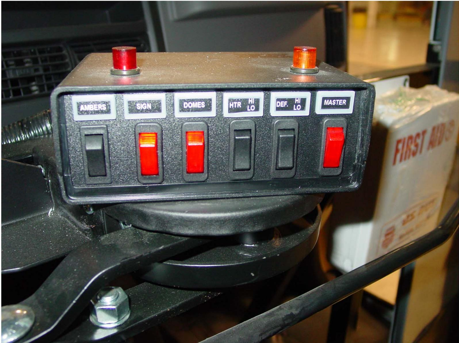
Photo 6 - Close Up View of the Switches That Allow Extension of the Stop Signal Arm(s)
