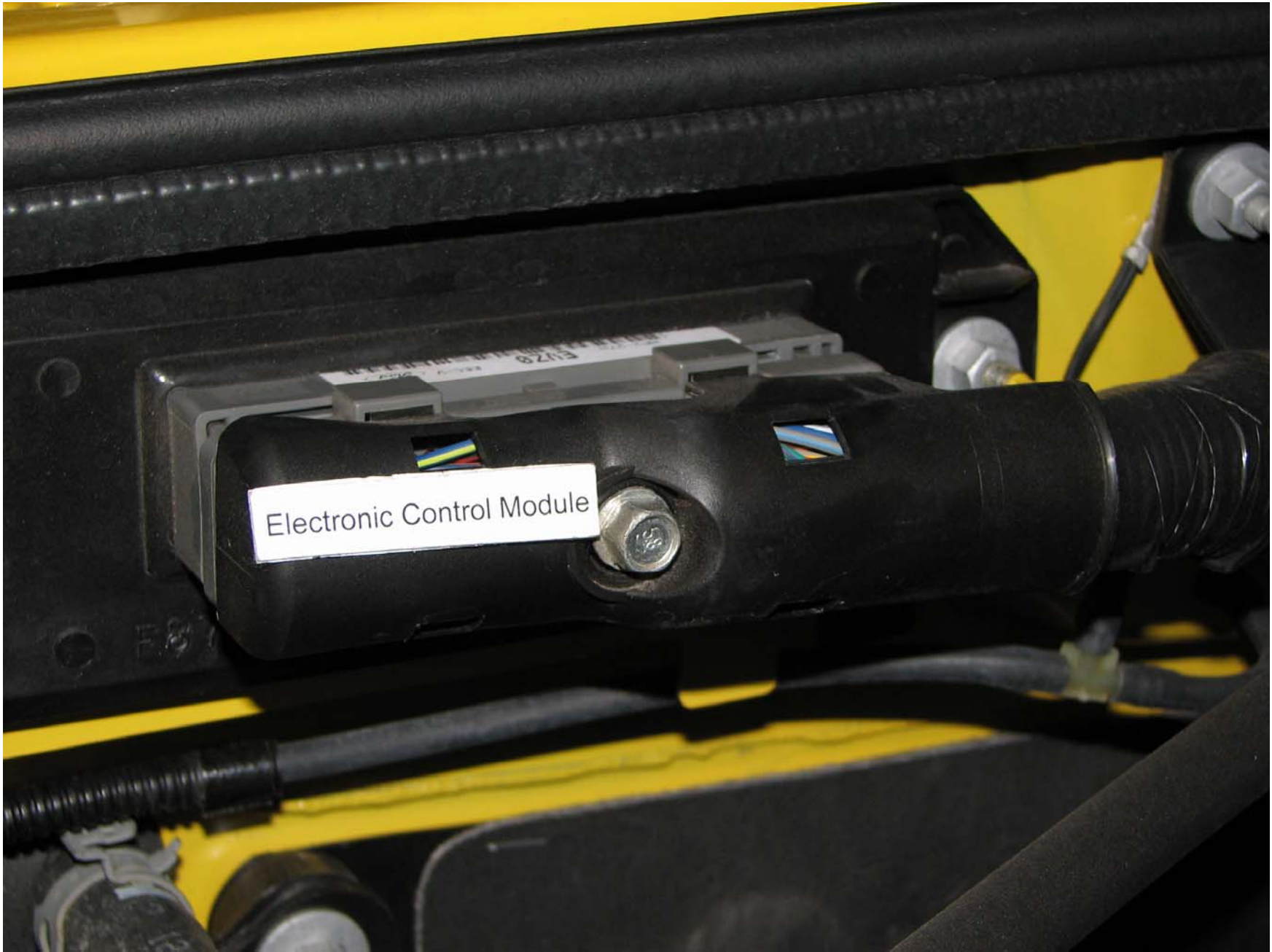
Figure A-10: Electronic Control Module
