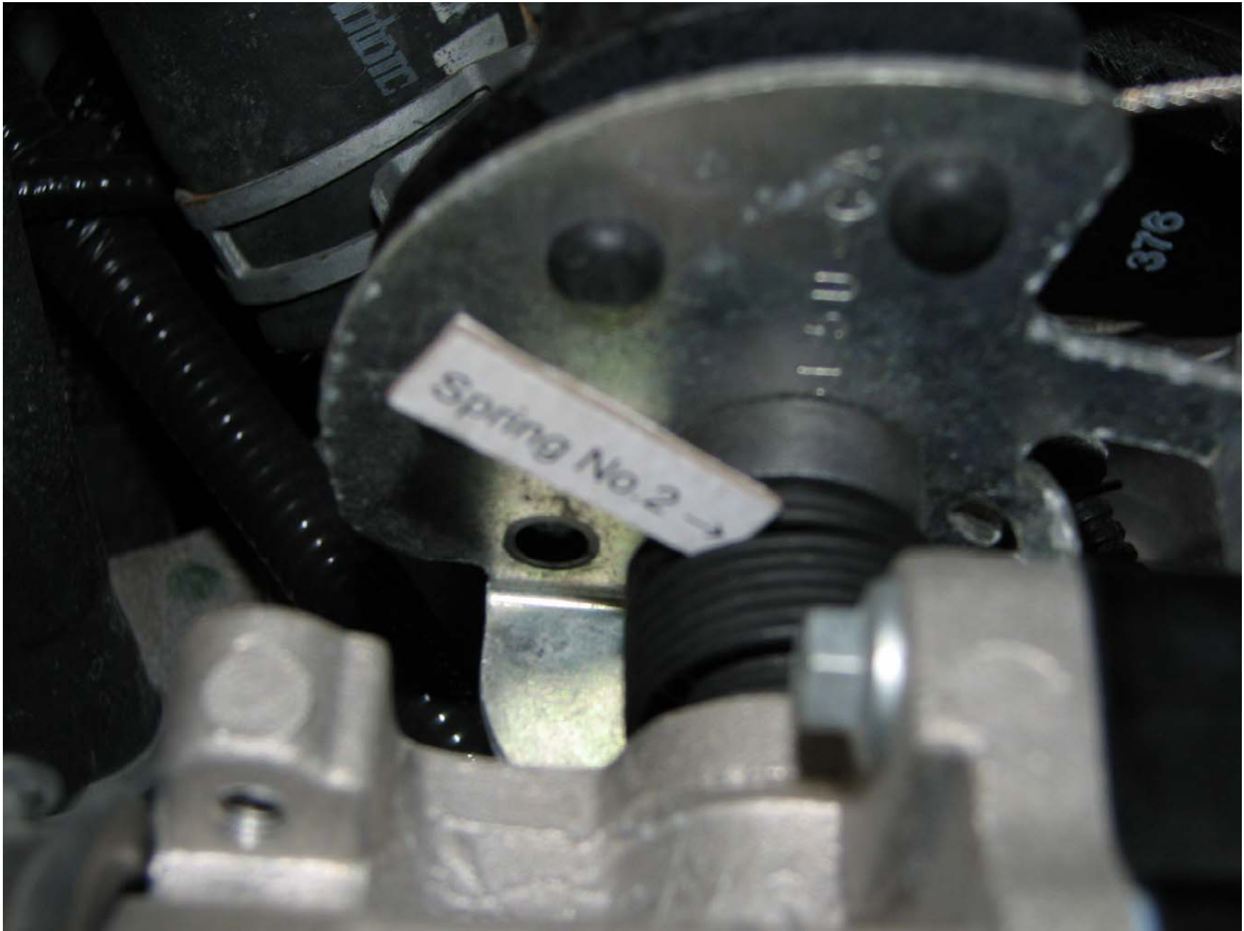
Figure A-8: Spring 2 Located on Vehicle's Accelerator Control System (Throttle Body)
