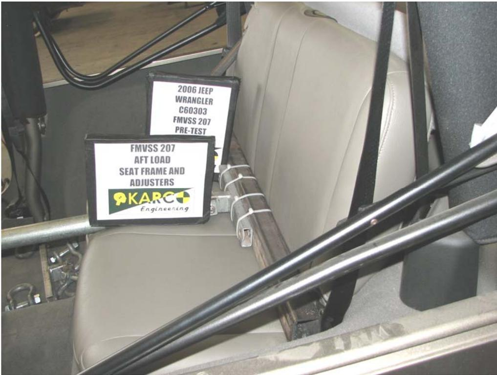
FIGURE 39. Aft Load on Seat Frame and Adjusters, P4, Pre-Test
