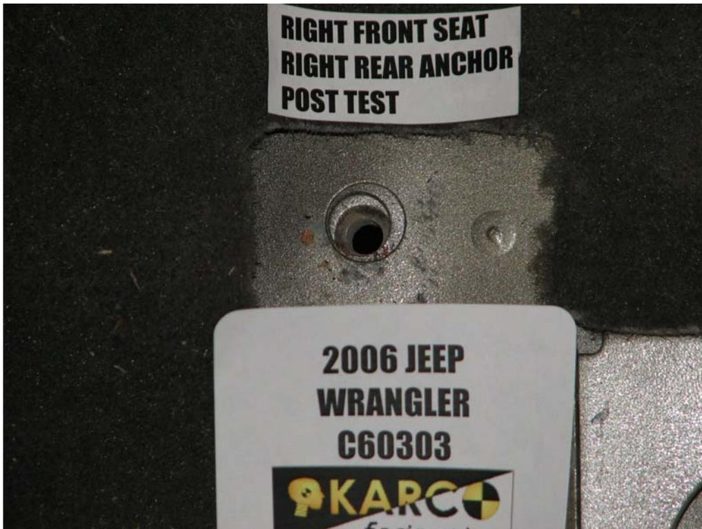
FIGURE 88. Floor Pan Anchor, P2, Post-Test
