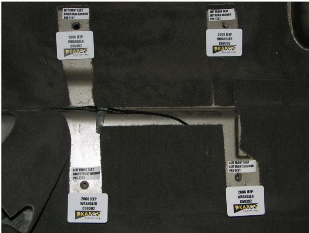
FIGURE 43. Floor Pan Anchors, P1 Overall, Pre-Test
