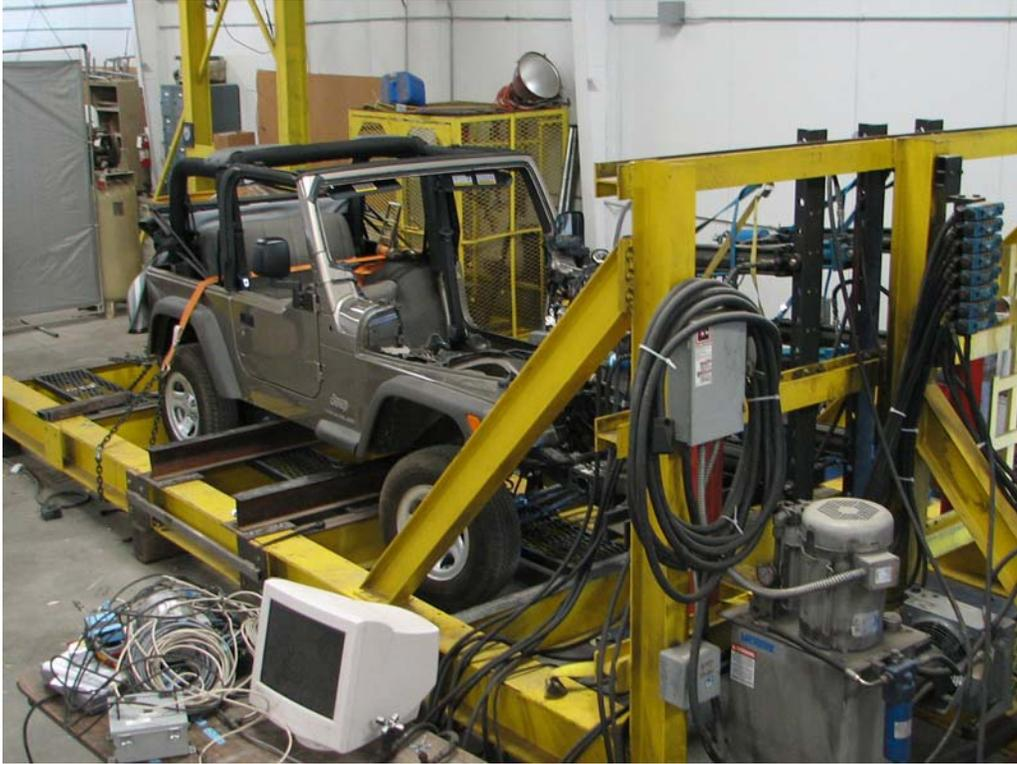
FIGURE 7. Vehicle Mounted in Test Fixture
