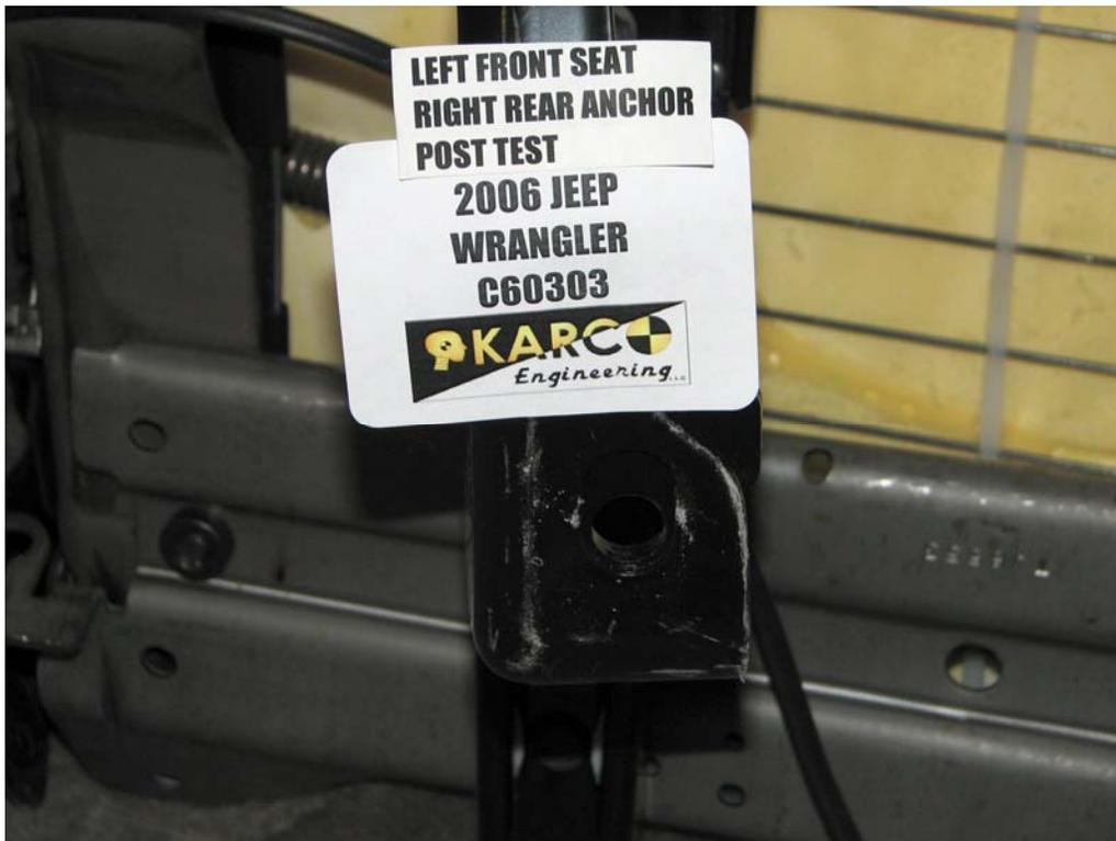
FIGURE 62. Seat Anchor, P1, Post-Test
