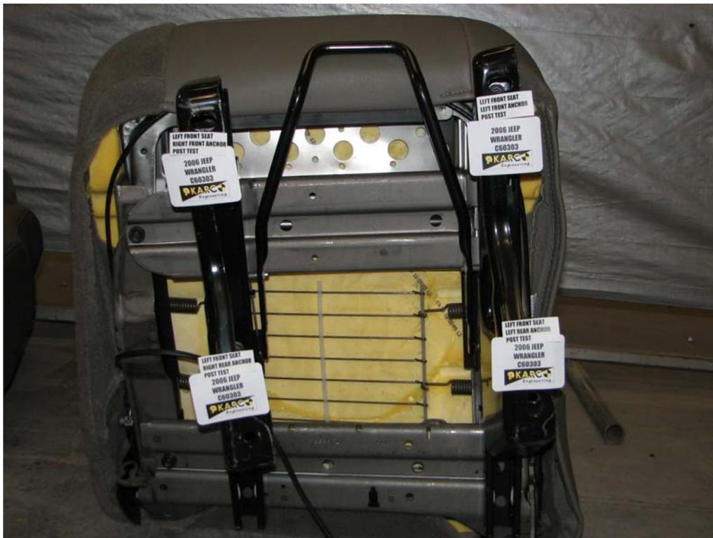
FIGURE 46. Seat Anchors, P1 Overall, Post-Test
