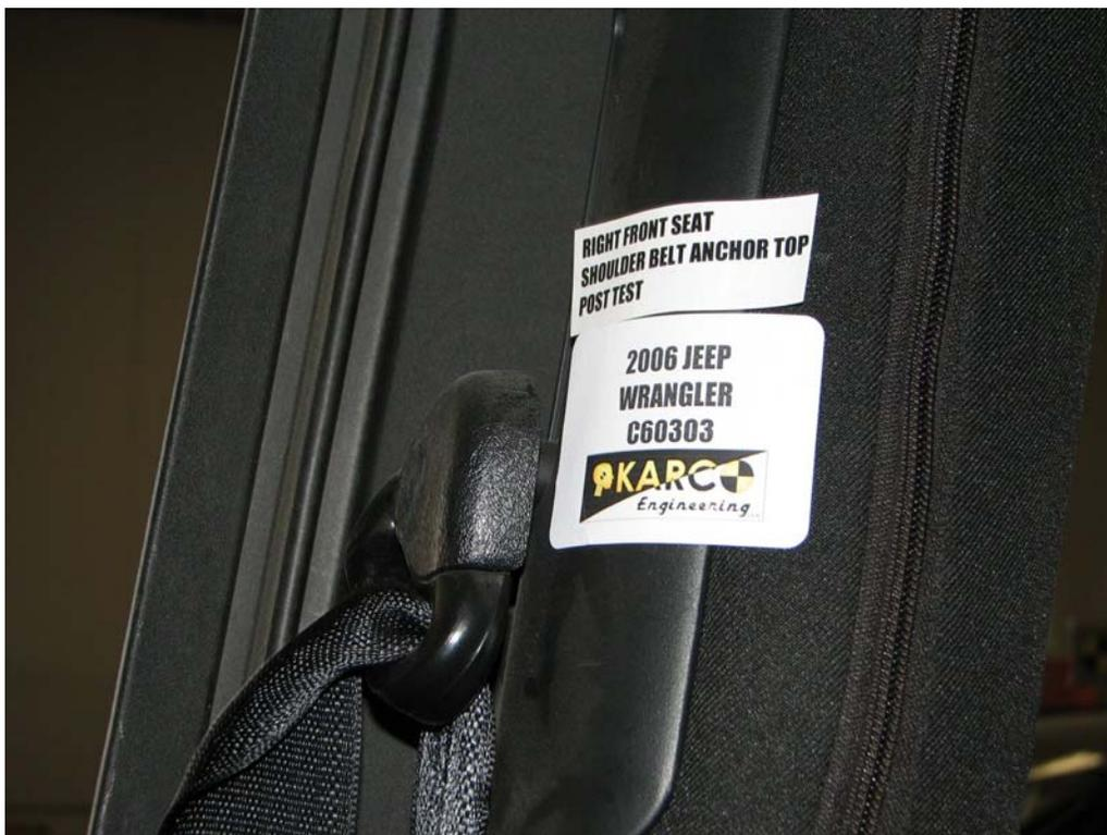
FIGURE 92. Shoulder Belt Anchor, P2, Post-Test
