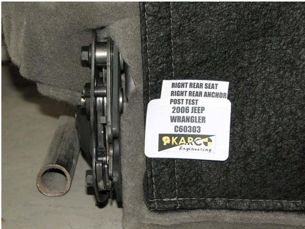
FIGURE 118. Seat Anchor, P3 and P4, Post-Test
