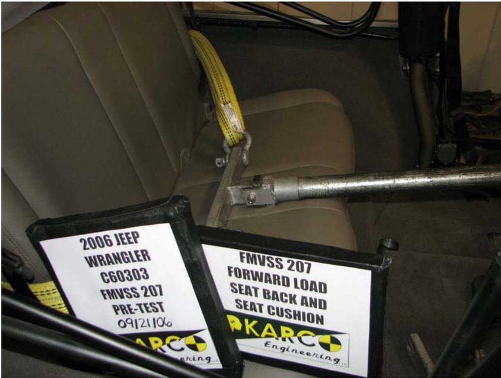
FIGURE 29. Forward Load on Seat Back, P3, Pre-Test
