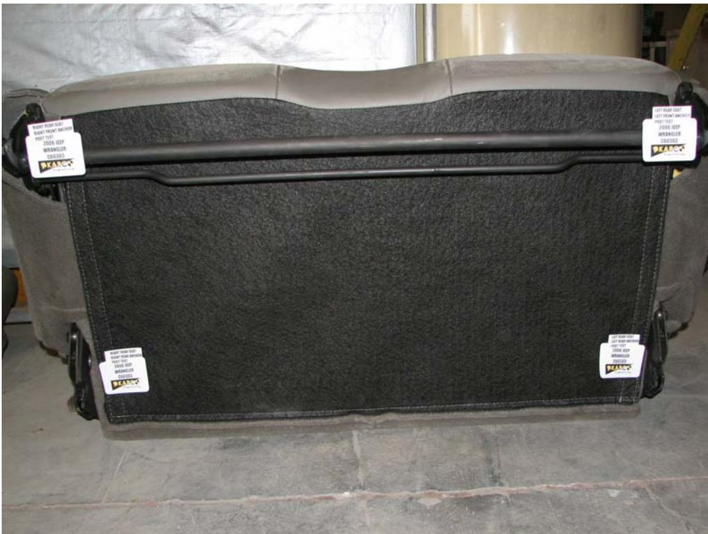
FIGURE 102. Seat Anchors, P3 and P4 Overall, Post-Test
