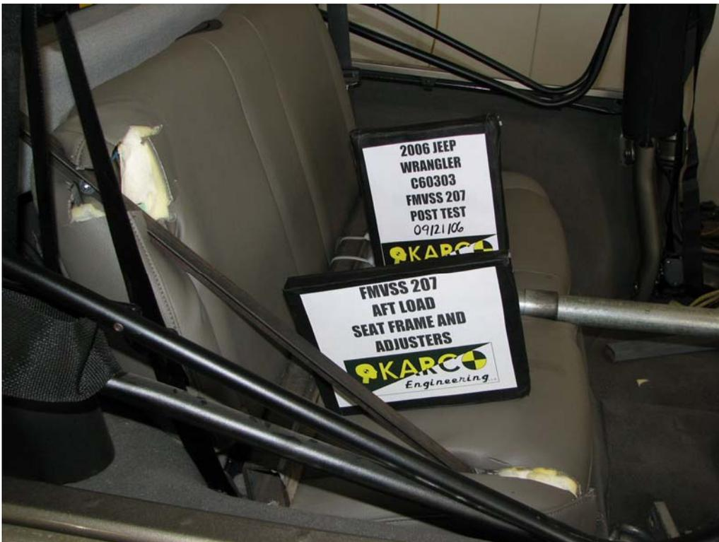
FIGURE 42. Aft Load on Seat Frame and Adjusters, P3, Post-Test
