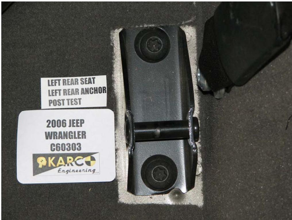
FIGURE 112. Floor Pan Anchor, P3 and P4, Post-Test
