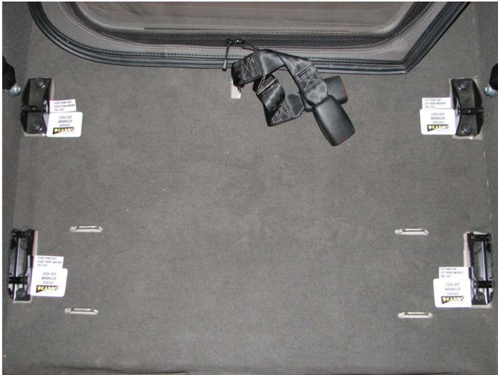
FIGURE 99. Floor Pan Anchors, P3 and P4 Overall, Pre-Test
