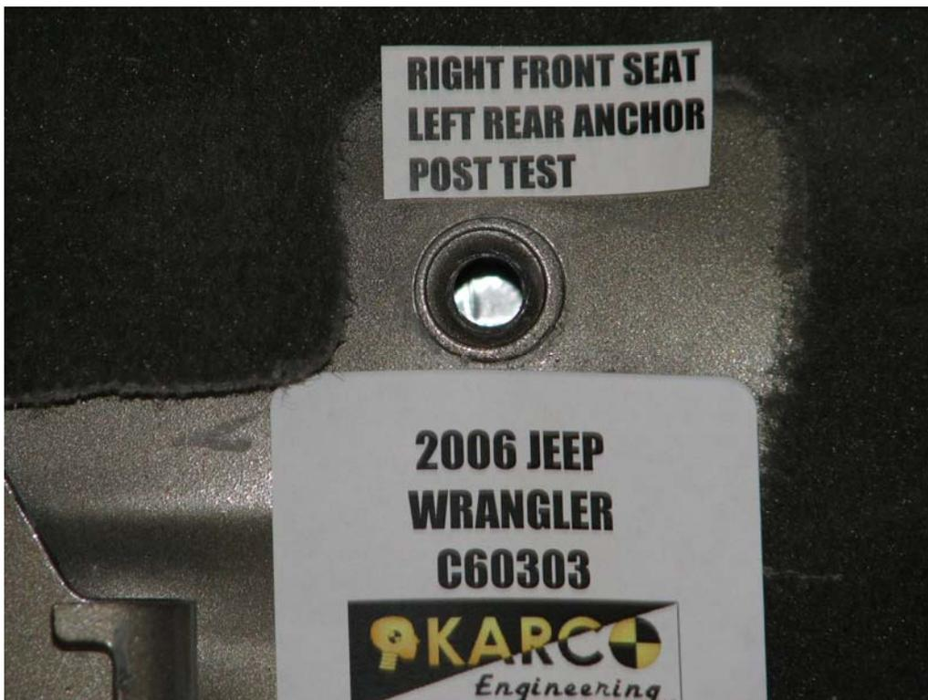
FIGURE 84. Floor Pan Anchor, P2, Post-Test
