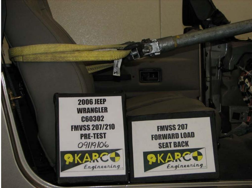
FIGURE 17. Forward Load on Seat Back, P2, Pre-Test
