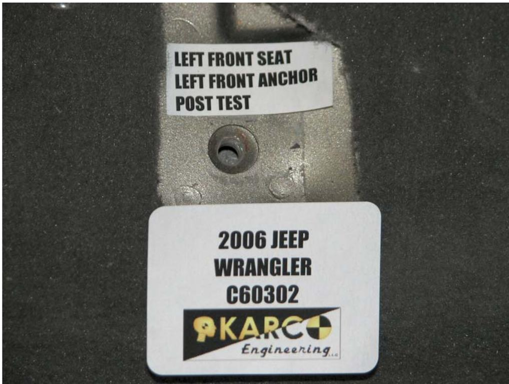
FIGURE 48. Floor Pan Anchor, P1, Post-Test
