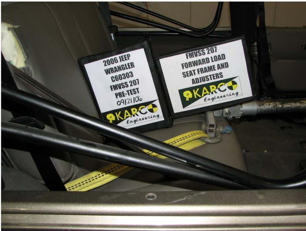
FIGURE 33. Forward Load on Seat Frame and Adjusters, P3, Pre-Test
