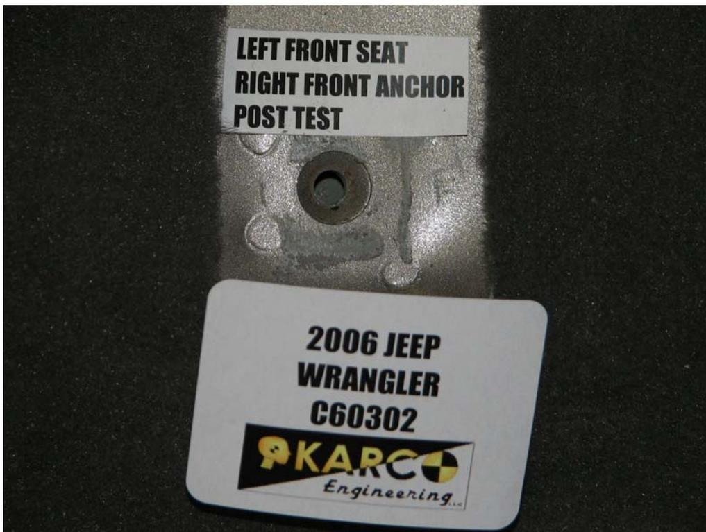
FIGURE 52. Floor Pan Anchor, P1, Post-Test
