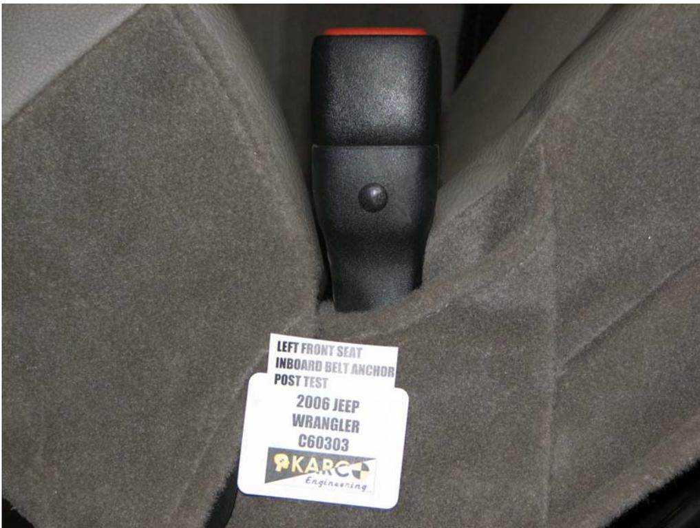
FIGURE 70. Belt Anchor, P1, Post-Test
