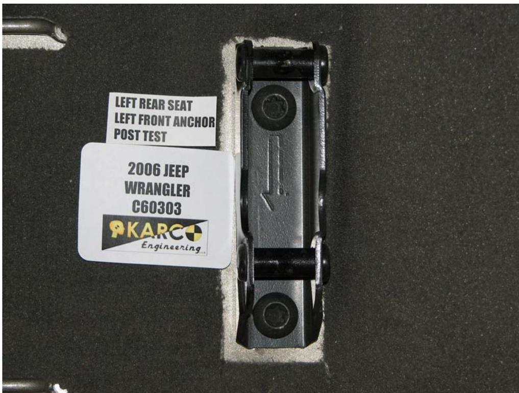
FIGURE 104. Floor Pan Anchor, P3 and P4, Post-Test
