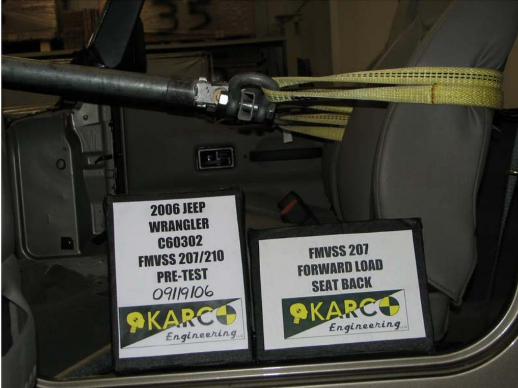
FIGURE 15. Forward Load on Seat Back, P1, Pre-Test
