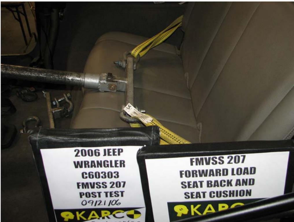
FIGURE 28. Forward Load on Seat Back, P4, Post-Test
