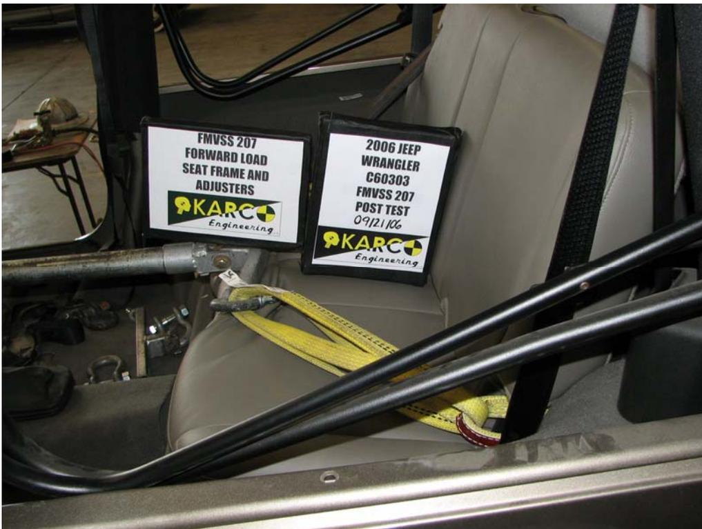
FIGURE 32. Forward Load on Seat Frame and Adjusters, P4, Post-Test
