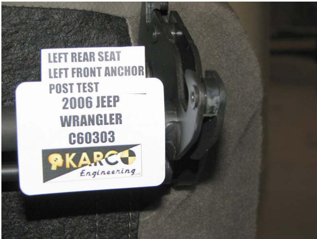
FIGURE 106. Seat Anchor, P3 and P4, Post-Test
