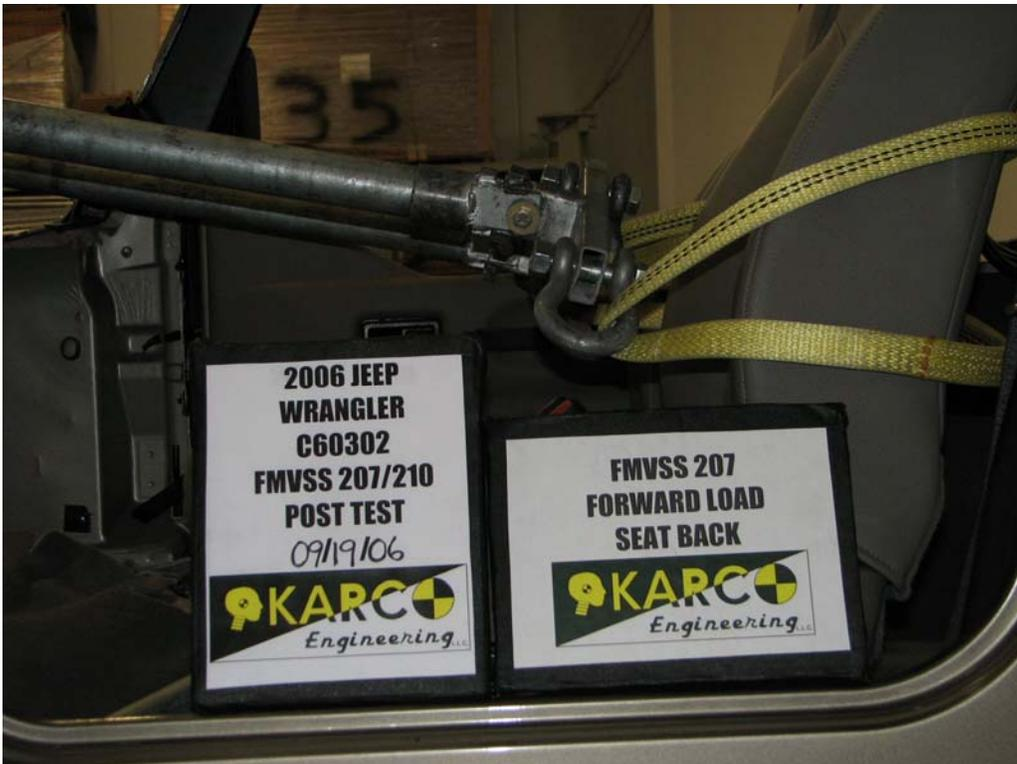
FIGURE 16. Forward Load on Seat Back, P1, Post-Test
