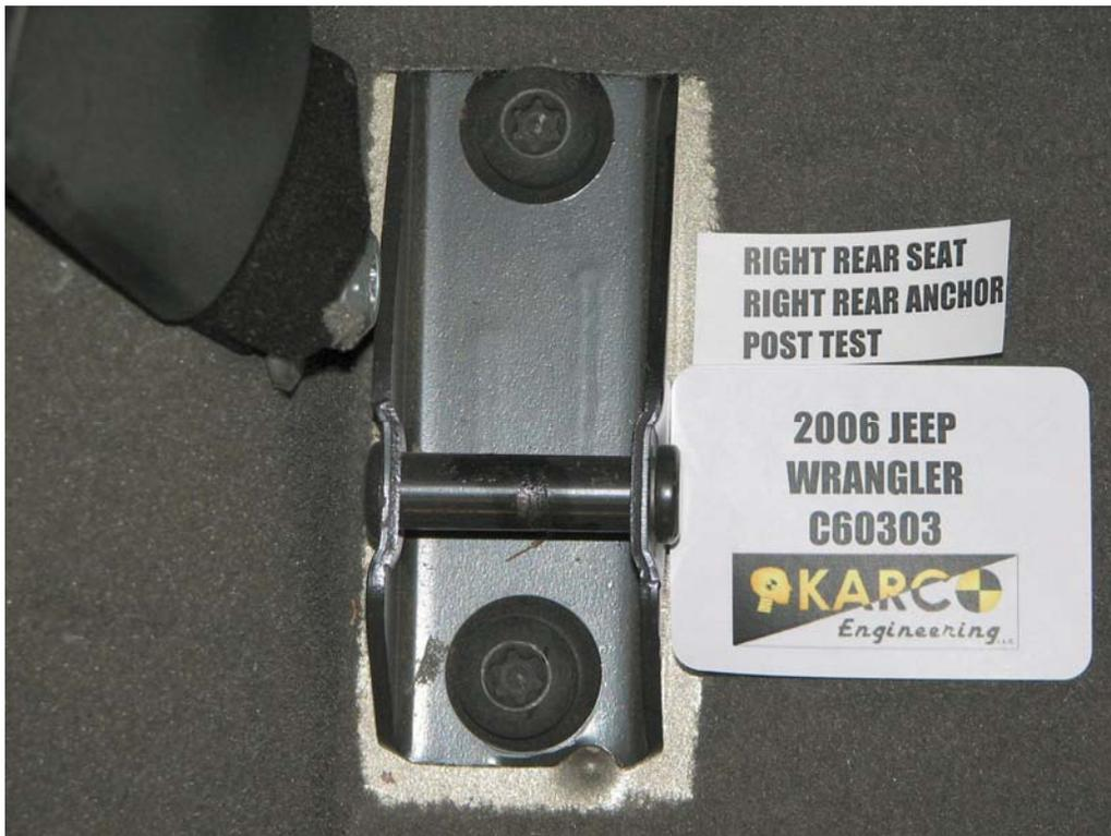
FIGURE 116. Floor Pan Anchor, P3 and P4, Post-Test
