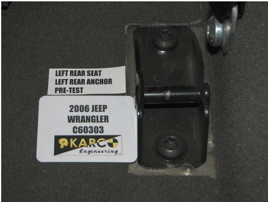
FIGURE 111. Floor Pan Anchor, P3 and P4, Pre-Test
