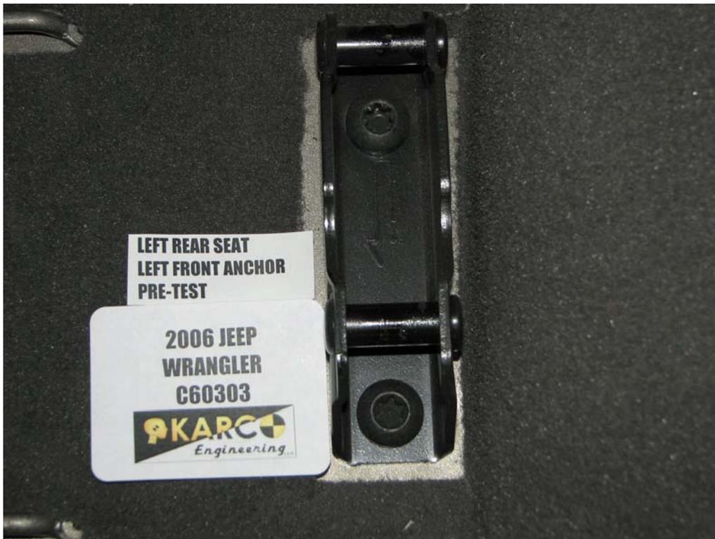
FIGURE 103. Floor Pan Anchor, P3 and P4, Pre-Test
