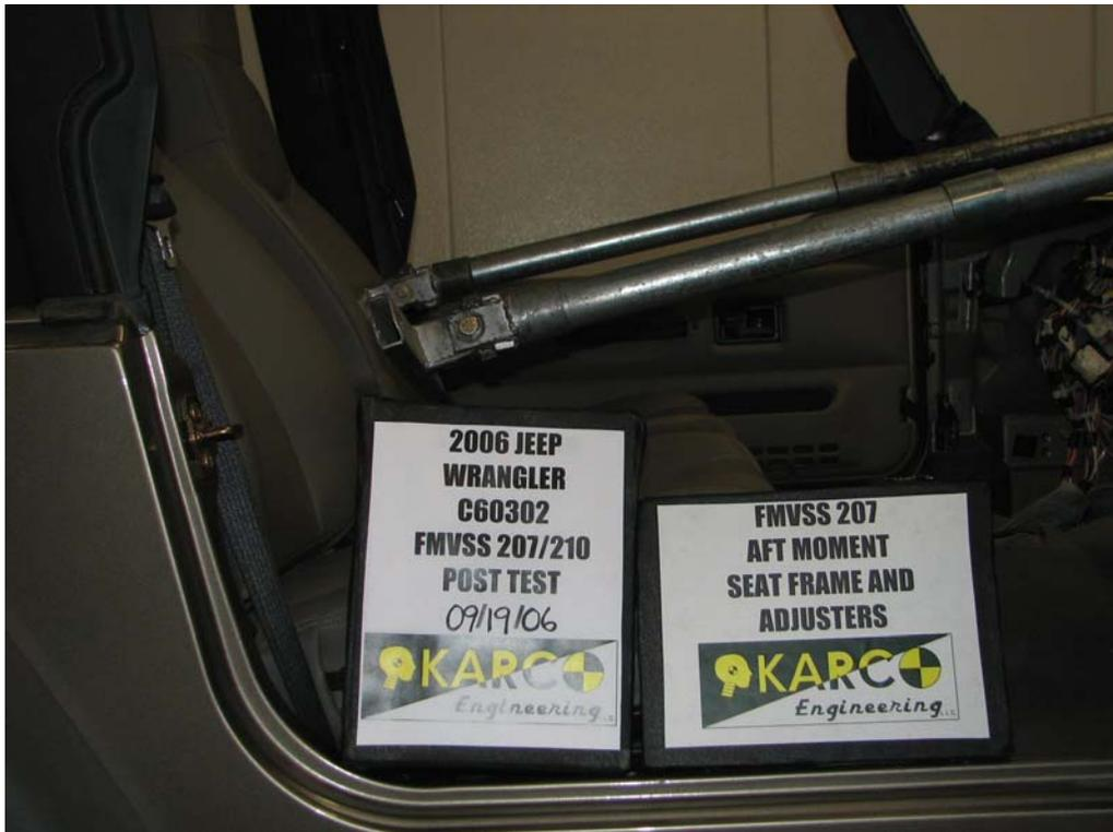
FIGURE 14. Aft Moment on Seat Back, P2, Post-Test
