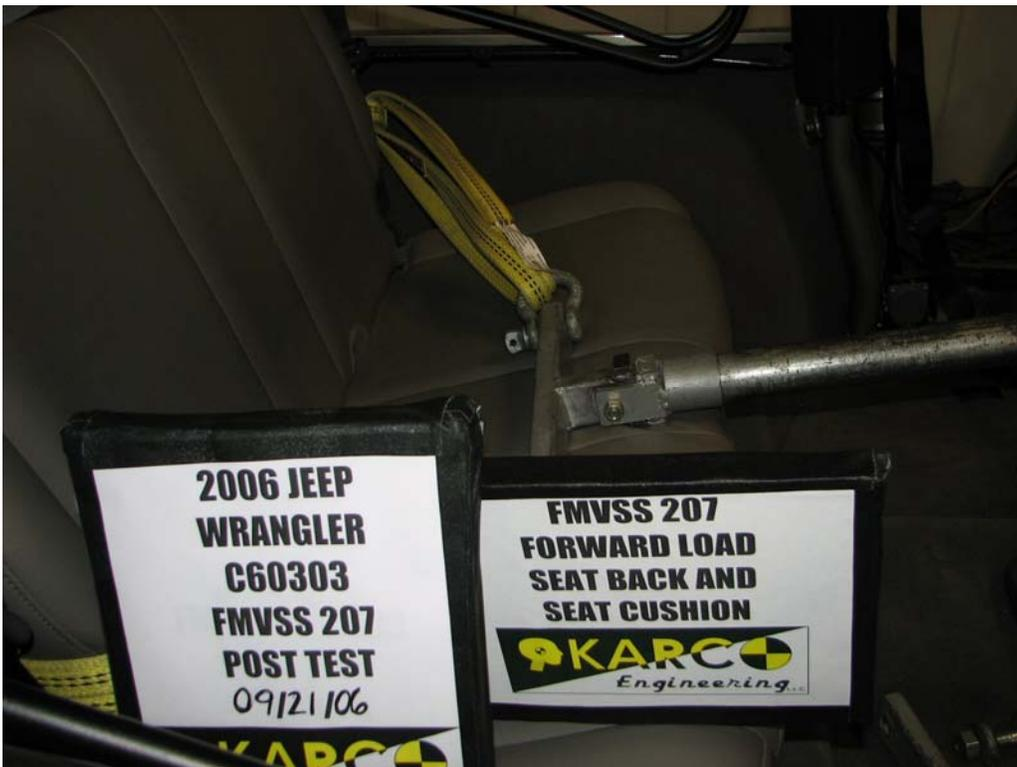
FIGURE 30. Forward Load on Seat Back, P3, Post-Test
