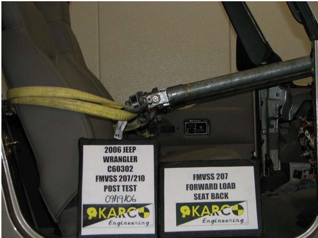
FIGURE 18. Forward Load on Seat Back, P2, Post-Test
