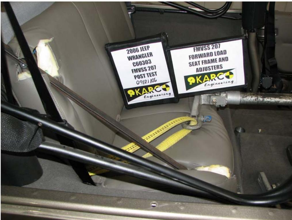
FIGURE 34. Forward Load on Seat Frame and Adjusters, P3, Post-Test
