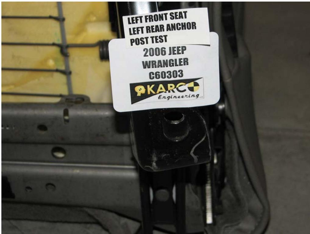
FIGURE 58. Seat Anchor, P1, Post-Test
