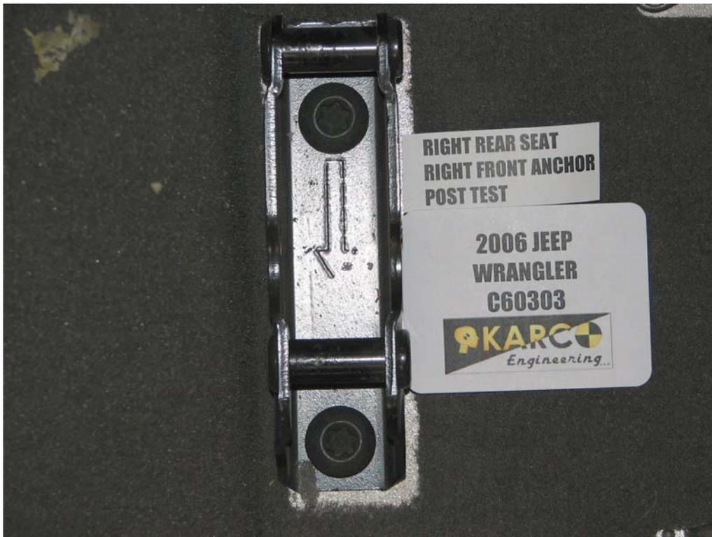
FIGURE 108. Floor Pan Anchor, P3 and P4, Post-Test
