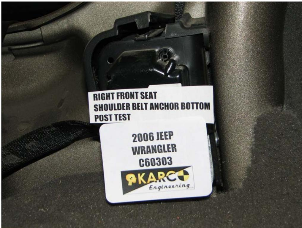
FIGURE 94. Shoulder Belt Anchor, P2, Post-Test
