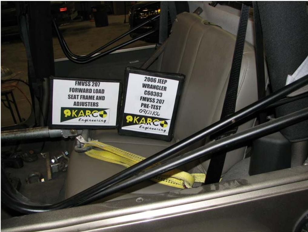
FIGURE 31. Forward Load on Seat Frame and Adjusters, P4, Pre-Test
