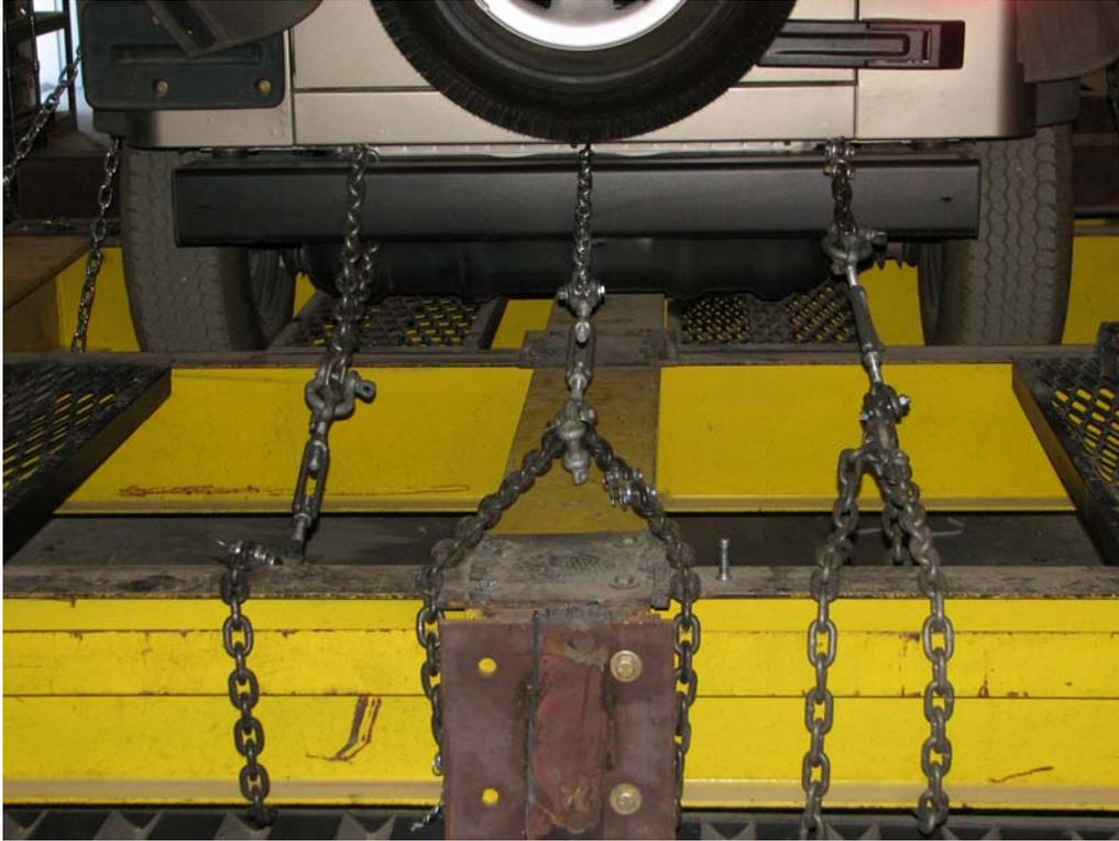
FIGURE 9. Vehicle Mounted in Test Fixture
