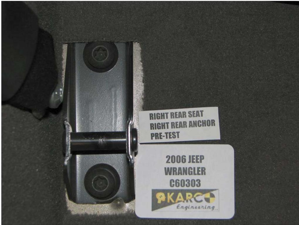
FIGURE 115. Floor Pan Anchor, P3 and P4, Pre-Test
