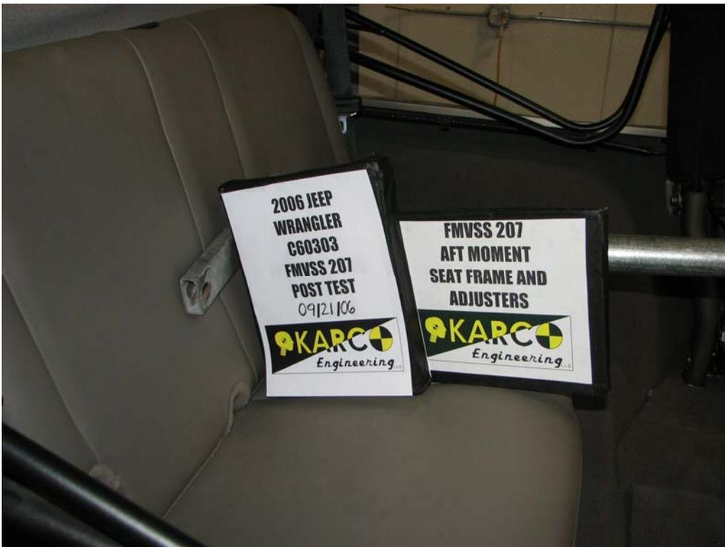
FIGURE 38. Aft Moment on Seat Back, P3, Post-Test
