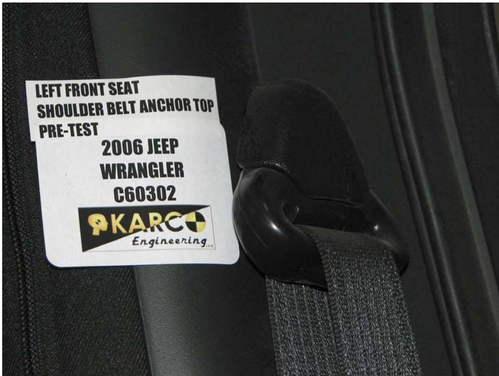
FIGURE 63. Shoulder Belt Anchor, P1, Pre-Test
