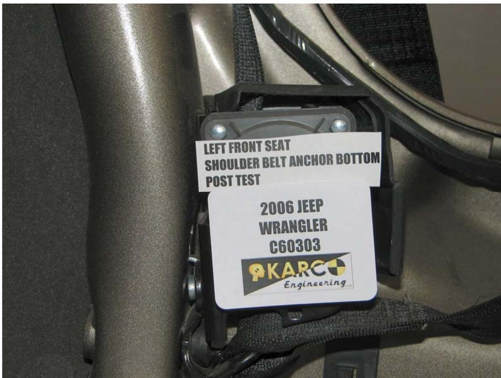
FIGURE 66. Shoulder Belt Anchor, P1, Post-Test
