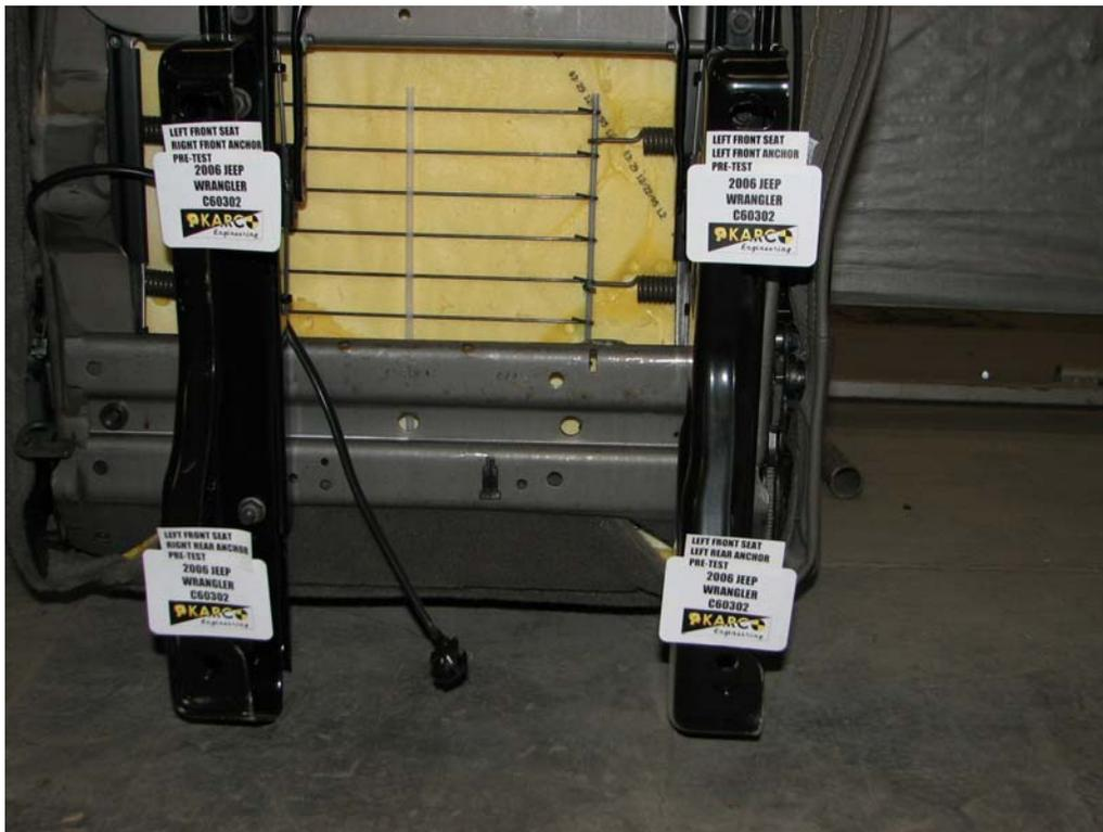
FIGURE 45. Seat Anchors, P1 Overall, Pre-Test
