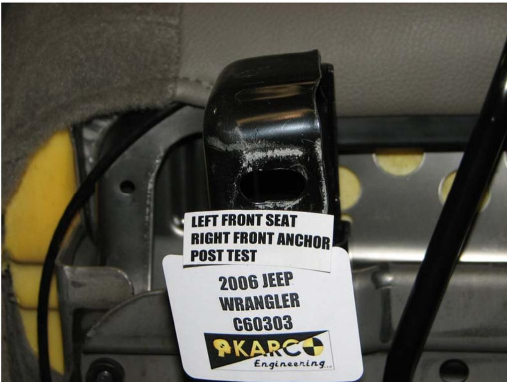
FIGURE 54. Seat Anchor, P1, Post-Test
