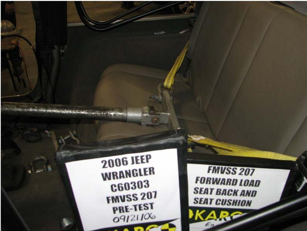
FIGURE 27. Forward Load on Seat Back, P4, Pre-Test
