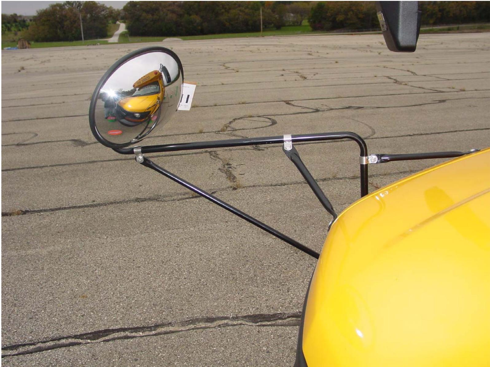
Photo 9 - Left Front Cross View Mirror and Mounting
