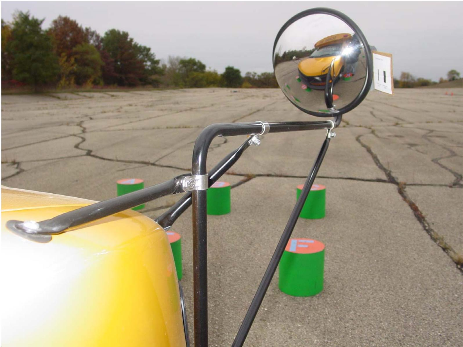
Photo 6 - Right Front Cross View Mirror and Mounting
