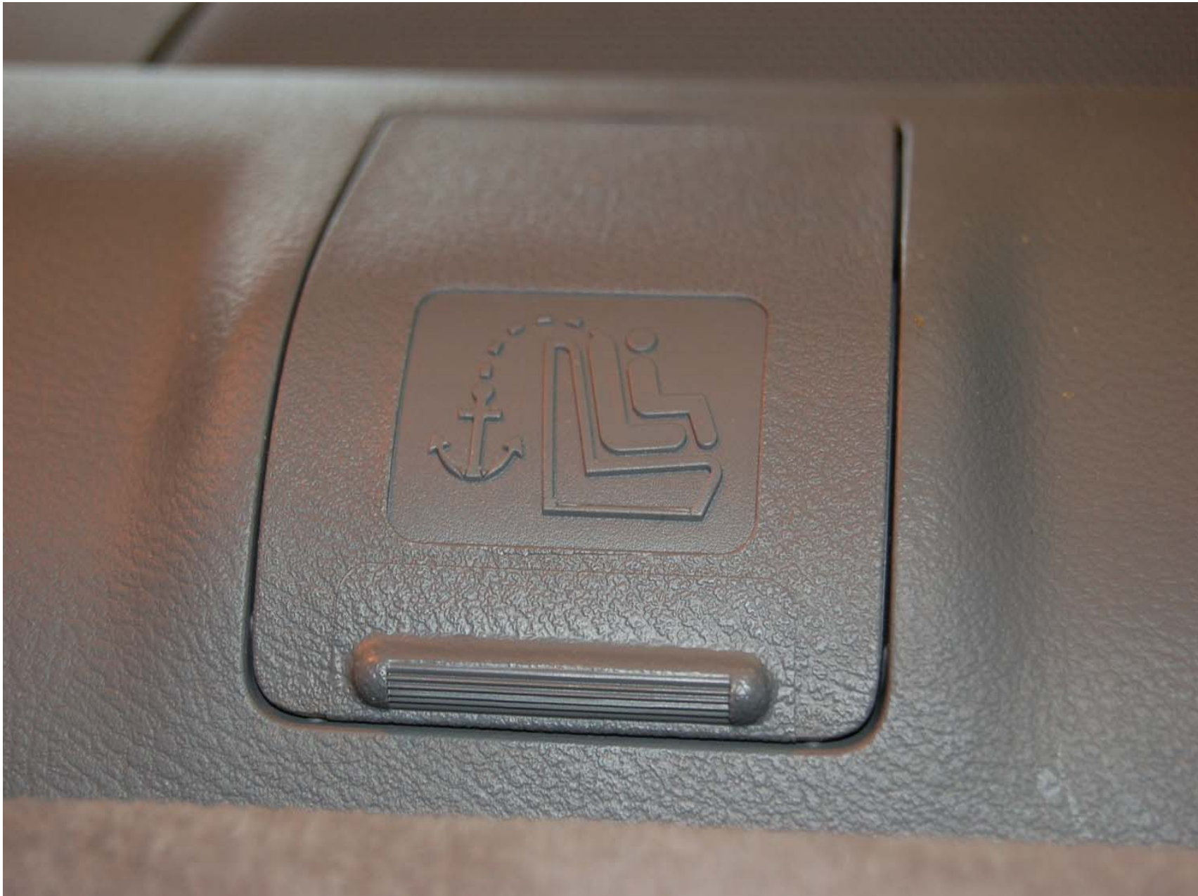
FIGURE 5.14 CAP OVER TOP TETHER ANCHOR
