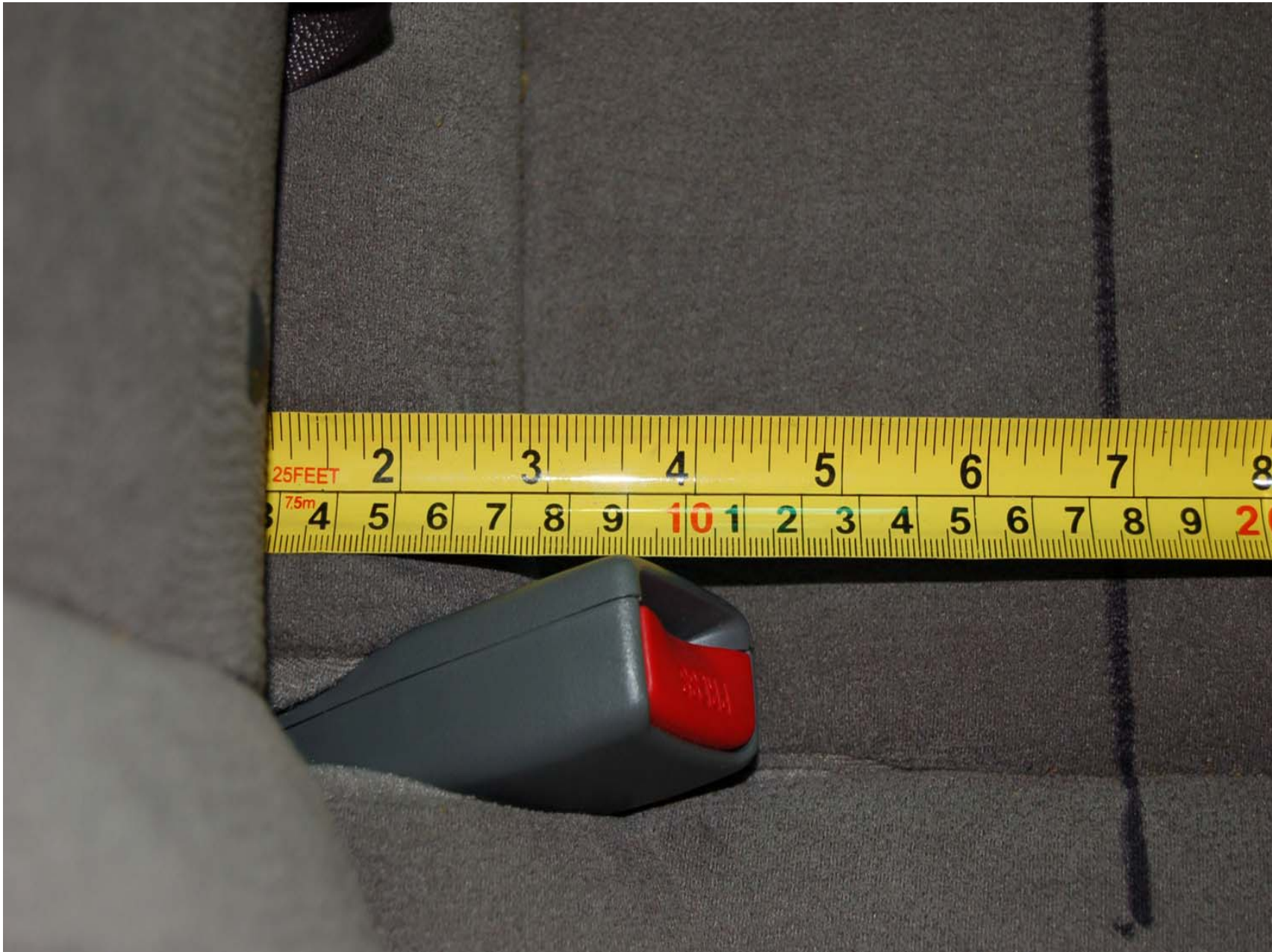
FIGURE 5.26 VIEW OF INBOARD "H" POINT MEASUREMENT LEFT SEAT
