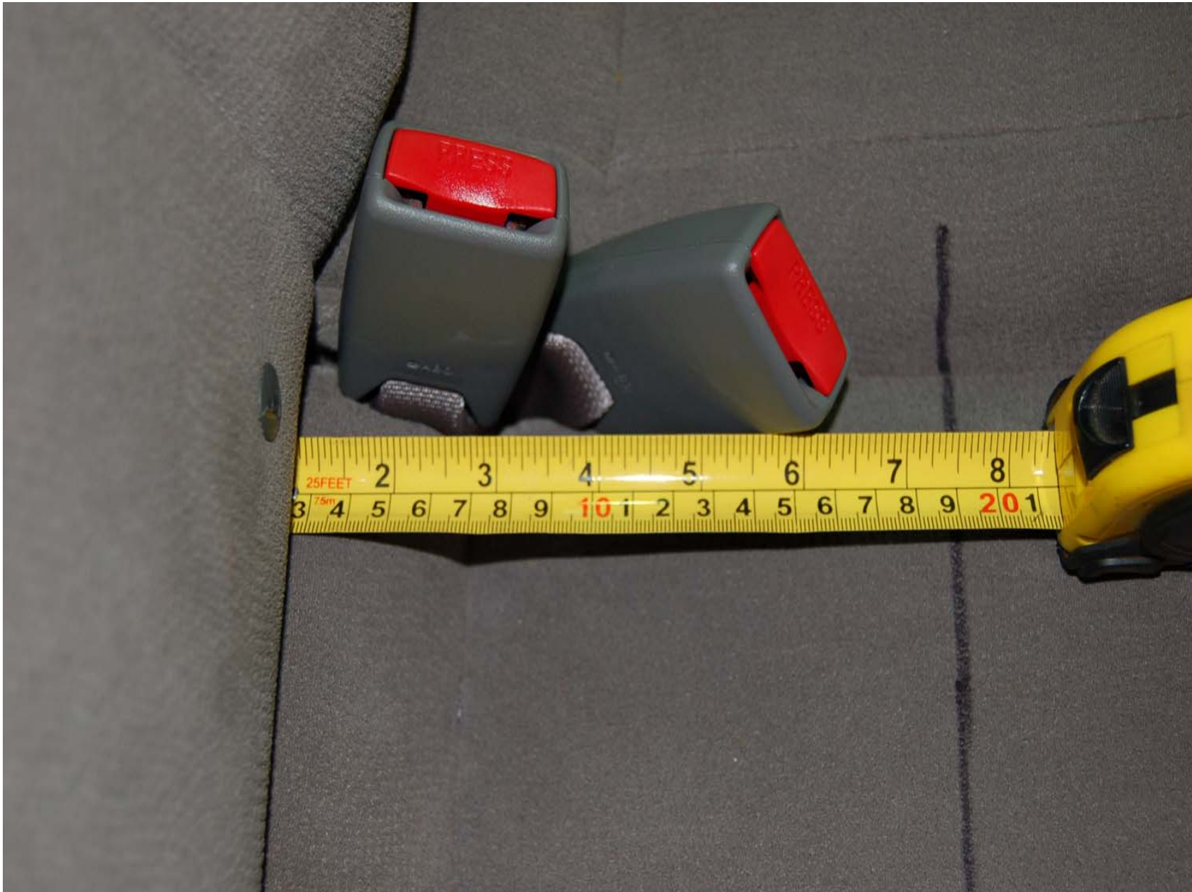
FIGURE 5.24 VIEW OF INBOARD "H" POINT MEASUREMENT RIGHT SEAT
