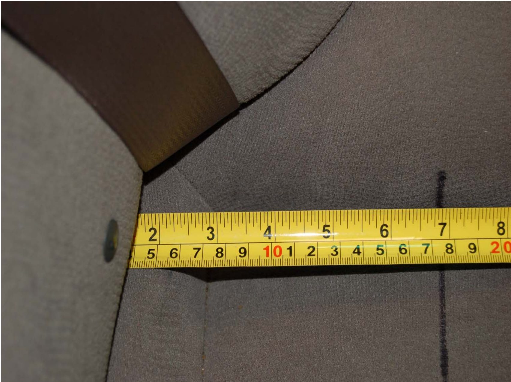
FIGURE 5.25 VIEW OF OUTBOARD "H" POINT MEASUREMENT IN 2 ND ROW LEFT SEAT
