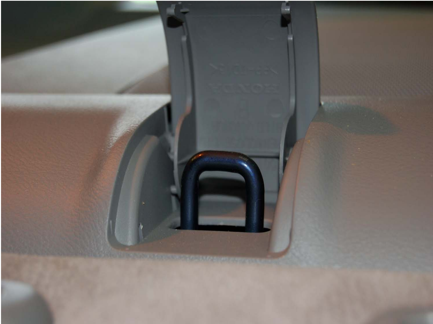
FIGURE 5.12 PRE-TEST 2 ND ROW LEFT TOP TETHER ANCHOR
