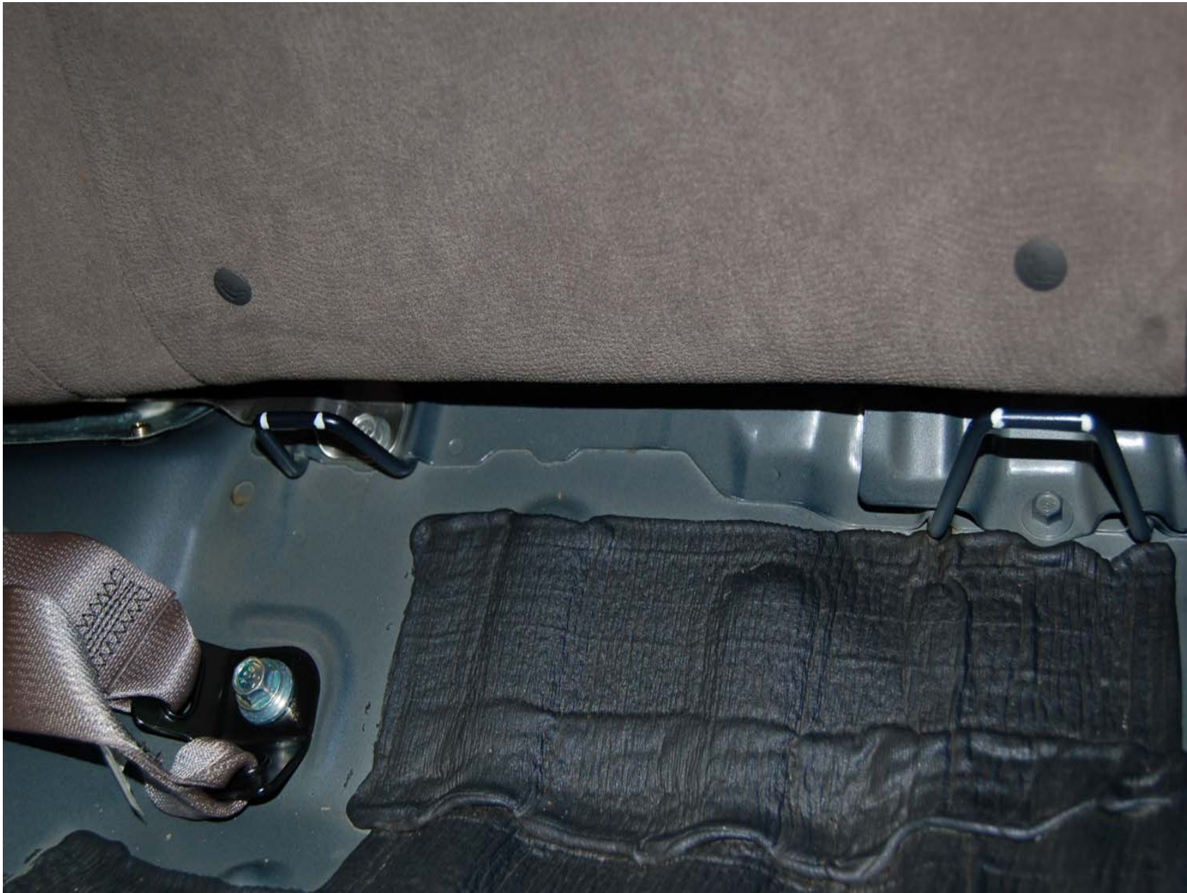
FIGURE 5.11 PRE-TEST 2 ND ROW LEFT LOWER ANCHORS
