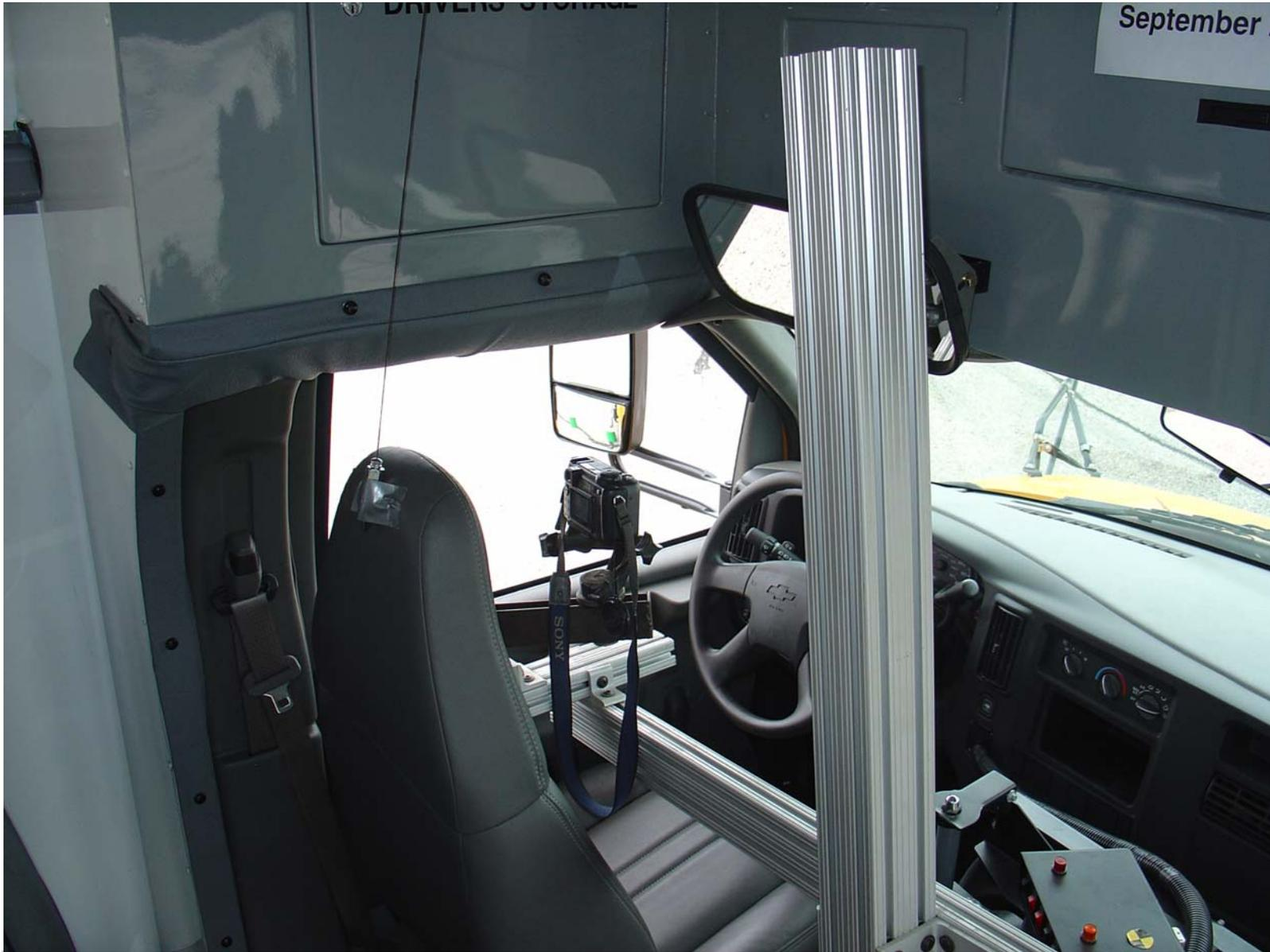
Photo 10 - Field of View Instrument Setup
