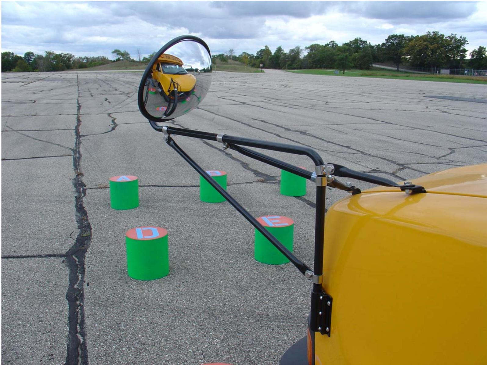
Photo 8 - Left Front Cross View Mirror and Mounting
