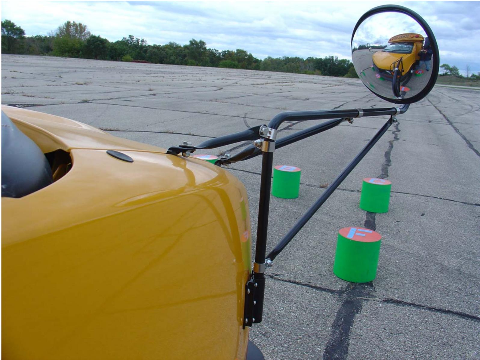
Photo 5 - Right Front Cross View Mirror and Mounting
