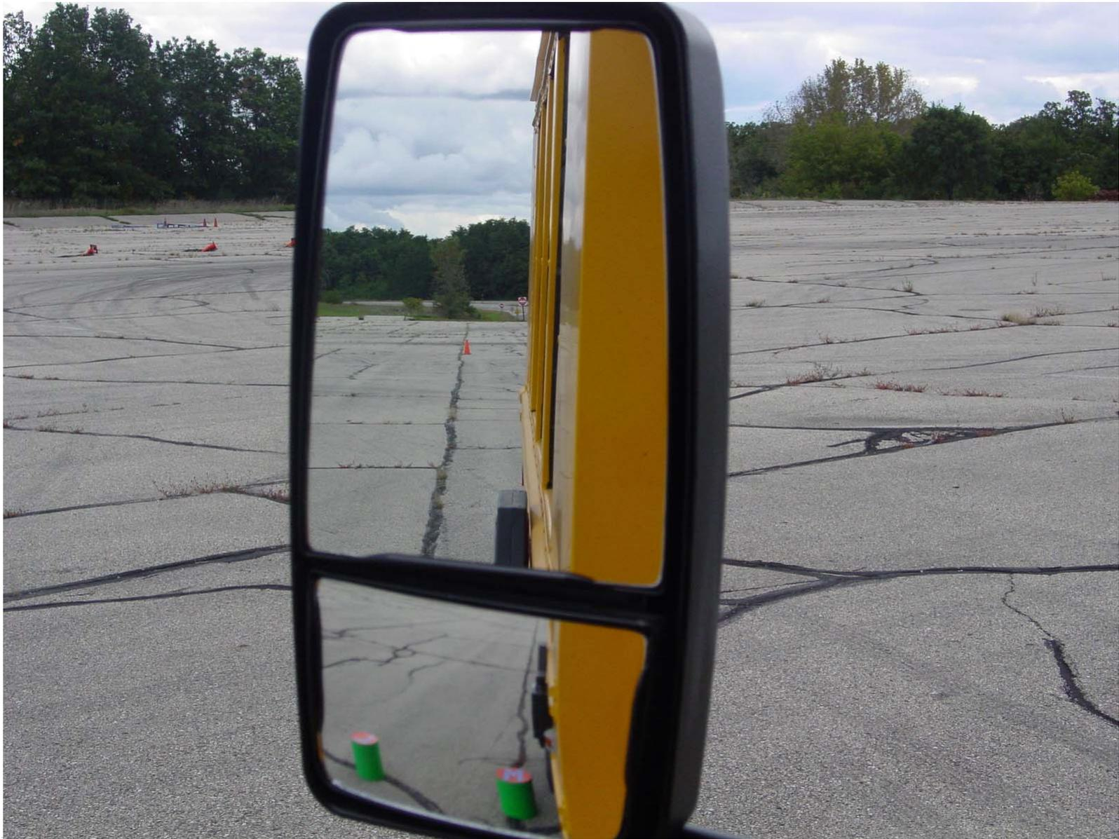
Photo 15 - Mirror #3 and #5 System A Field of View
