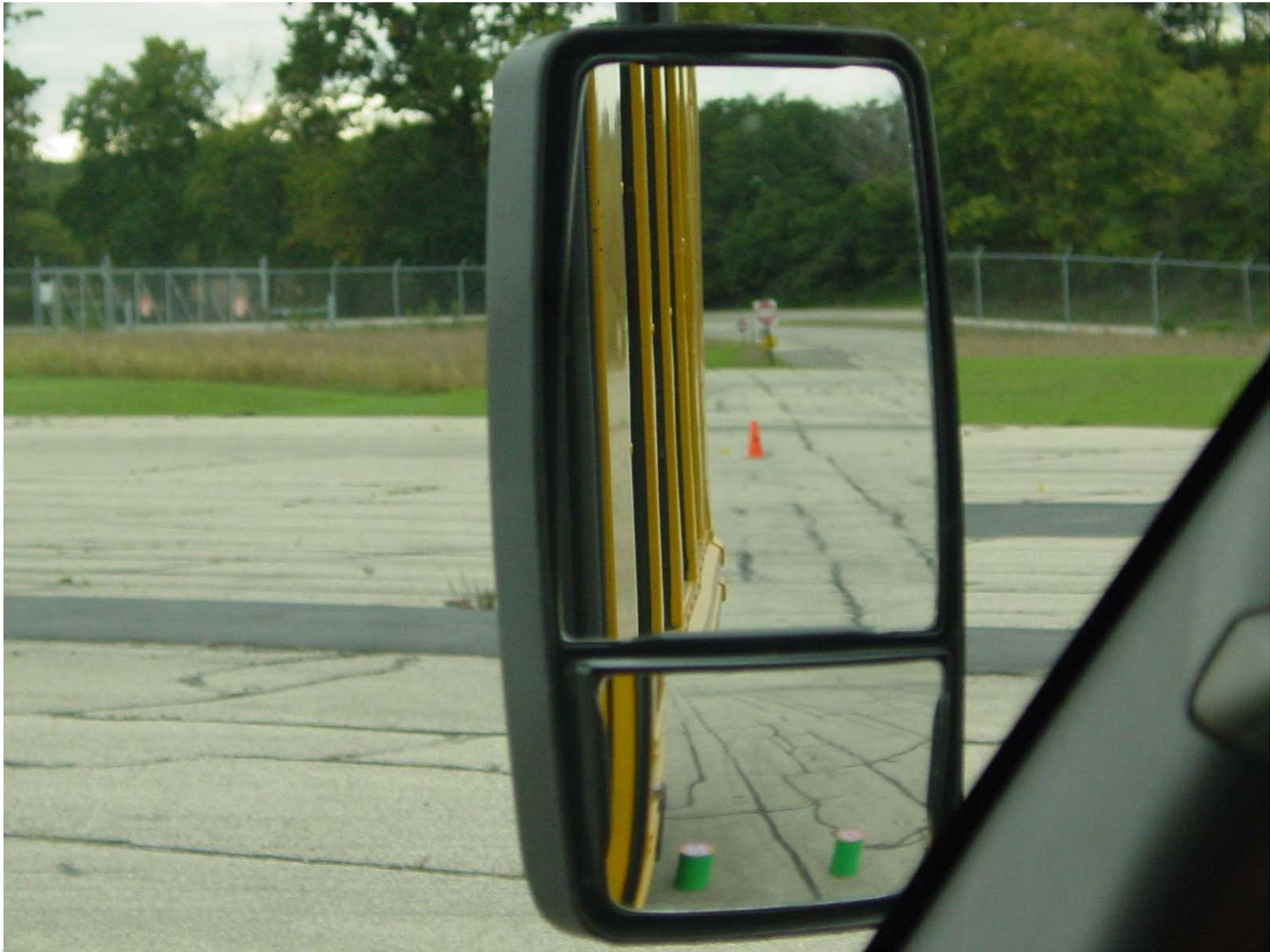
Photo 14 - Mirror #4 and #6 System A Field of View
