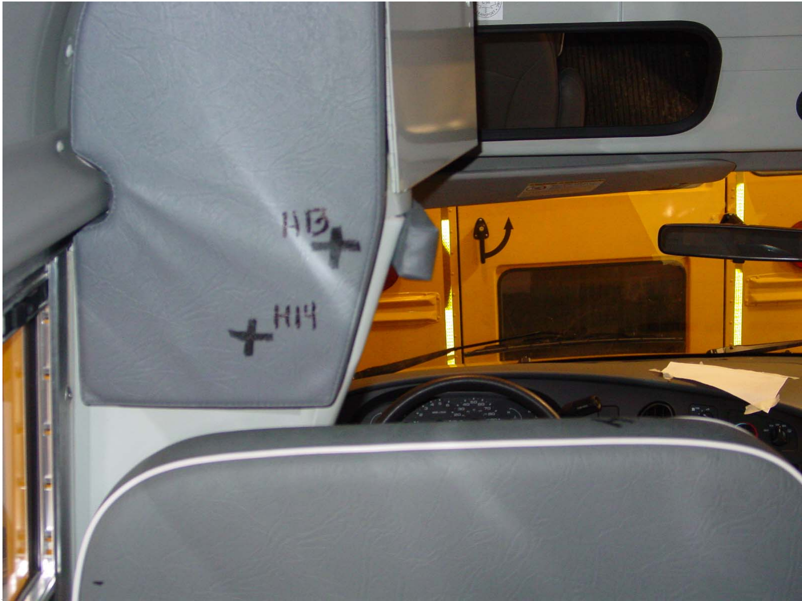
Post-Test of Head Impact Locations on Bulkhead
