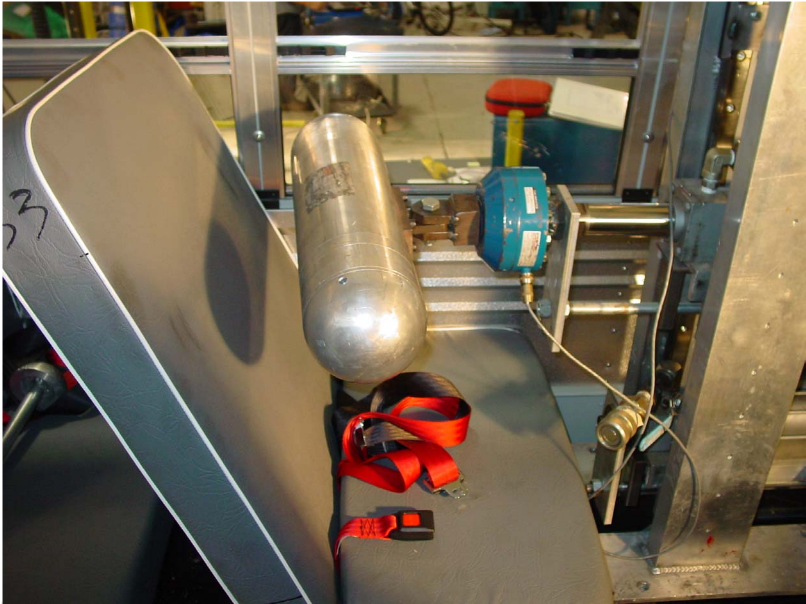
Post-Test of Seat Back S3 Force Deflection Rearward Test
