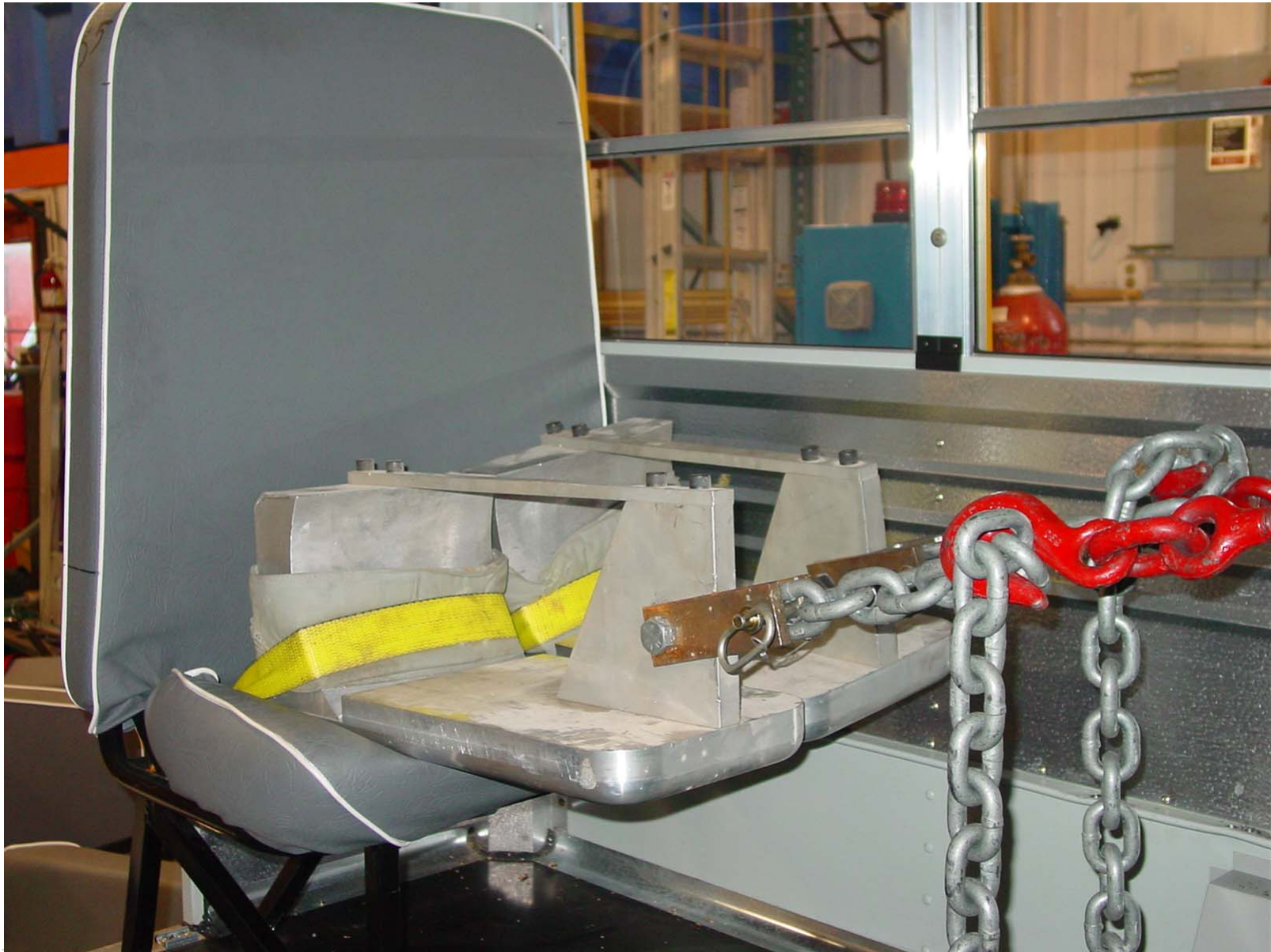
Pre-Test Seat Belt Assembly Anchorage on Seat S5
