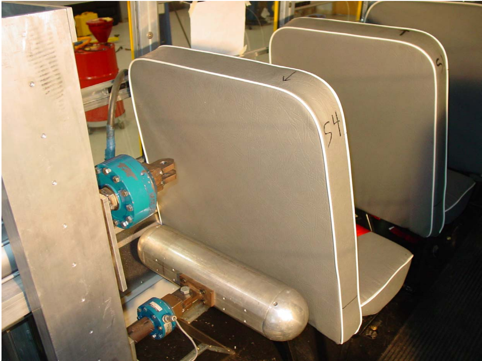
Pre-Test of Seat Back S4 Force Deflection Forward Test (In S2 Location)
