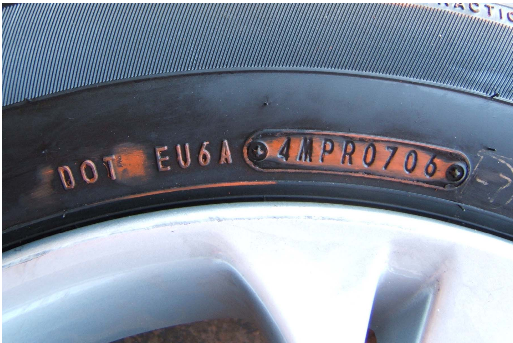
FIGURE 5.7 TIRE SHOWING DOT SERIAL NUMBER
