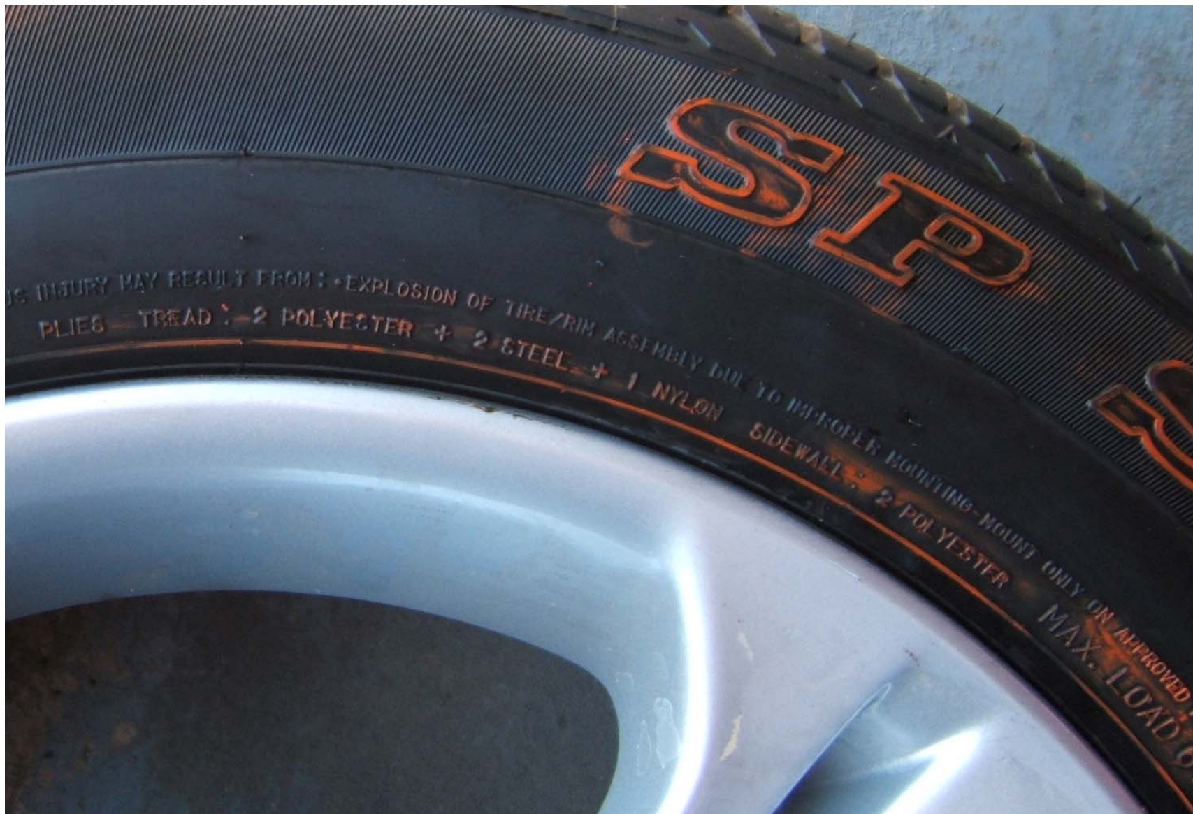
FIGURE 5.9 TIRE SHOWING SIDEWALL/TREAD CONSTRUCTION
