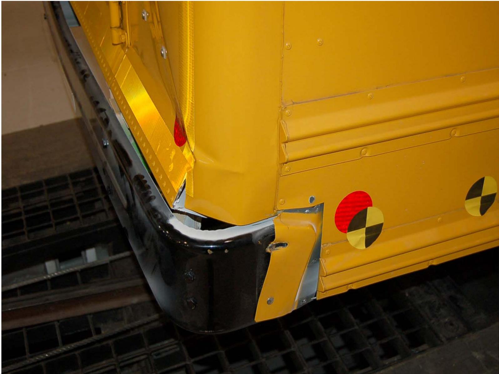
Post-Test Vehicle Damage Right Rear Bumper
