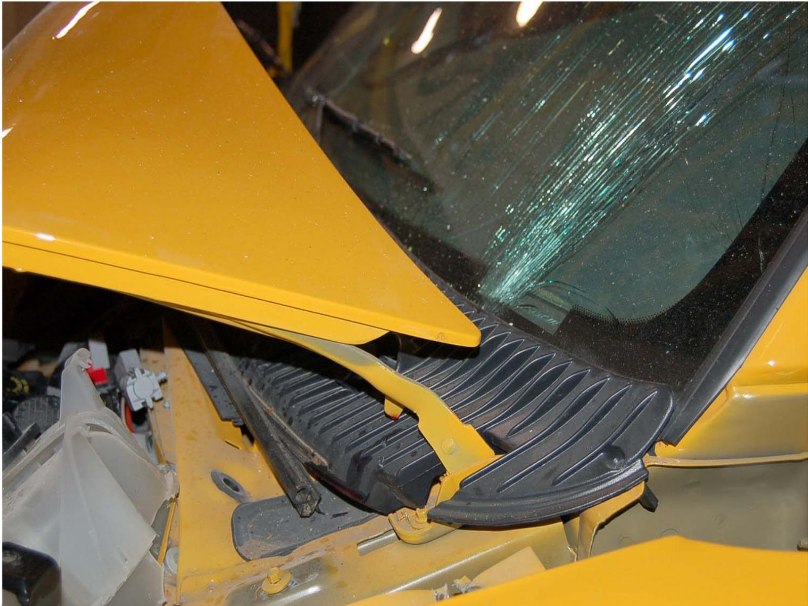
Post-Test Vehicle Damage Left Side View of Hood
