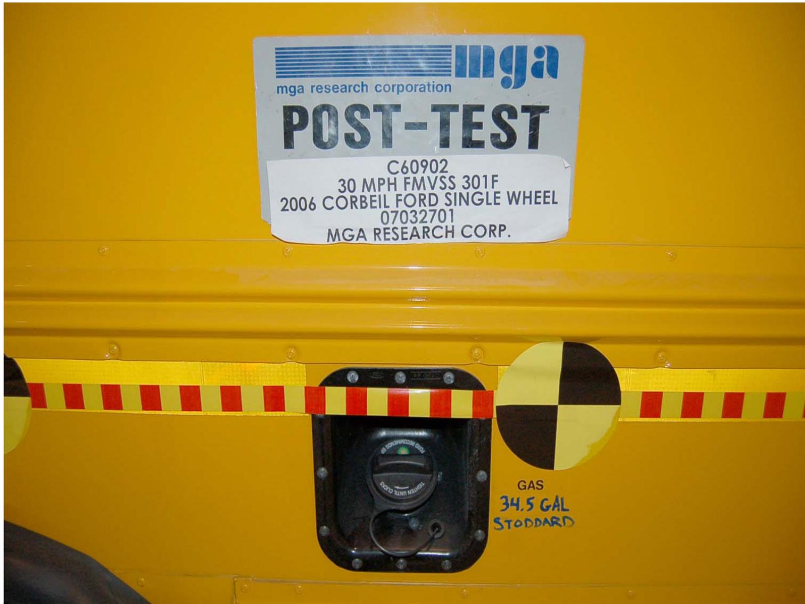
Post-Test Fuel Filler Cap
