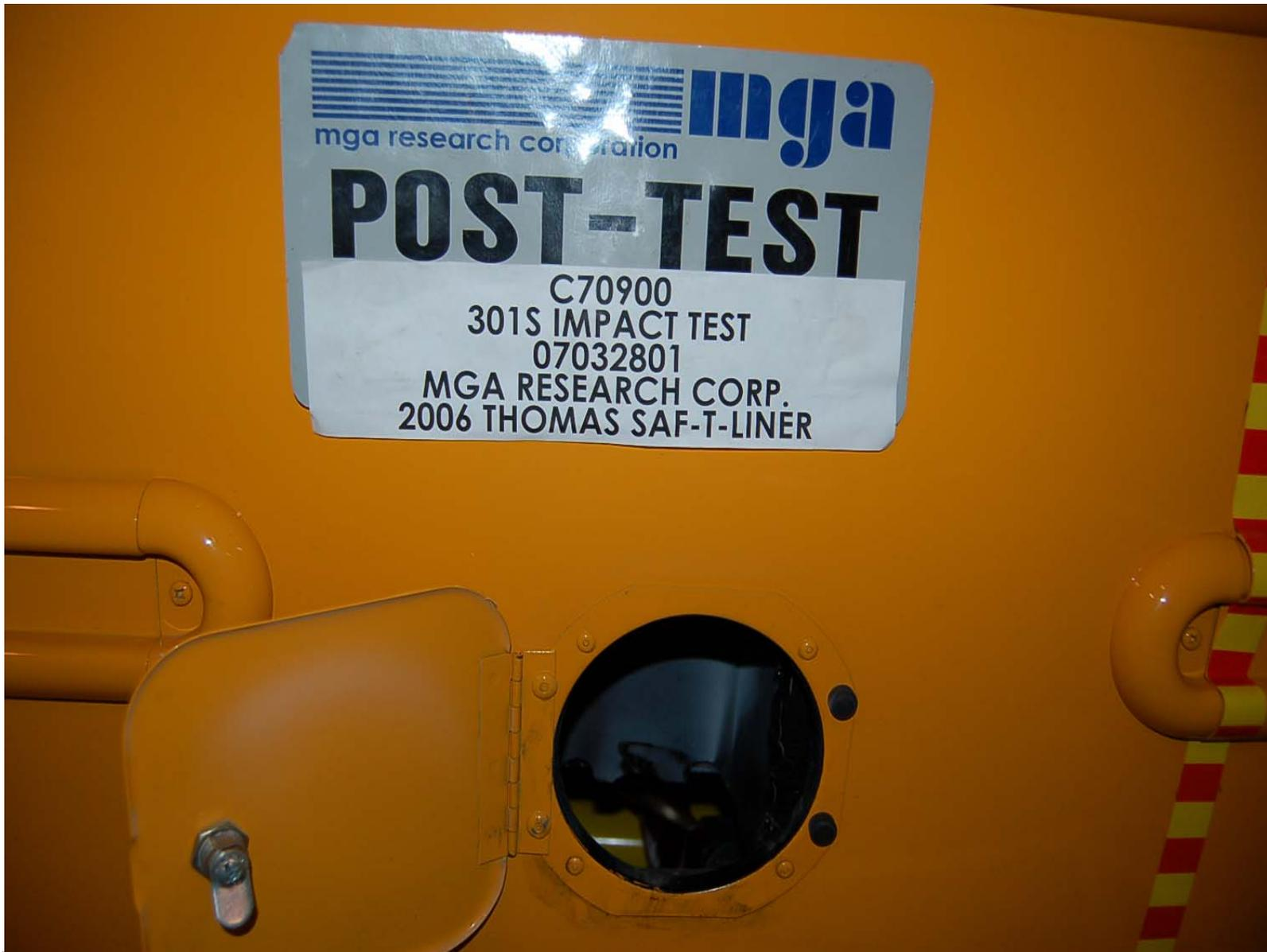
Post-Test of Fuel Filler Cap
