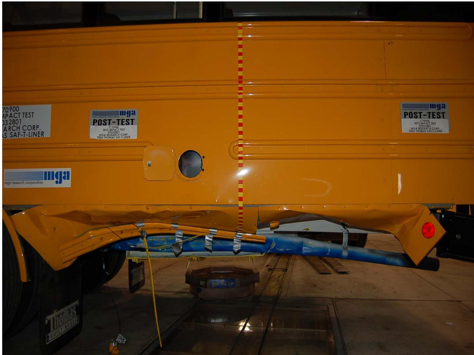
Post-Test Left Rear Side of the Bus
