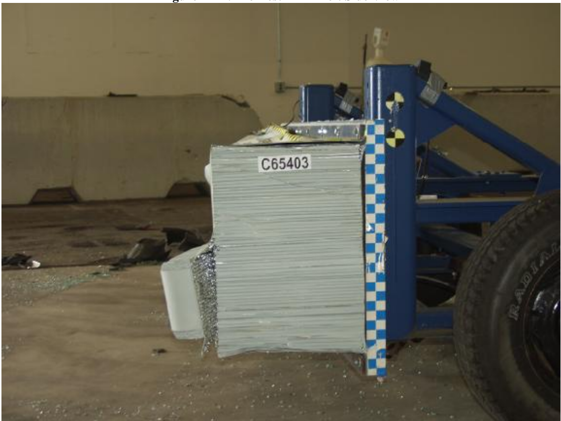
Figure A-22: Post-Test MDB Left Side View
