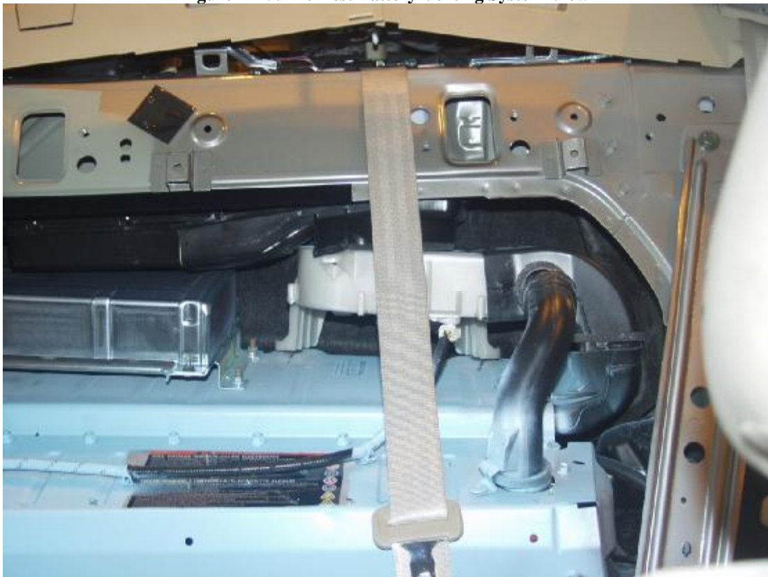
Figure A-16: Post-Test Battery Venting System View
