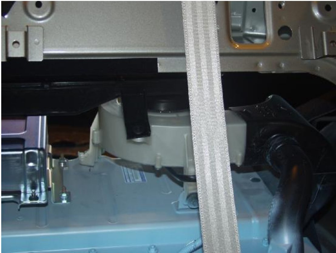
Figure A-15: Pre-Test Battery Venting System View
