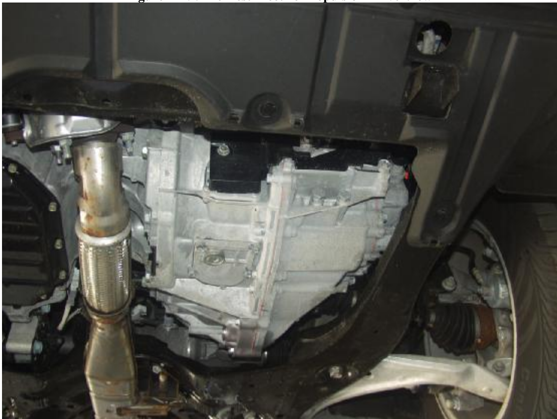
Figure A-20: Post-Test Electric Propulsion Drive View
