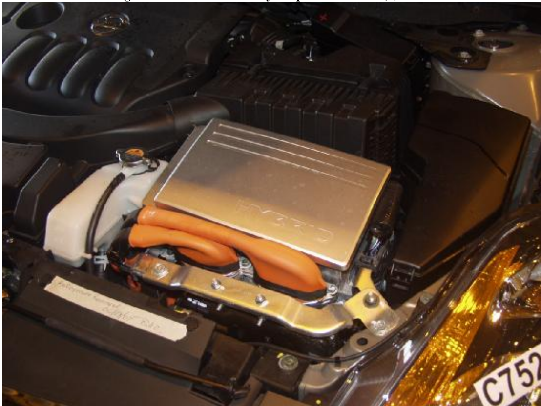
Figure A-8: Post-Test Battery Propulsion Module(S) View
