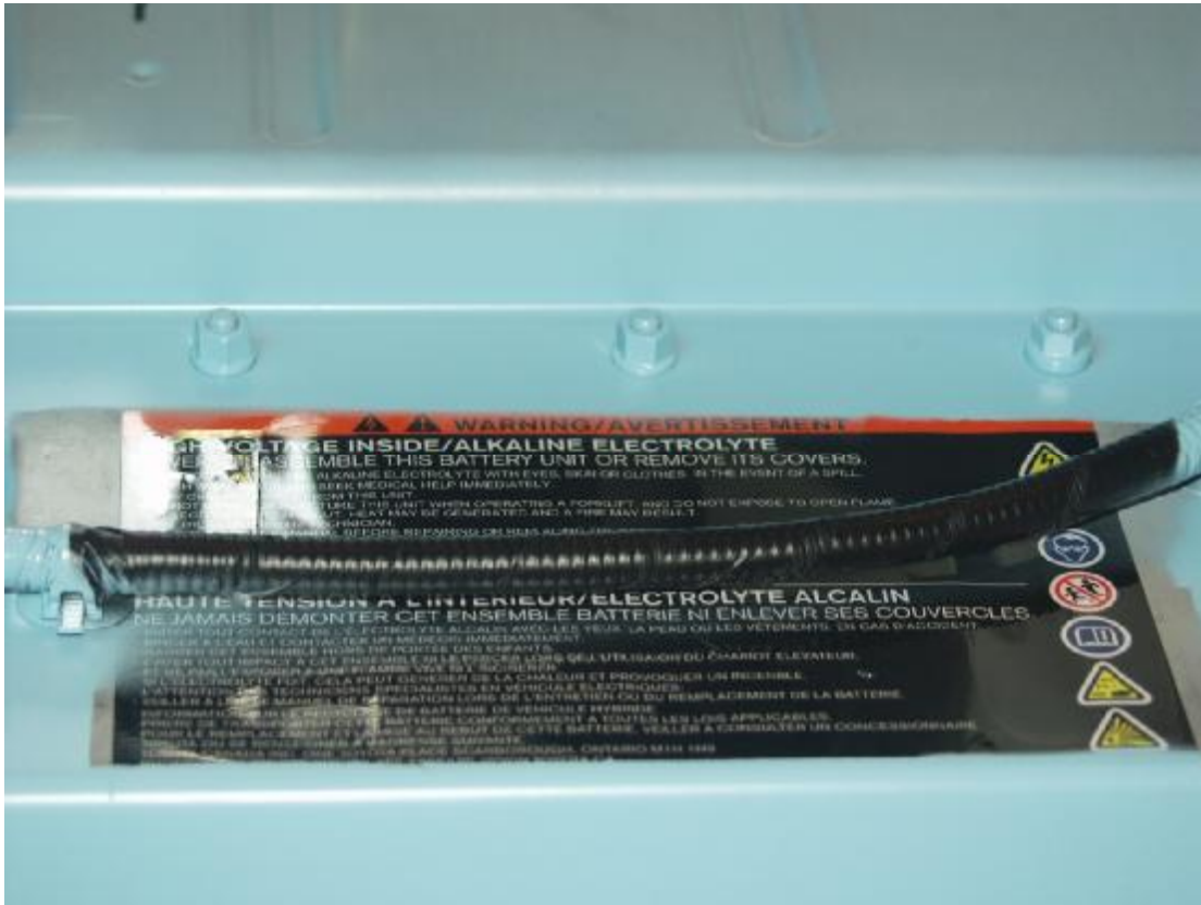
Figure A-3: Vehicle Electric Propulsion System Label
