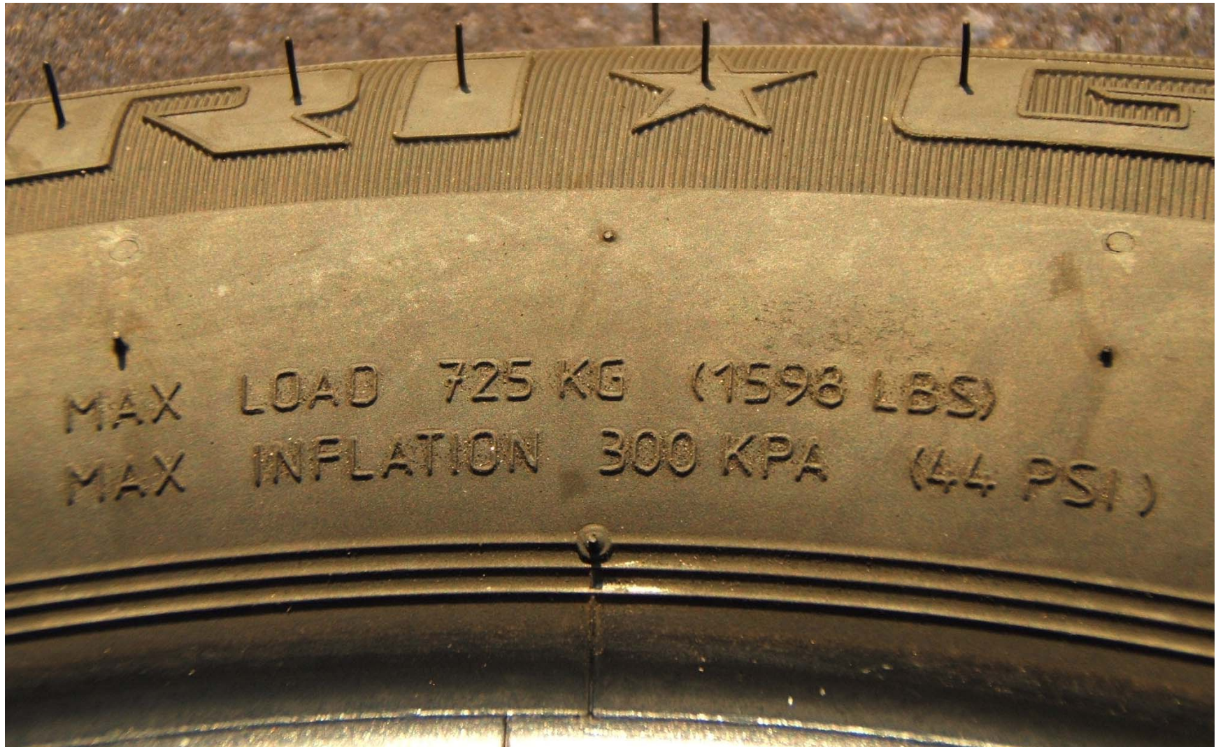
FIGURE 5.8 TIRE SHOWING MAX LOAD RATING AND MAX INFLATION PRESSURE
