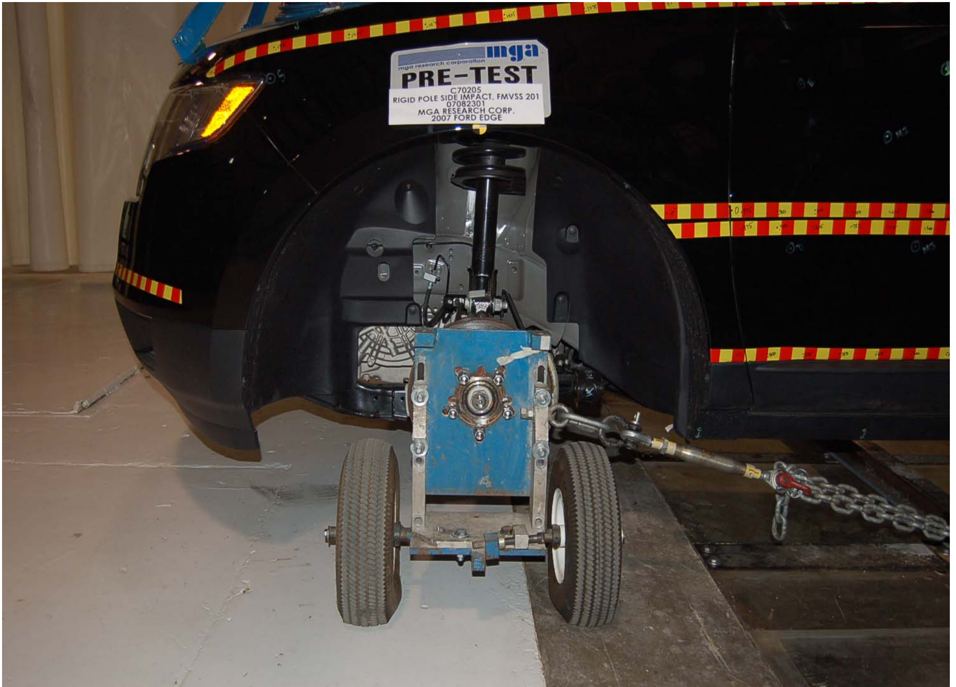
Pre-Test Left Front Wheel Dolly
