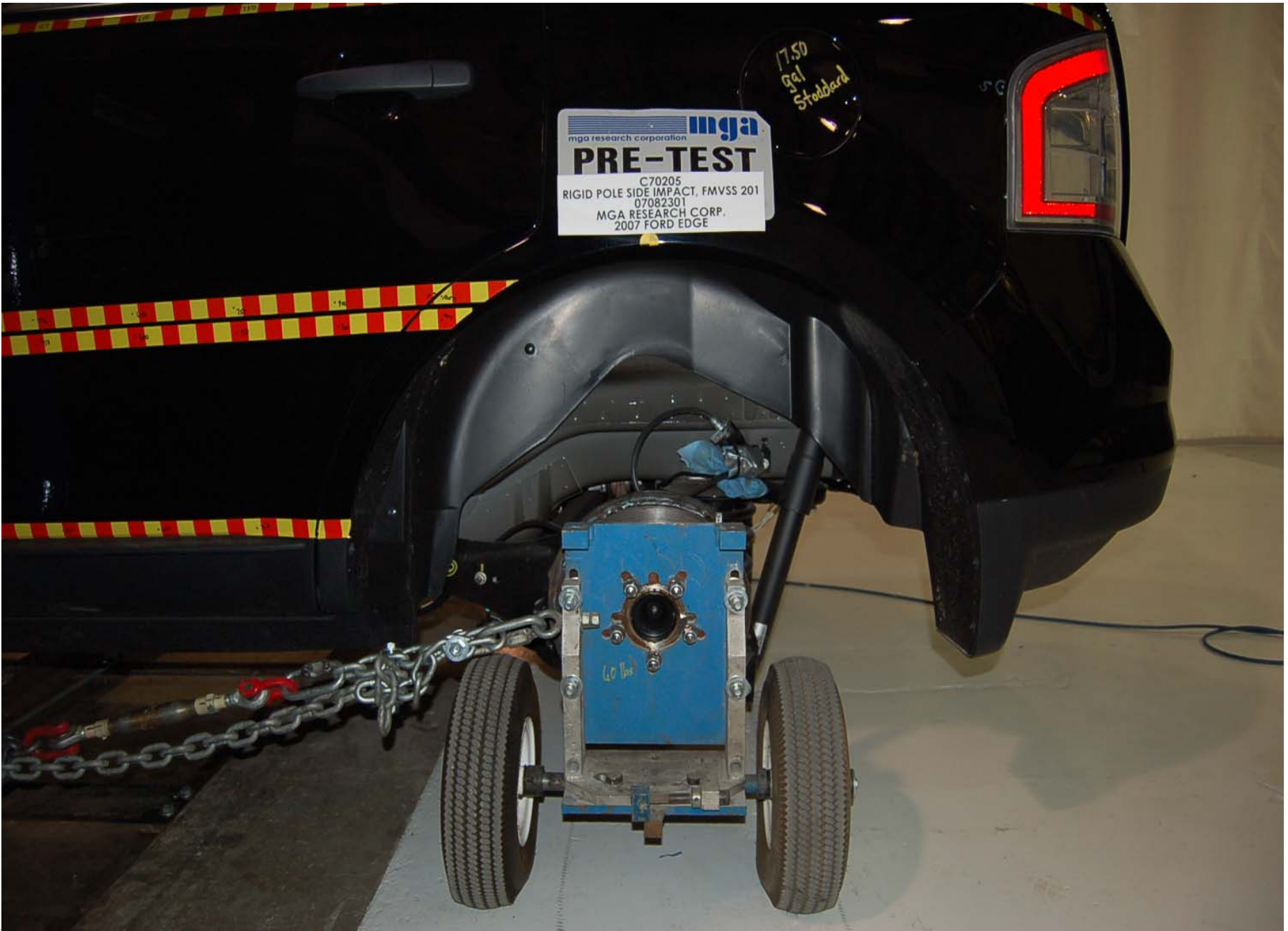
Pre-Test Left Rear Wheel Dolly
