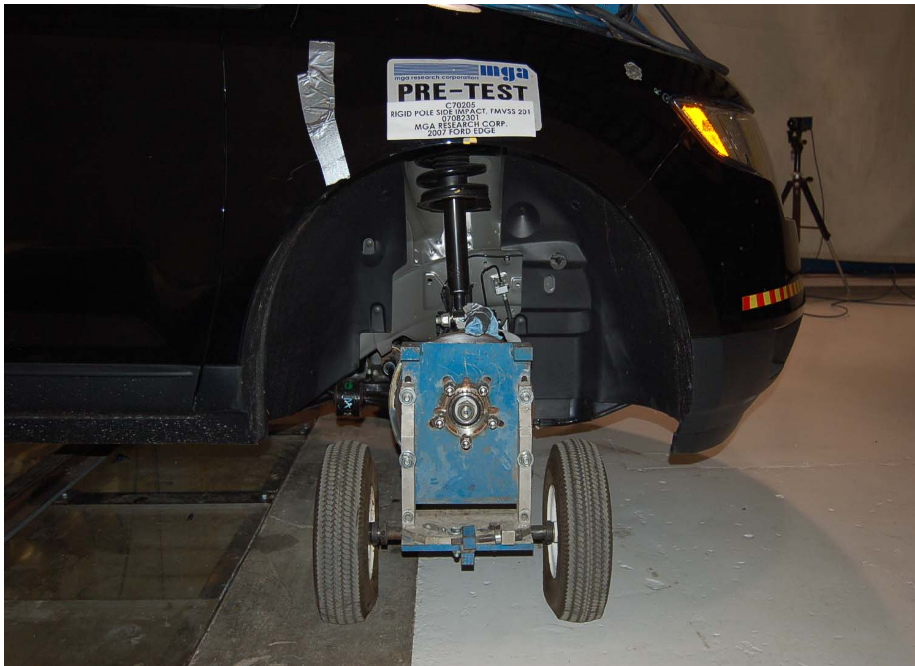
Pre-Test Right Front Wheel Dolly
