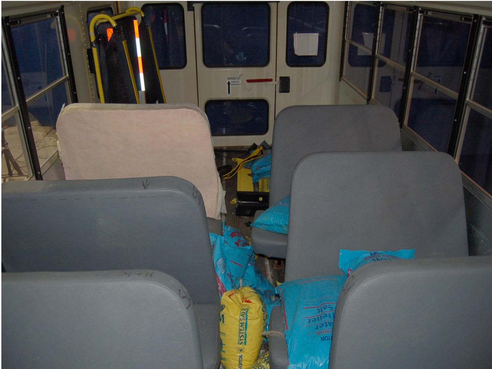
Pre-Test View of Ballast Weight View
