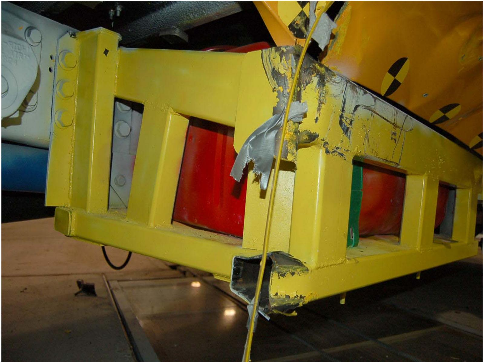
Post-Test Damage Underbody View 1
