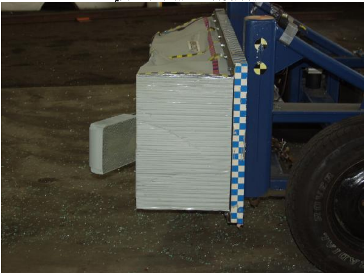
Figure A-22: Post-Test MDB Left Side View
