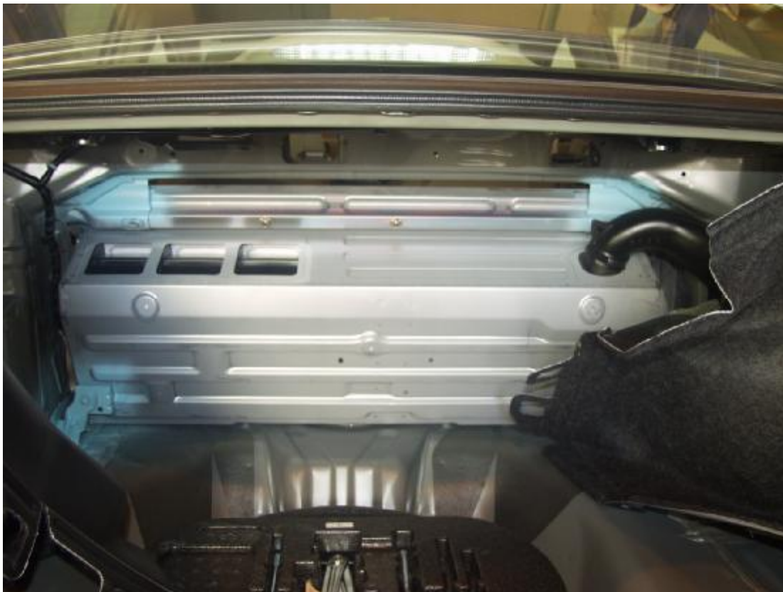
Figure A-41: Pre-Test Battery Venting System View
