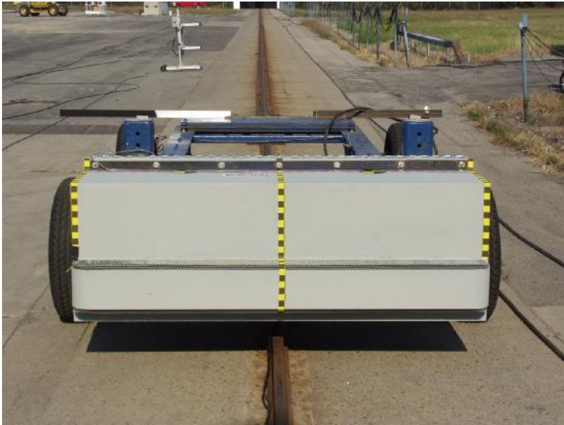
Figure A-23: Pre-Test MDB Front View
