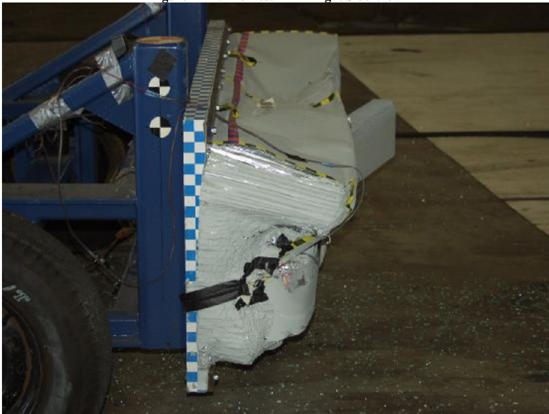
Figure A-28: Post-Test MDB Right Side View
