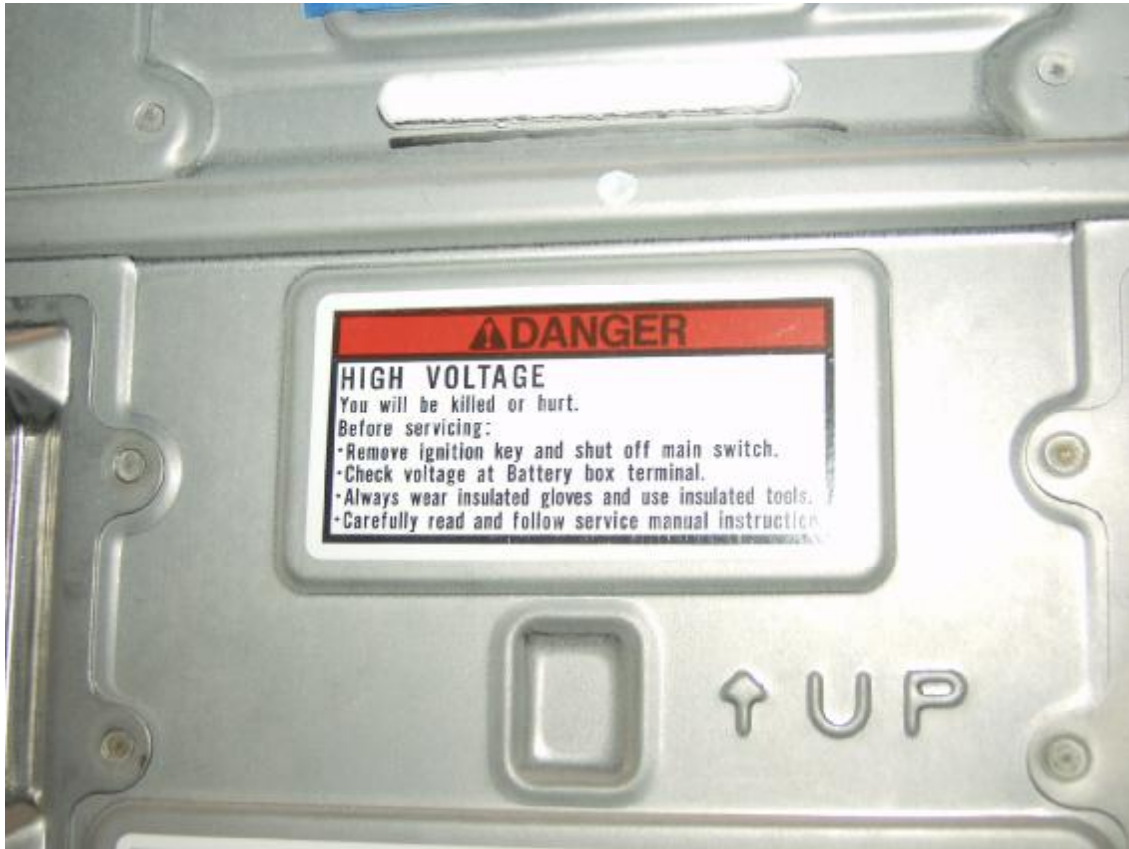
Figure A-3: Vehicle Electric Propulsion System Label
