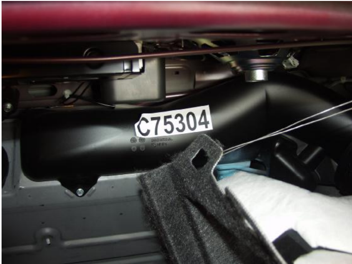
Figure A-15: Pre-Test Battery Venting System View
