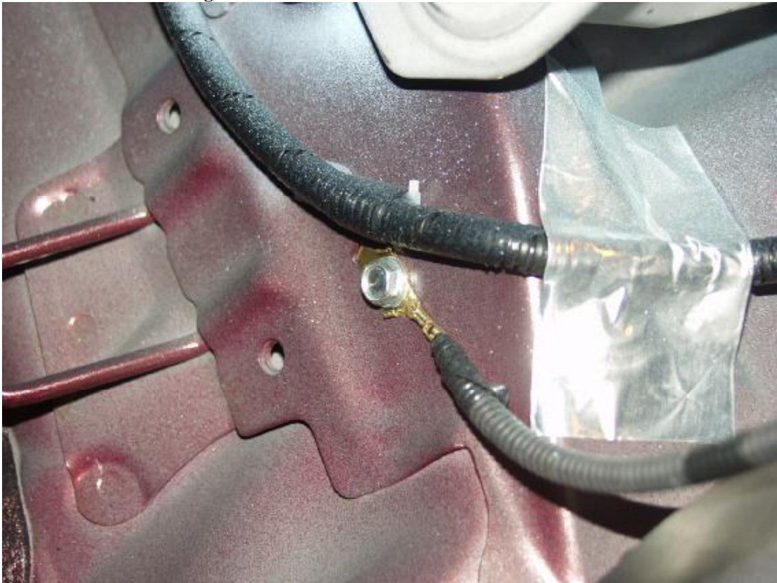
Figure A-6: Pre-Test Chassis Ground Point View
