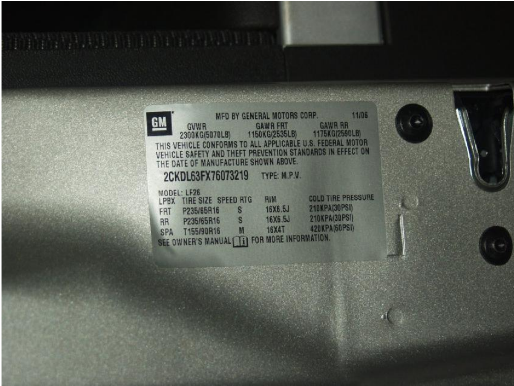
Figure A-5 : VEHICLE'S CERTIFICATION LABEL
