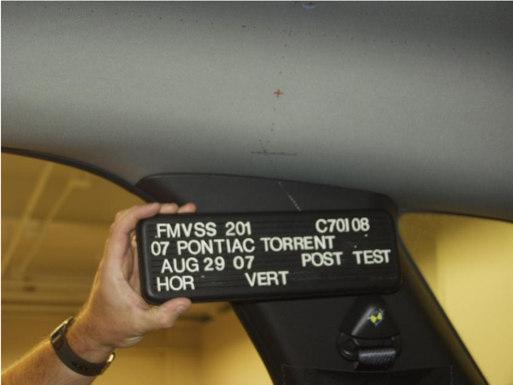
Figure A-29 : POST-TEST PASSENGER SIDE OTHER PILLAR
