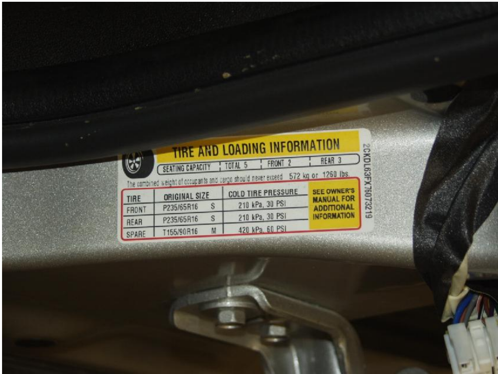
Figure A-6 : VEHICLE'S TIRE INFORMATION LABEL
