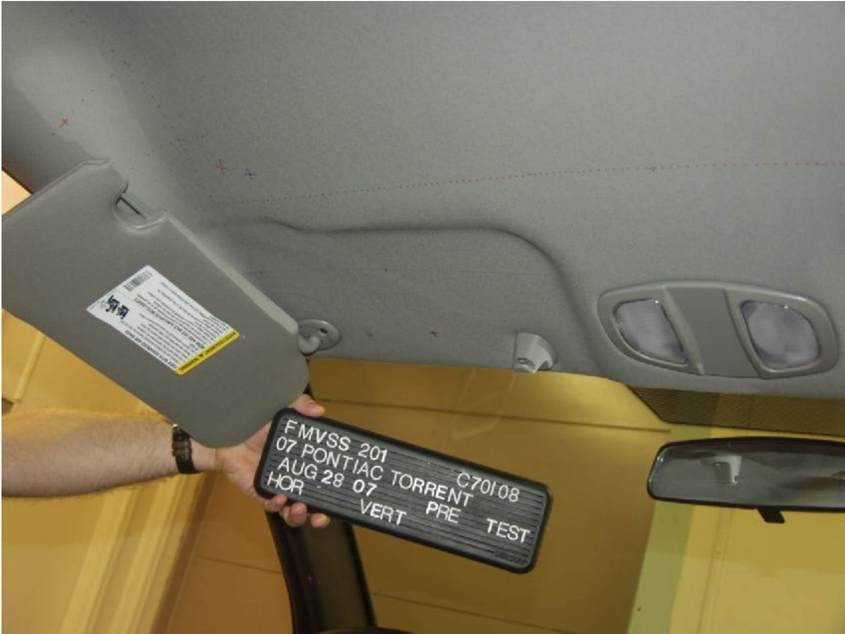
Figure A-8 : PRE-TEST DRIVER SIDE FRONT HEADER
