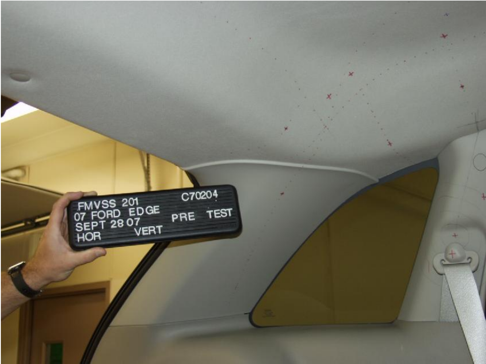
Figure A-12 : PRE-TEST DRIVER SIDE REAR PILLAR
