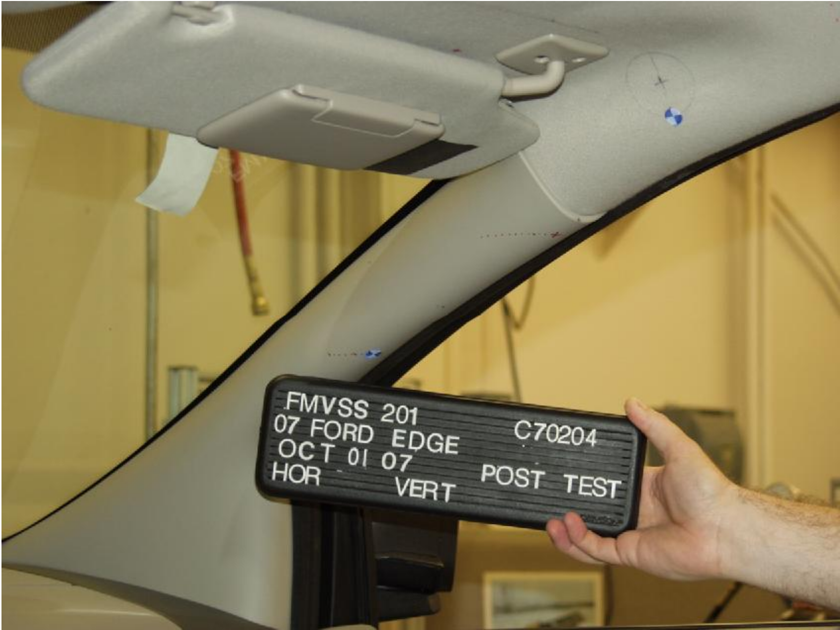
Figure A-25 : POST-TEST PASSENGER SIDE A-PILLAR
