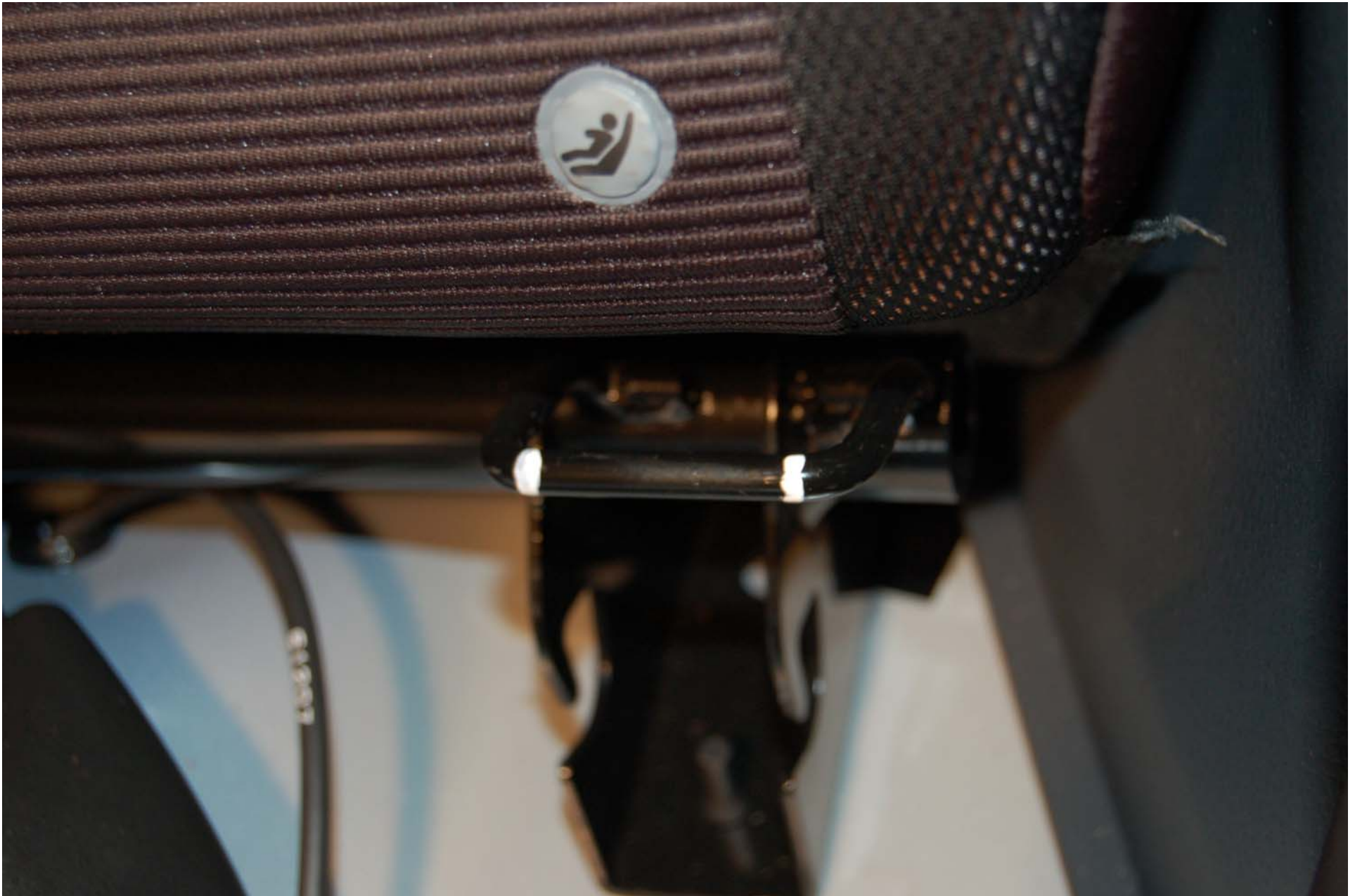
FIGURE 5.6 ROW 2, LEFT SIDE, OUTBOARD LOWER ANCHOR, PRE-TEST
