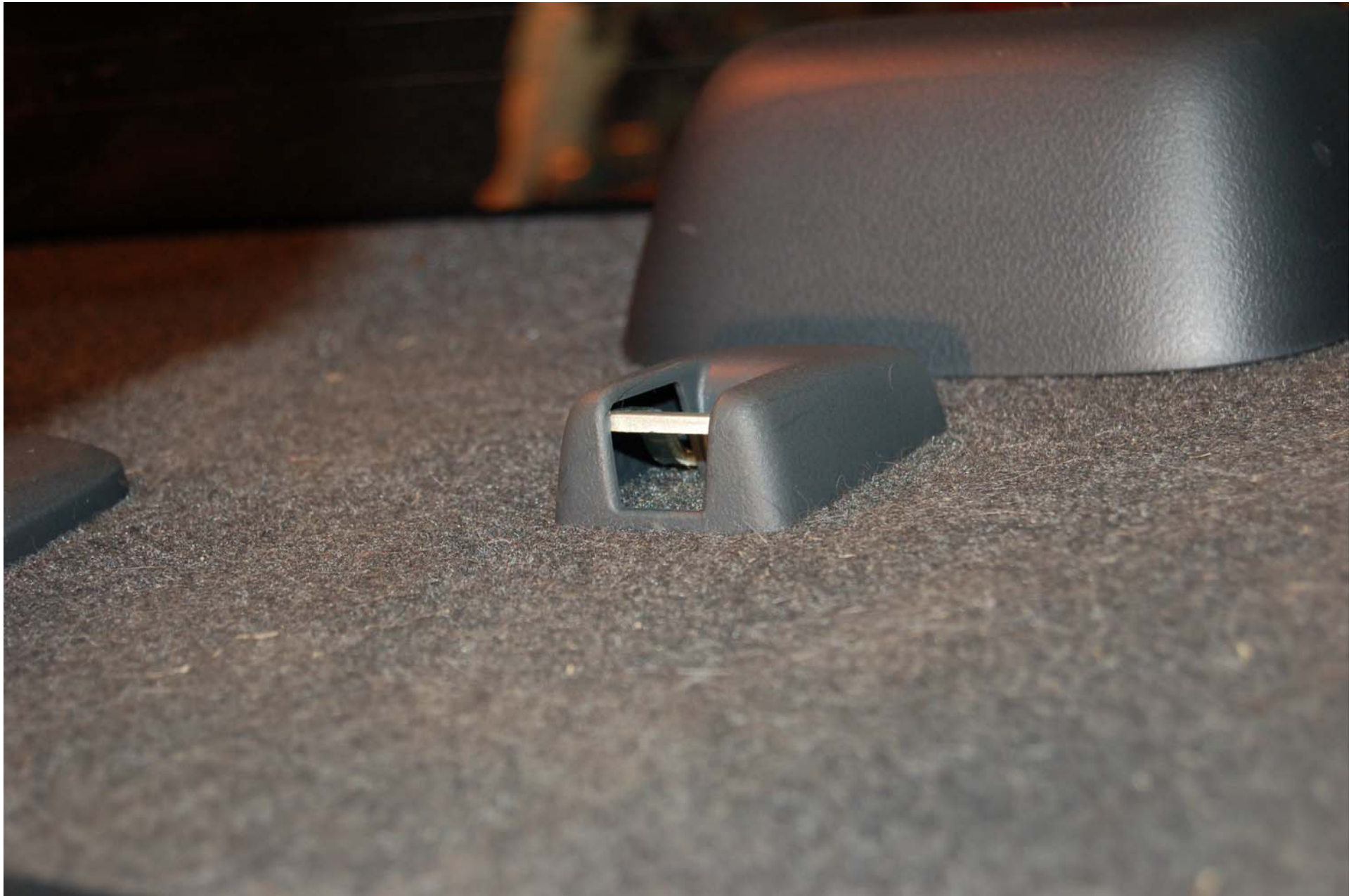
FIGURE 5.9 ROW 2, CENTER, TOP TETHER ANCHOR, PRE-TEST
