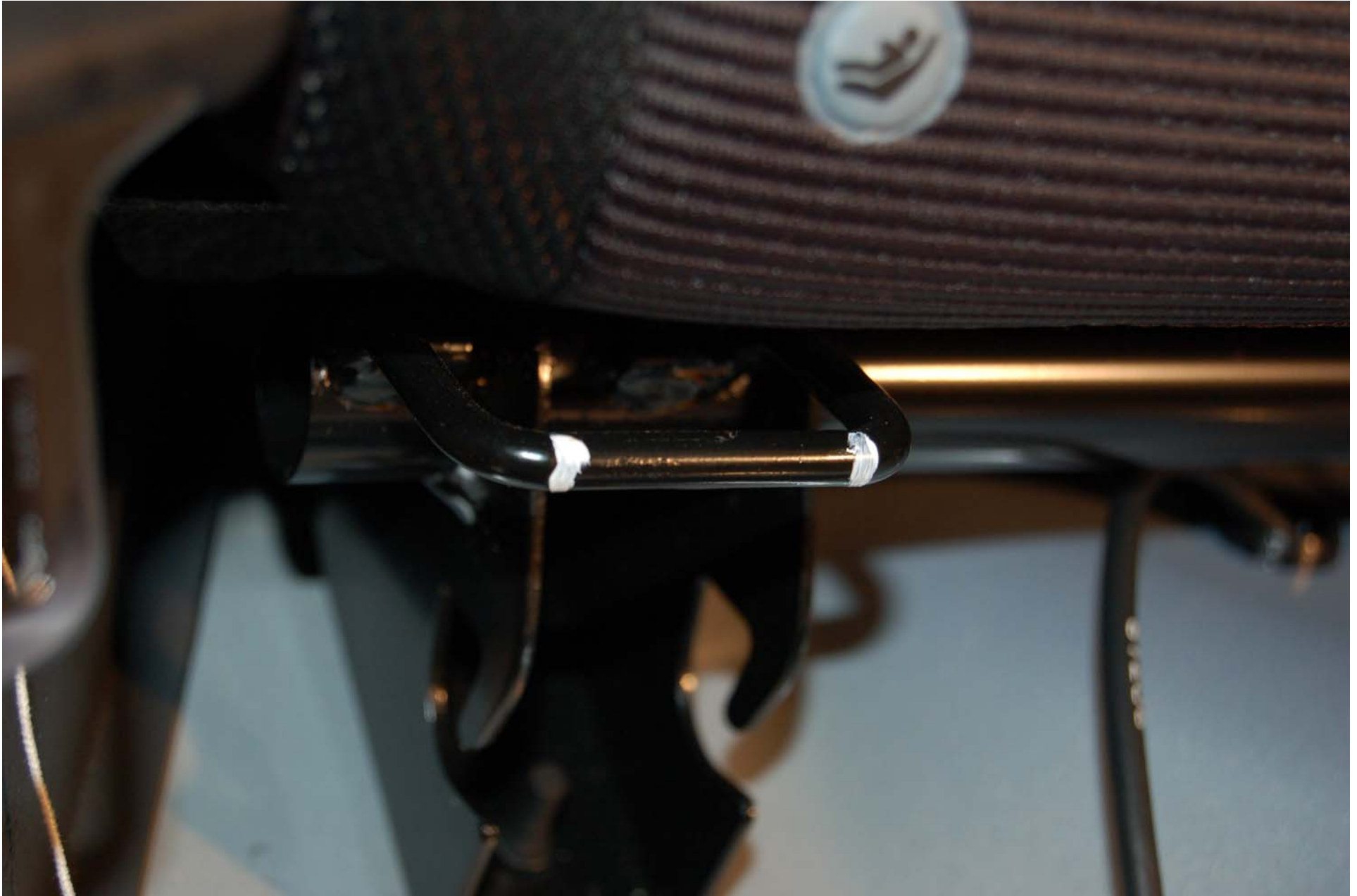
FIGURE 5.11 ROW 2, RIGHT SIDE, OUTBOARD LOWER ANCHOR, PRE-TEST
