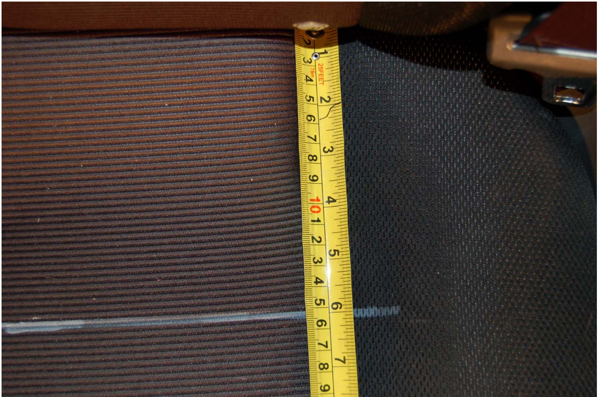
FIGURE 5.29 ROW 2, LEFT SIDE OUTBOARD SRP MEASUREMENT
