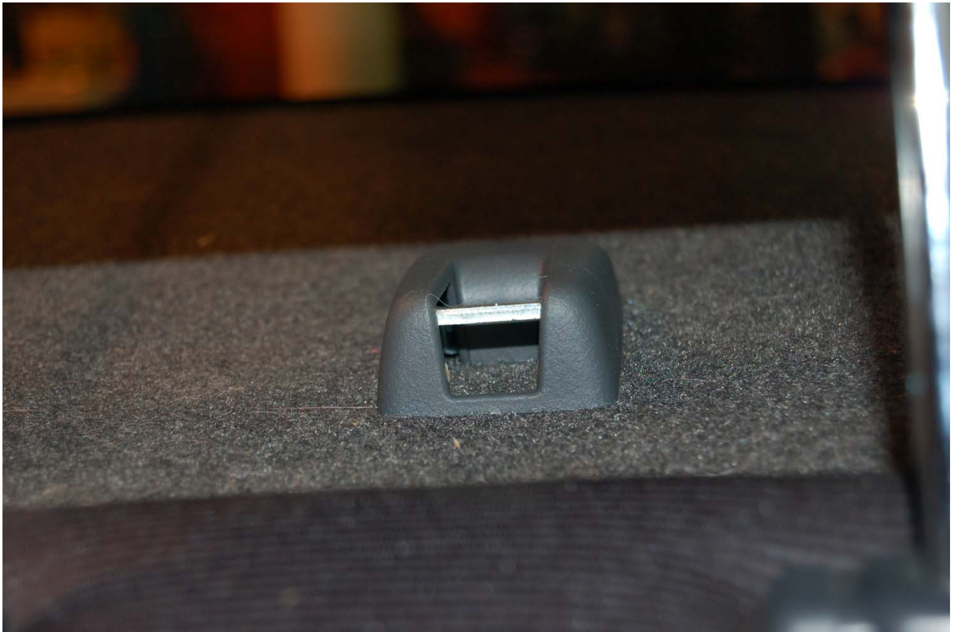
FIGURE 5.8 ROW 2, LEFT SIDE, TOP TETHER ANCHOR, PRE-TEST
