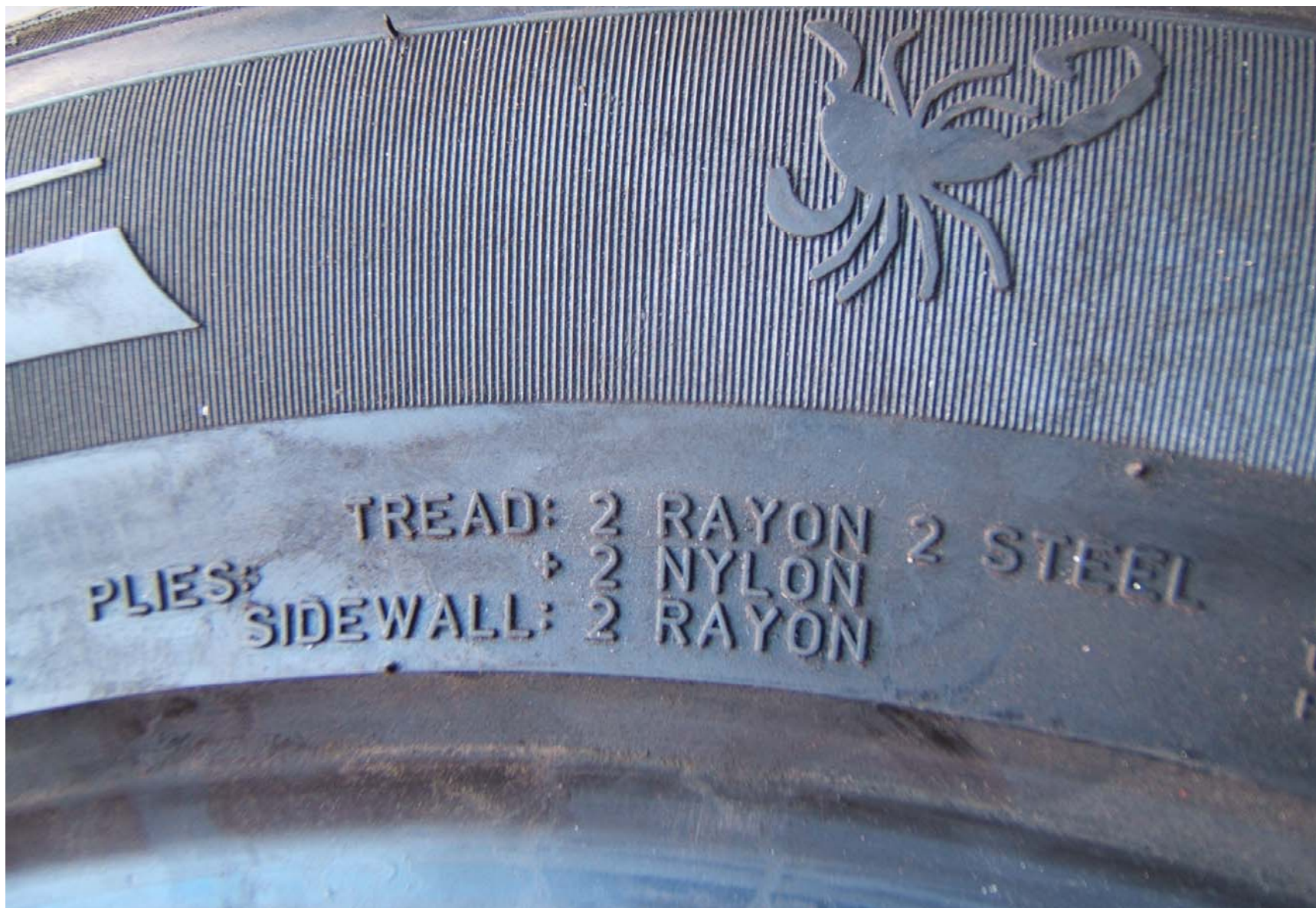
FIGURE 5.9 TIRE SHOWING SIDEWALL / TREAD CONSTRUCTION
