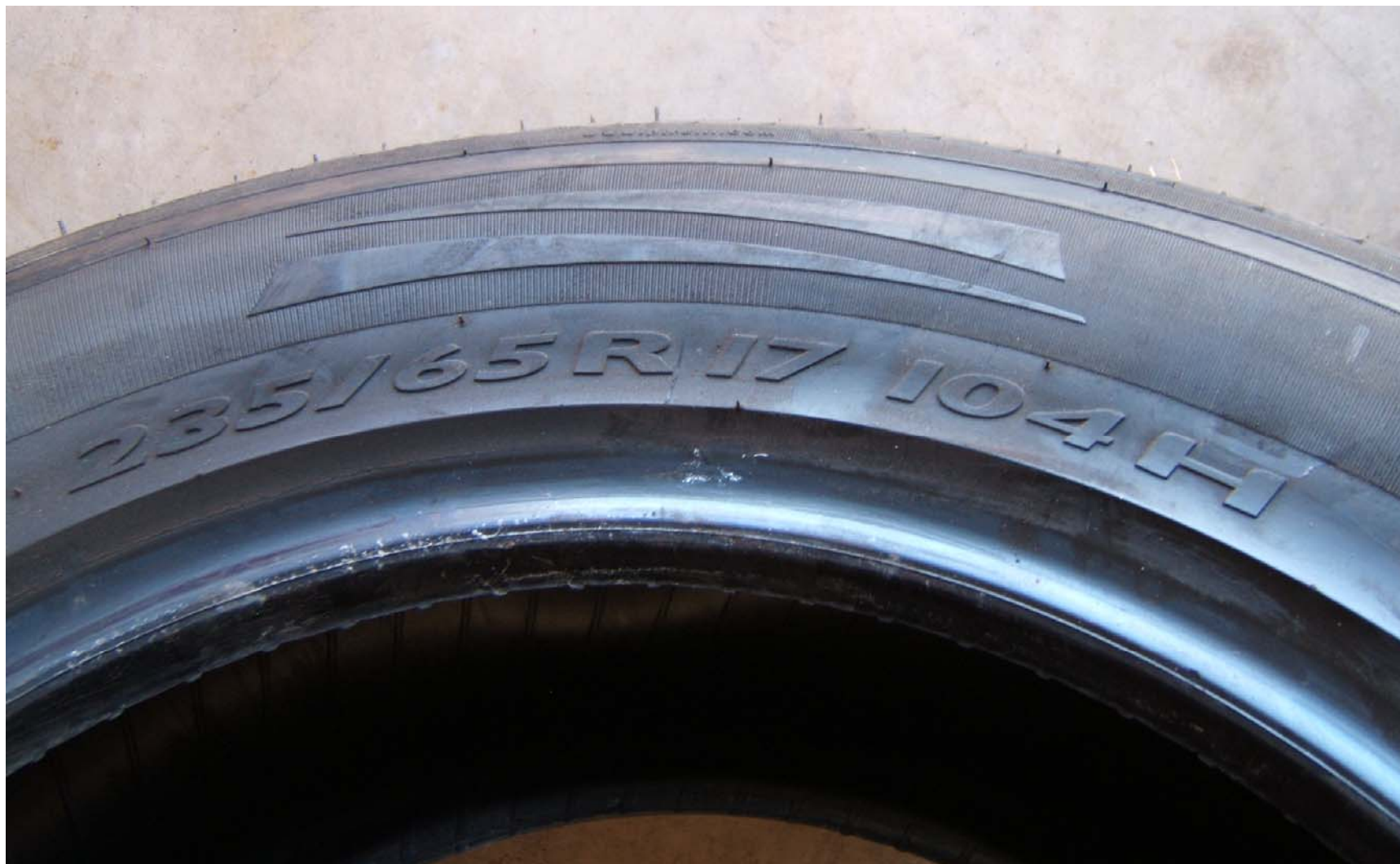
FIGURE 5.6 TIRE SHOWING SIZE, LOAD INDEX, AND SPEED RATING
