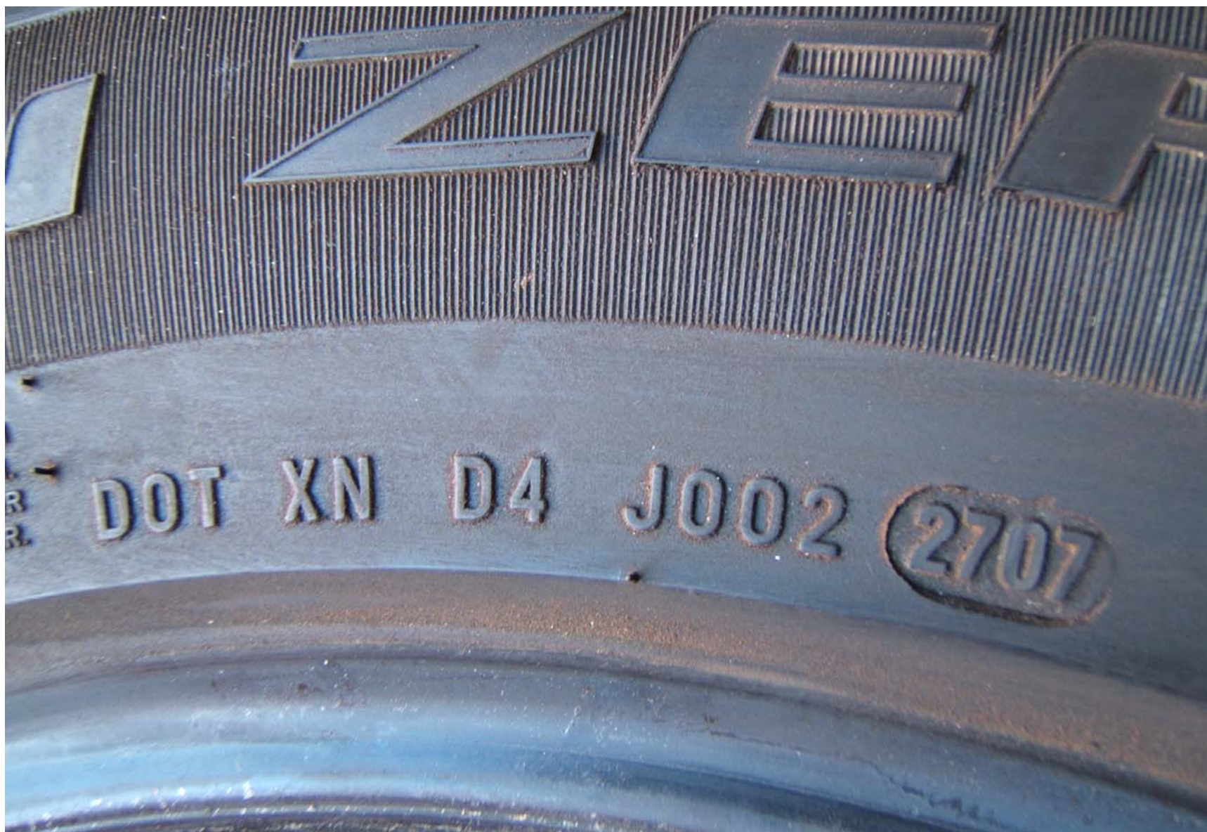
FIGURE 5.7 TIRE SHOWING DOT SERIAL NUMBER
