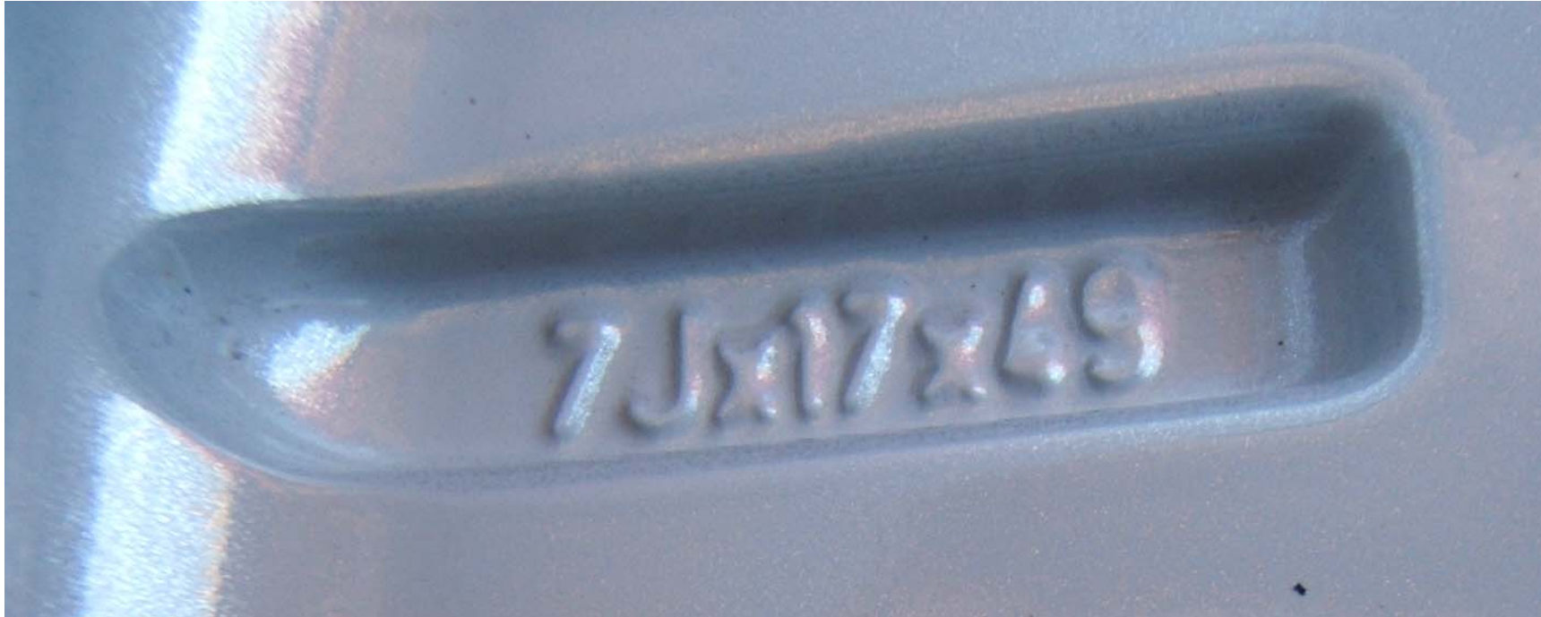
FIGURE 5.14 RIM SHOWING SIZE
