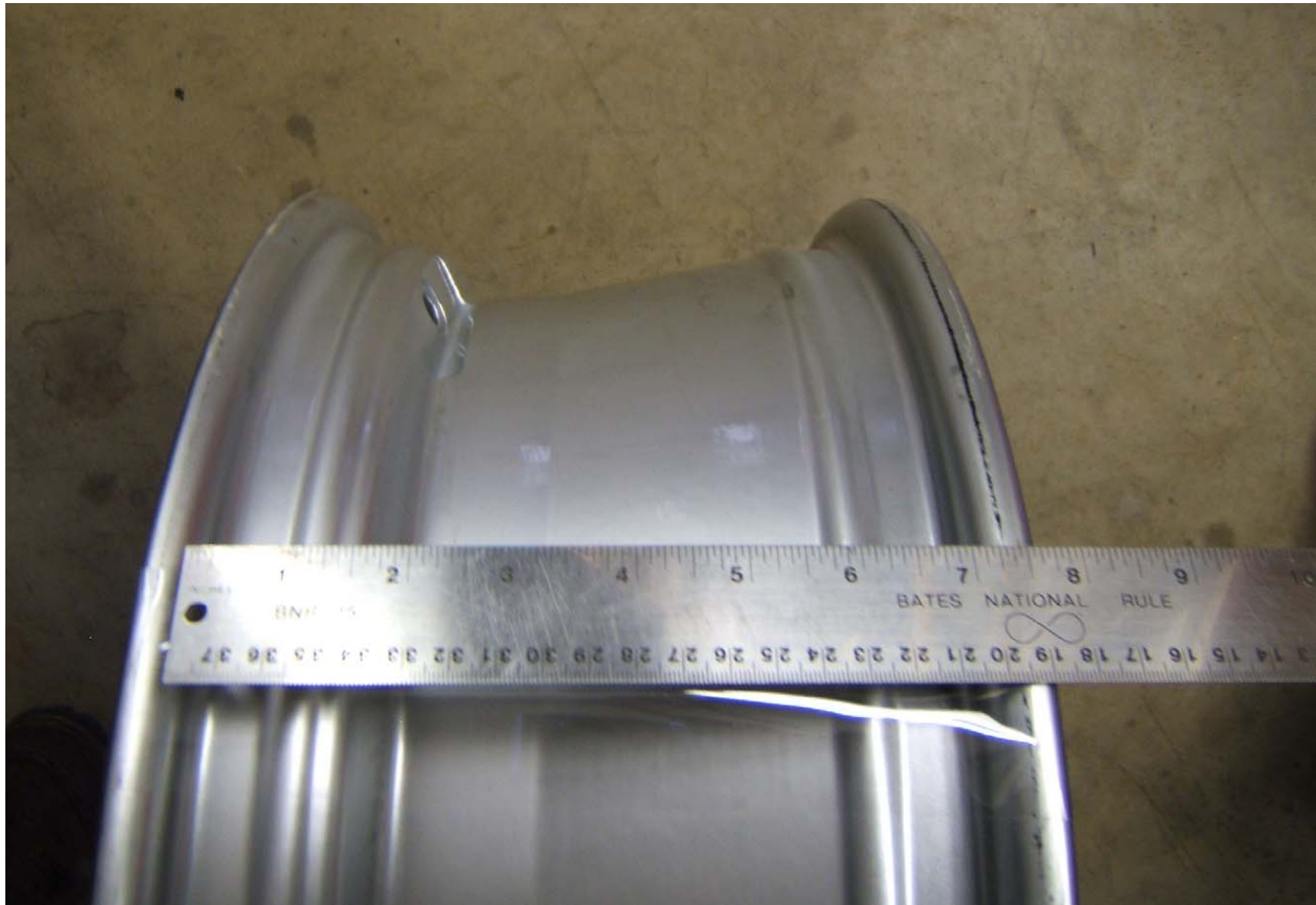
FIGURE 5.11 RIM CONTOUR FOR FULL WIDTH OF CROSS SECTION
