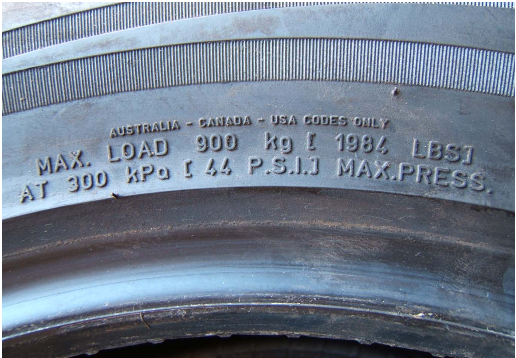
FIGURE 5.8 TIRE SHOWING MAX LOAD RATING AND MAX INFLATION PRESSURE
