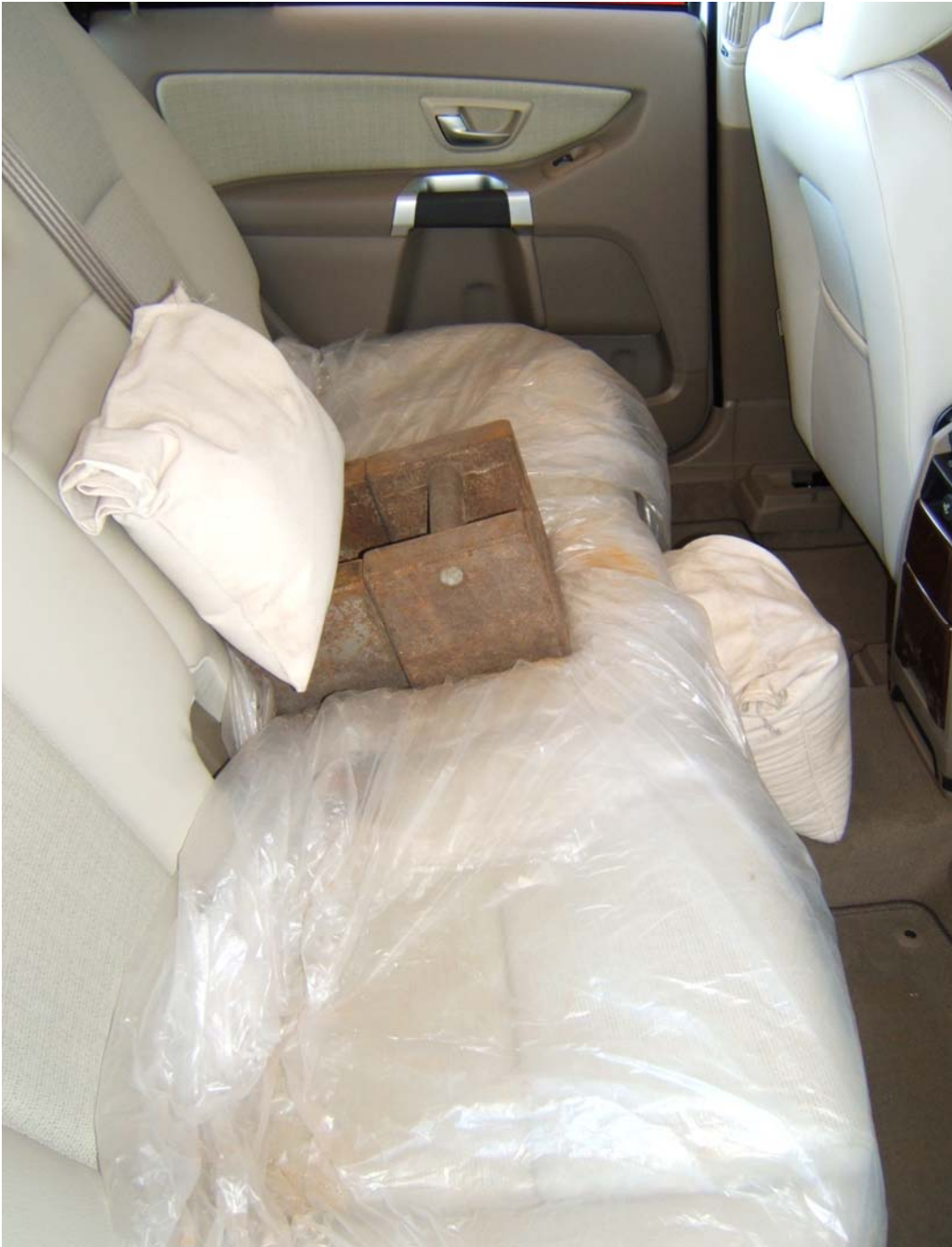
FIGURE 5.16 VEHICLE REAR SEAT BALLASTED FOR NORMAL LOAD
