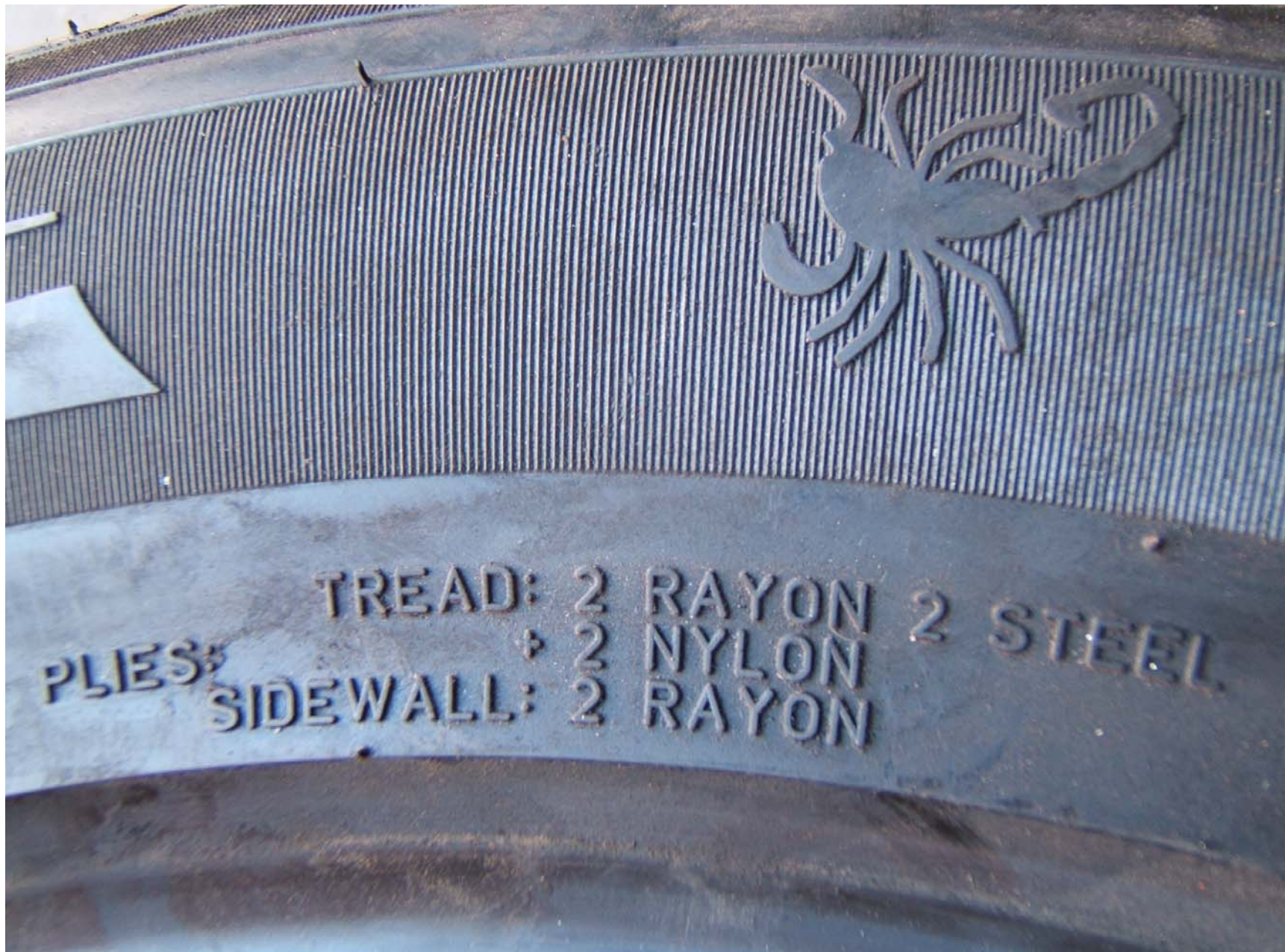
FIGURE 5.9 TIRE SHOWING CONSTRUCTION
