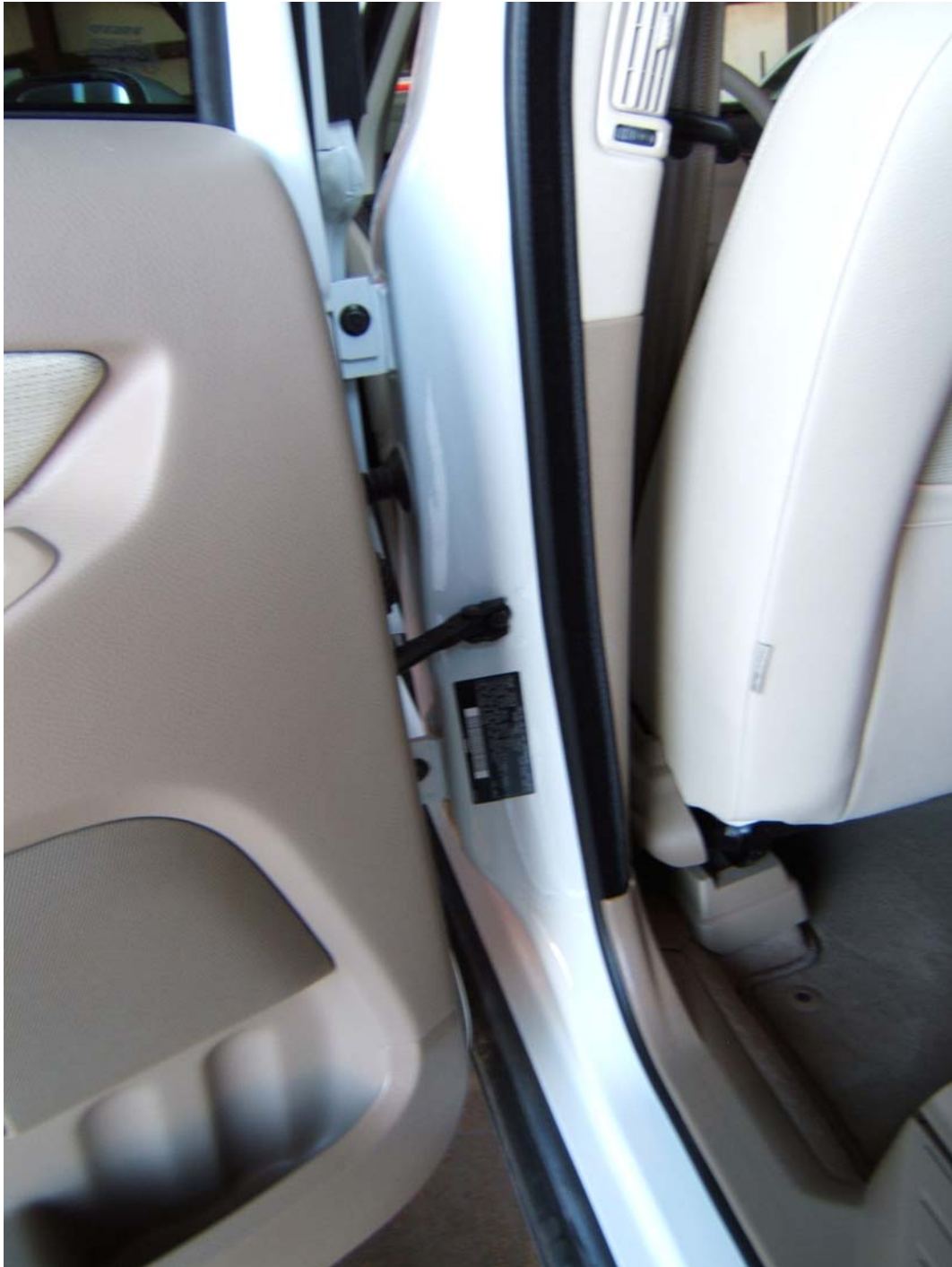
FIGURE 5.21 CERTIFICATION LABEL SHOWN ON BACK OF DRIVER'S SIDE B PILLAR
