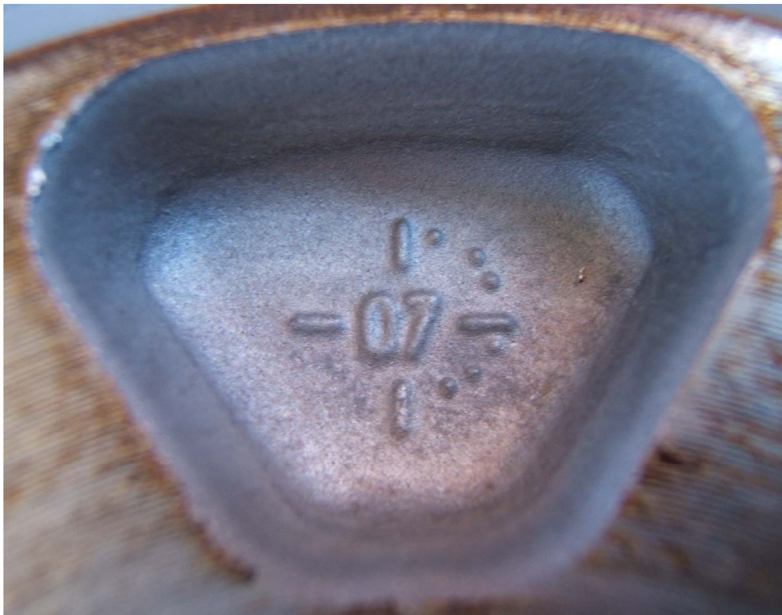
FIGURE 5.13 RIM SHOWING MANUFACTURE DATE
