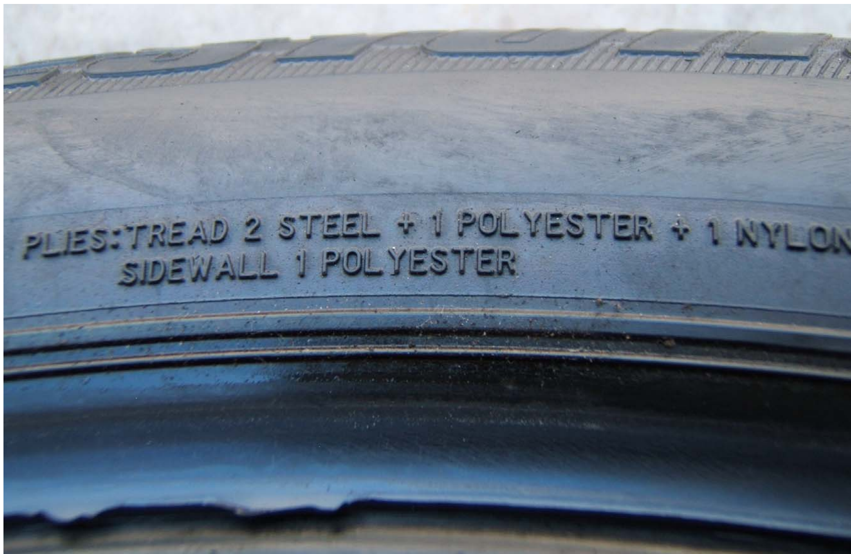
FIGURE 5.9 TIRE SHOWING SIDEWALL / TREAD CONSTRUCTION
