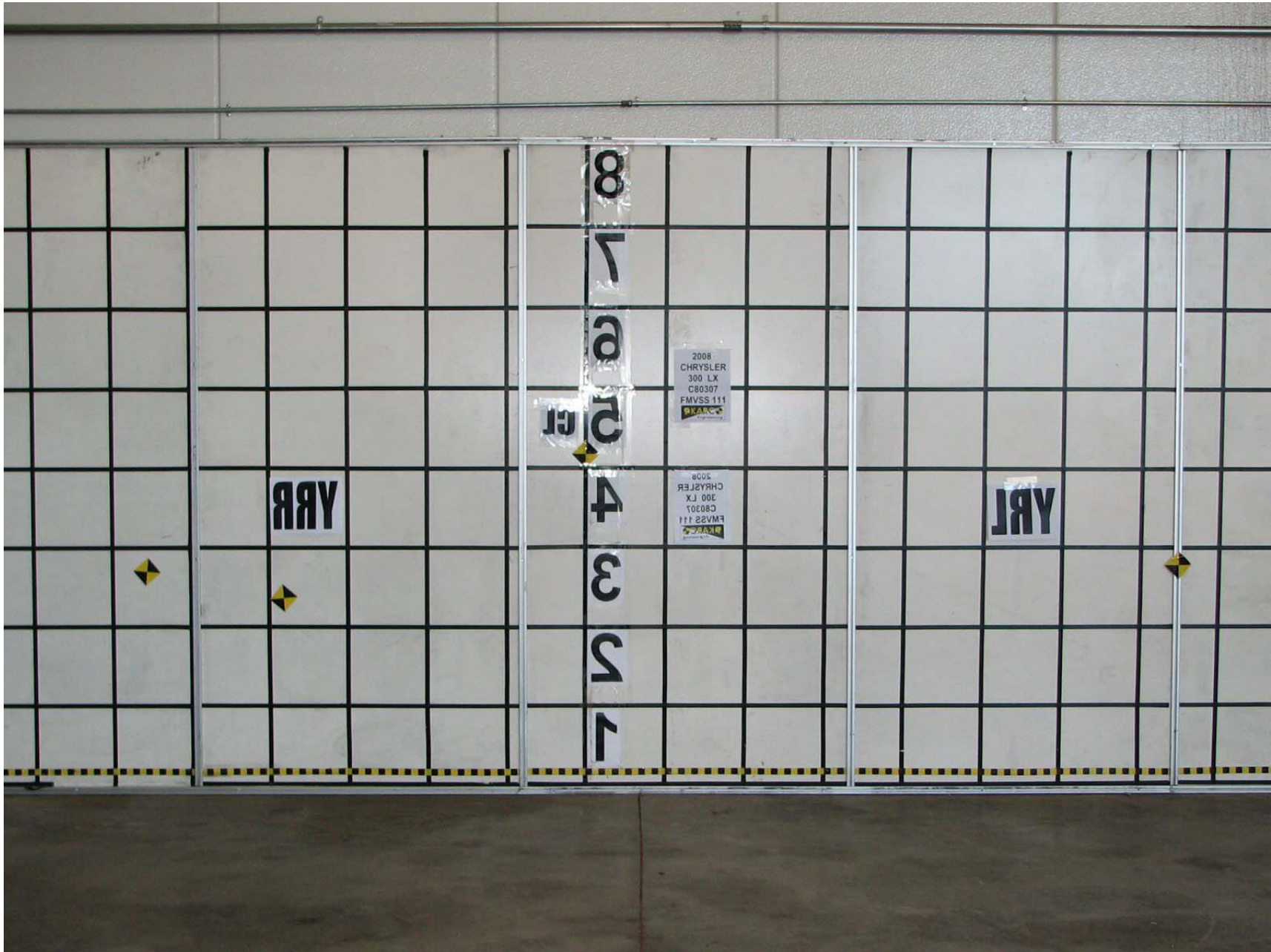
FIGURE 19:REFERENCE BOARD FOR INSIDE MIRROR, RIGHT EYE
