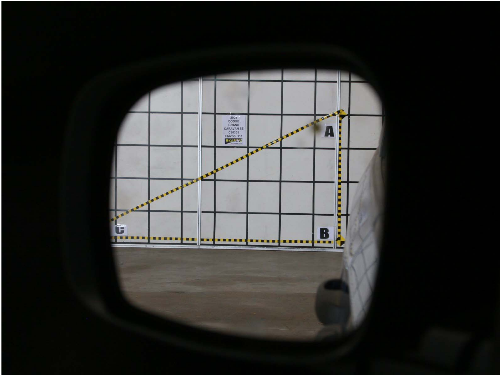
2008 DODGE GRAND CARAVAN SE NHTSA NO. C80305 FMVSS NO. 111 FIGURE 20:LEFT EYE FIELD OF VIEW TEST (DRIVER SIDE MIRROR)
