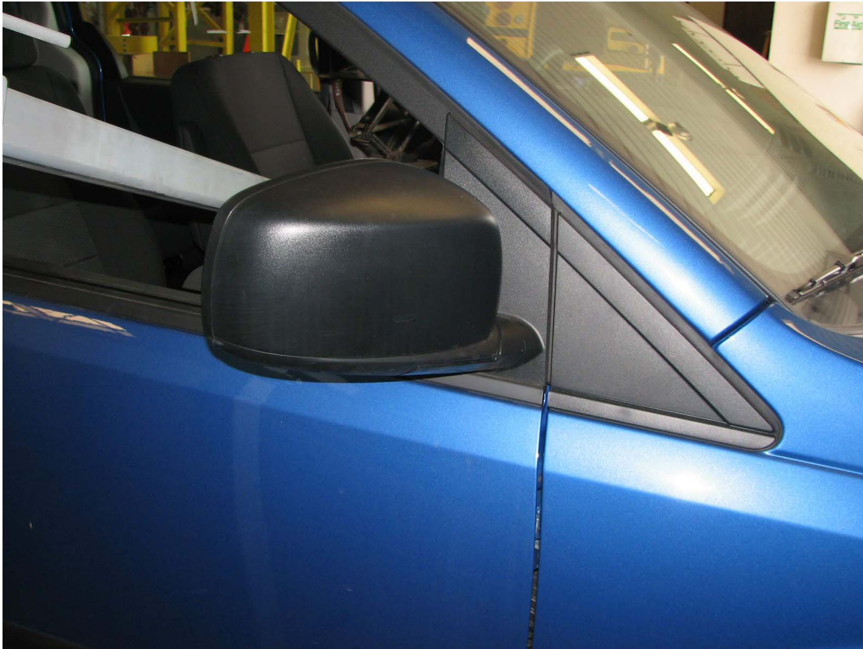
2008 DODGE GRAND CARAVAN SE FIGURE 8: PASSENGER SIDE REARVIEW MIRROR AND MOUNTING NHTSA NO. C80305 FMVSS NO. 111
