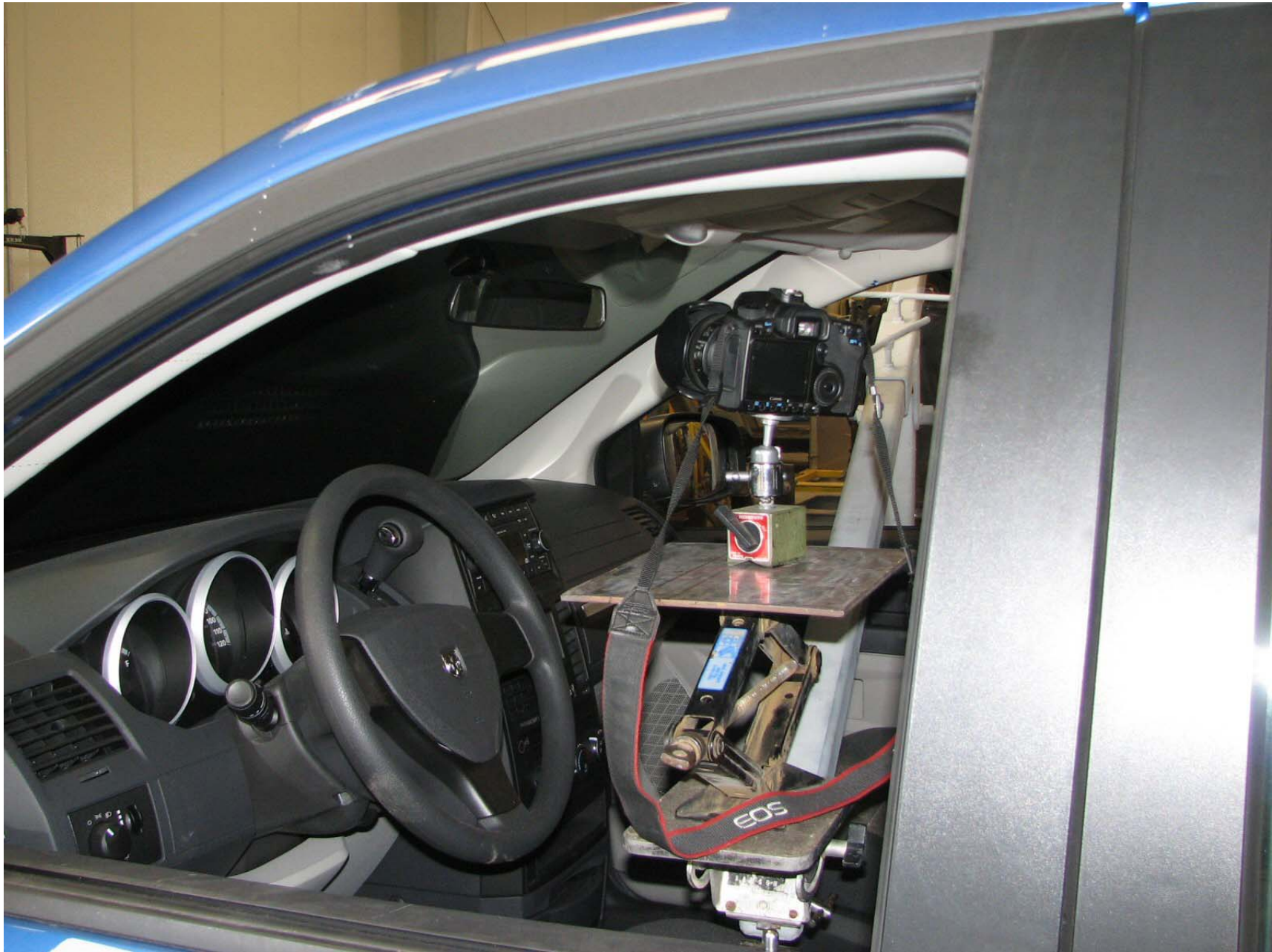
2008 DODGE GRAND CARAVAN SEFIGURE 11:CAMERA SET-UP FOR PHOTOGRAPHING REFERENCE BOARD NHTSA NO. C80305 FMVSS NO. 111
