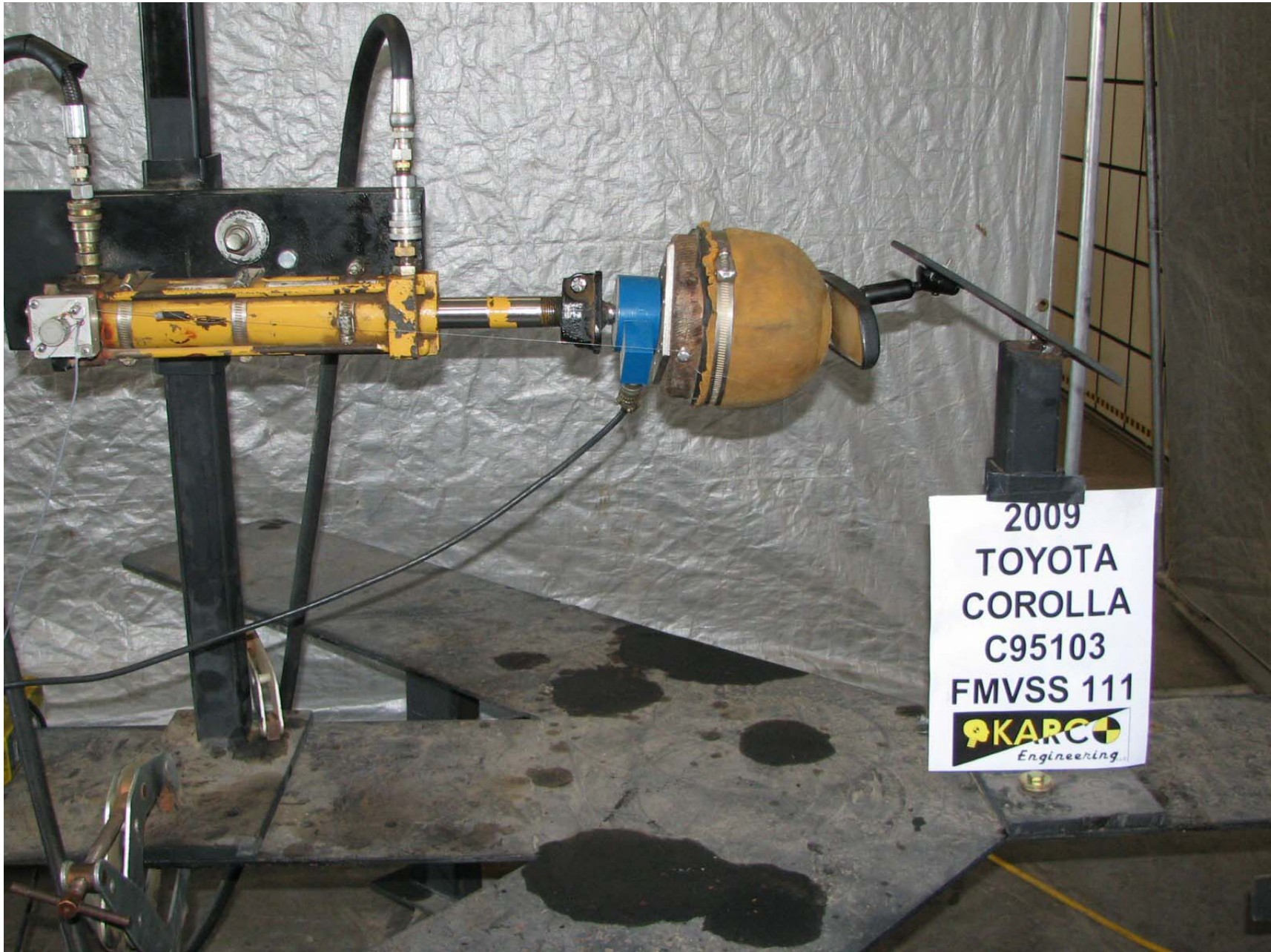
2009 TOYOTA COROLLA LE FIGURE 12: OVERALL SET-UP AND INSTRUMENTATION FOR MIRROR BREAK- AWAY TEST NHTSA NO. C95103 FMVSS NO. 111
