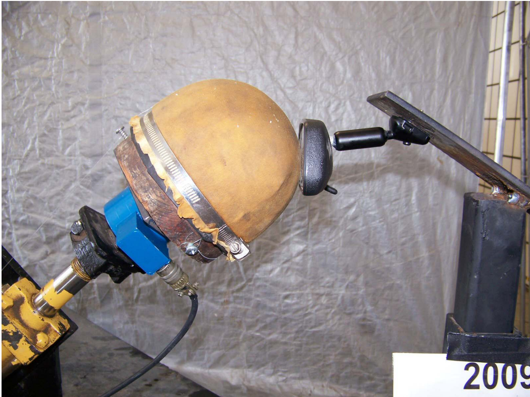
FIGURE 13:CLOSE-UP OF MIRROR BREAK- AWAY TEST
