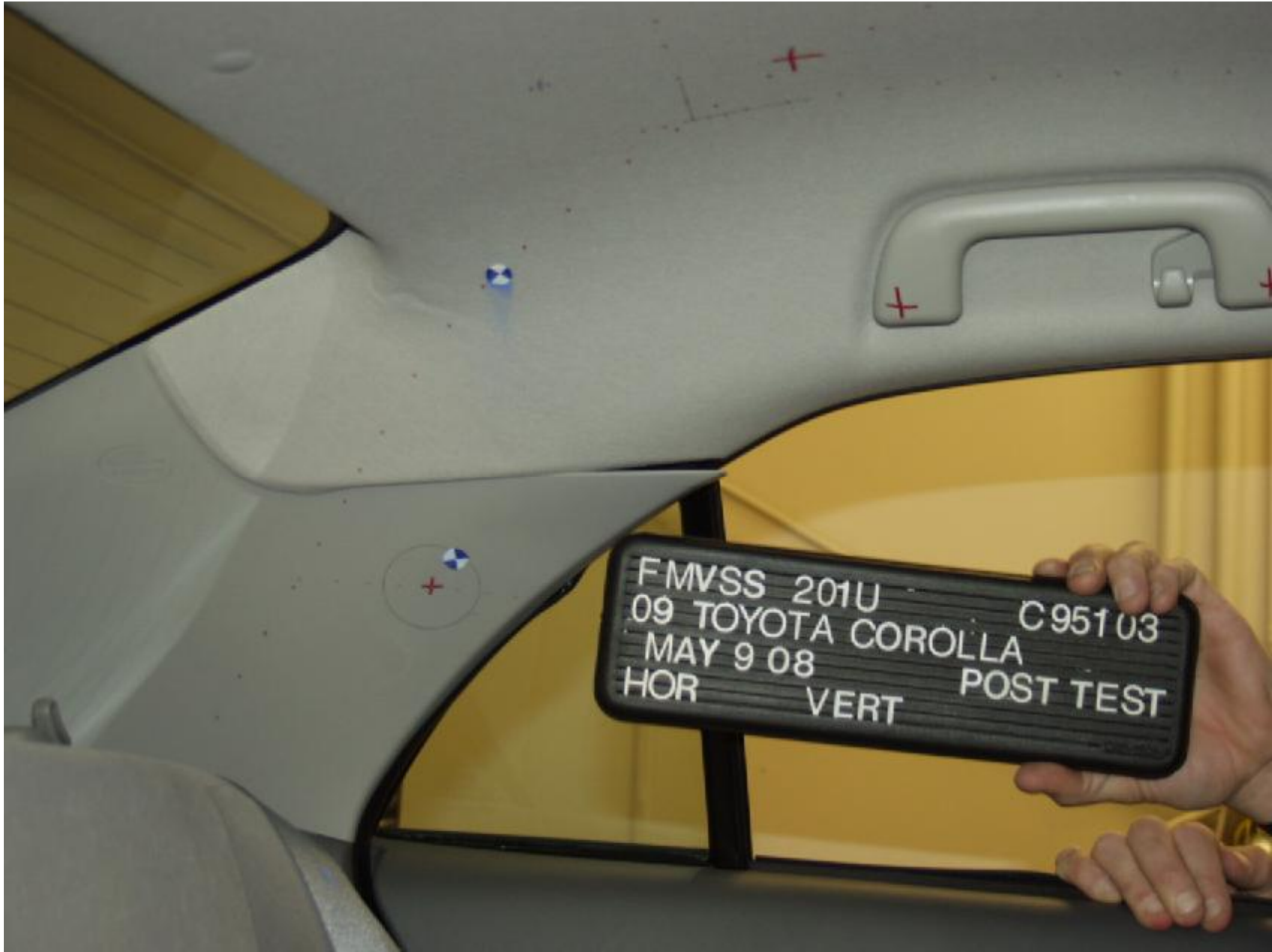
Figure A-21 : POST-TEST DRIVER SIDE REAR PILLAR
