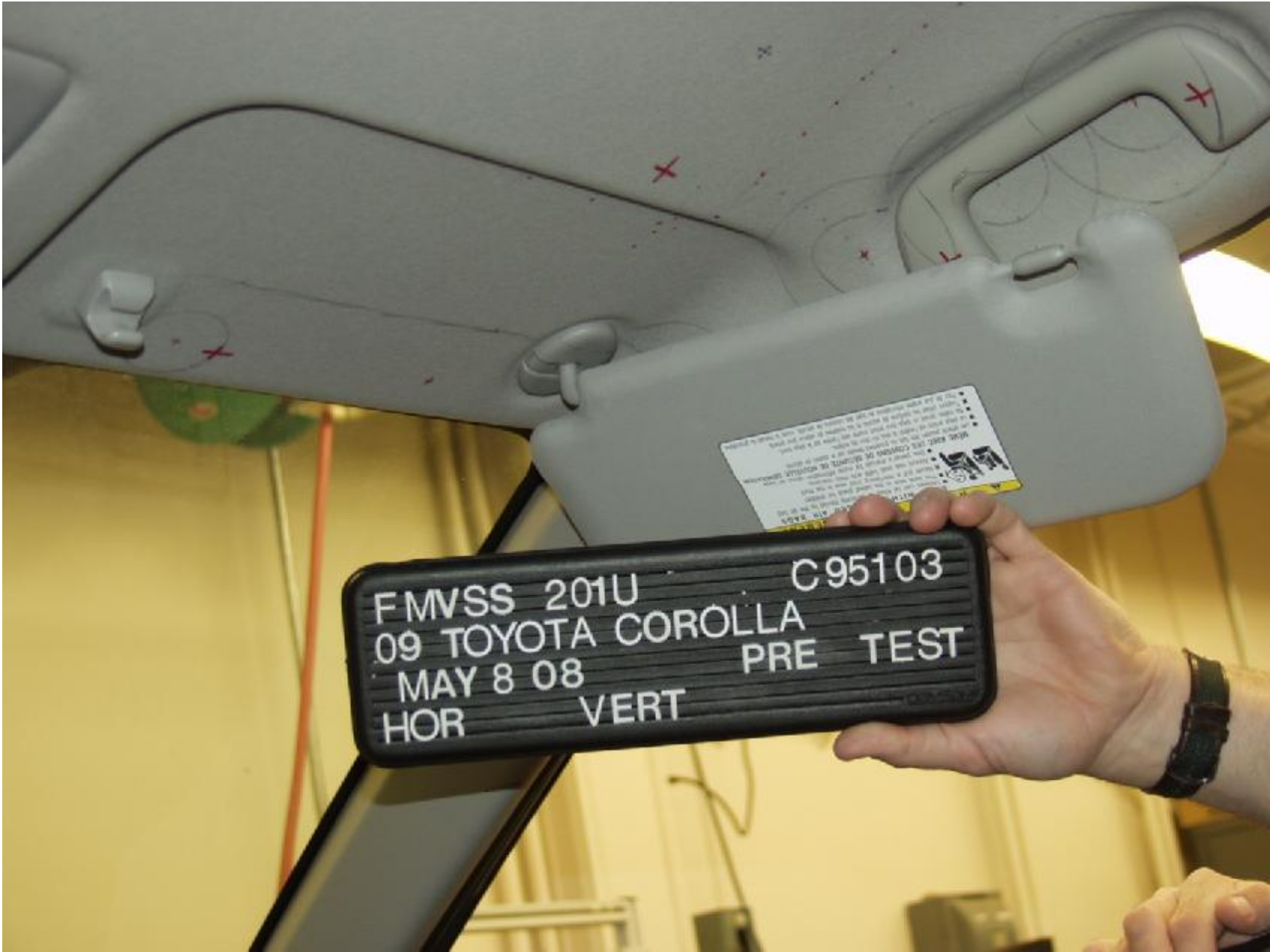
Figure A-13 : PRE-TEST PASSENGER SIDE FRONT HEADER
