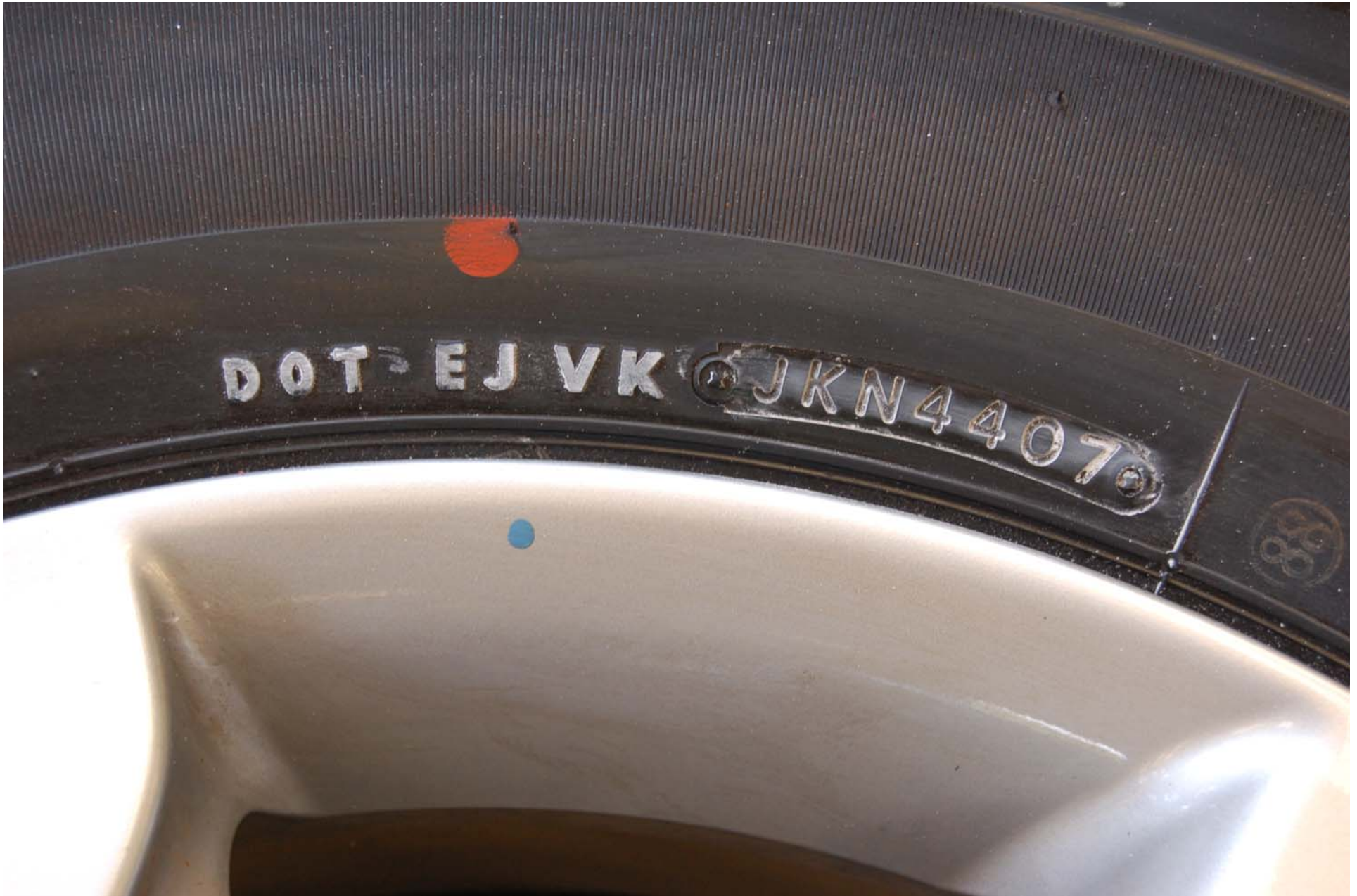
FIGURE 5.8 TIRE SHOWING SERIAL NUMBER
