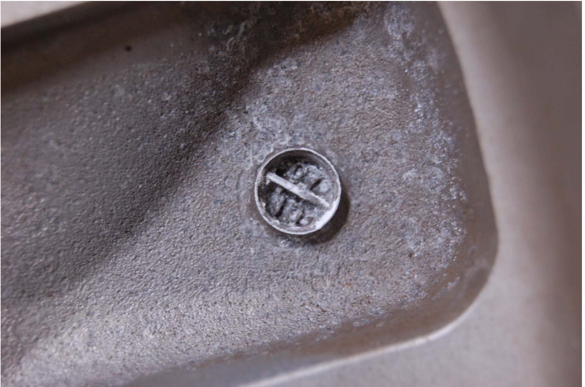
FIGURE 5.11 RIM MARKING SHOWING DATE CODE
