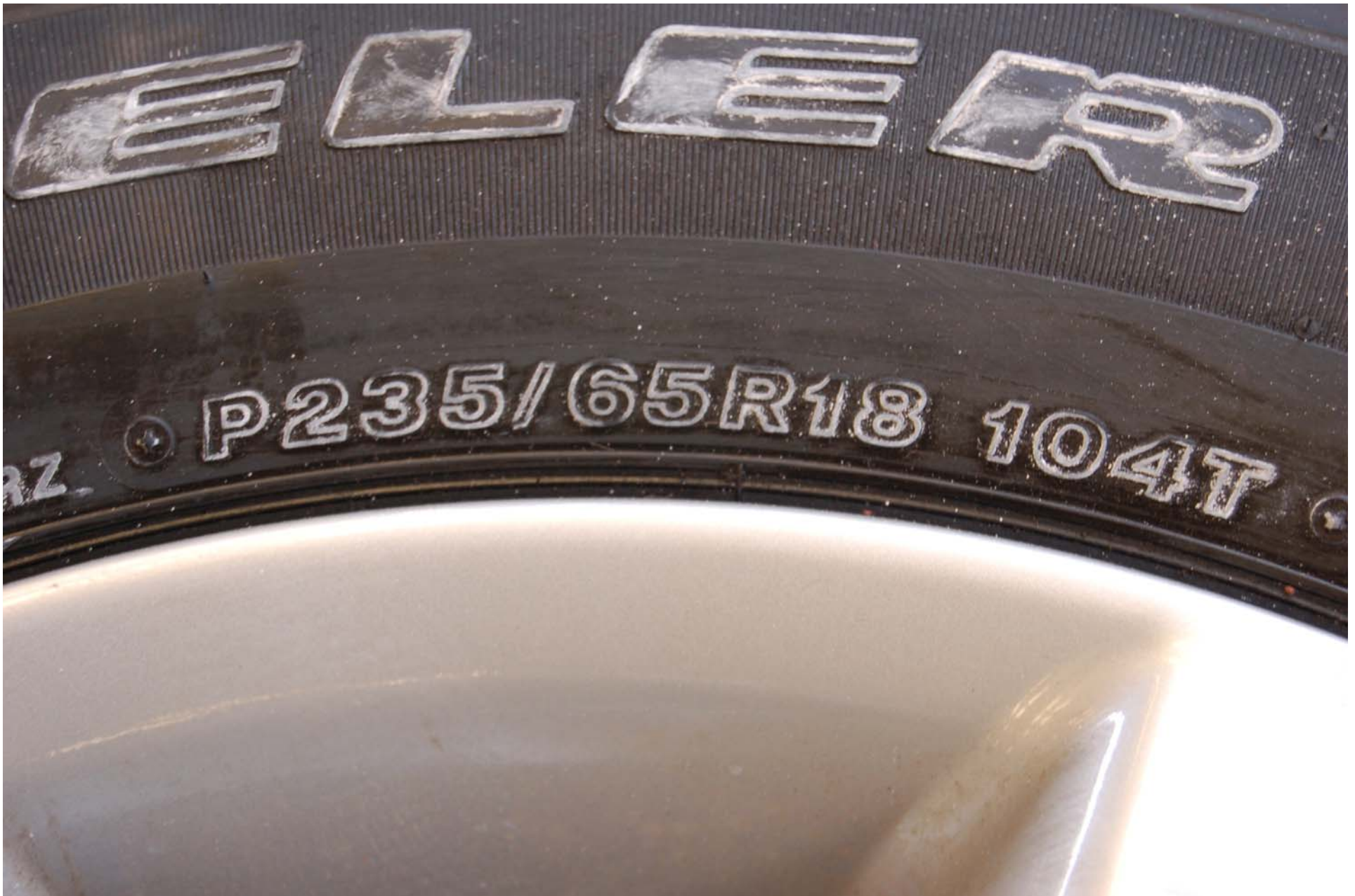
FIGURE 5.6 TIRE SHOWING SIZE, LOAD INDEX AND SPEED SYMBOL
