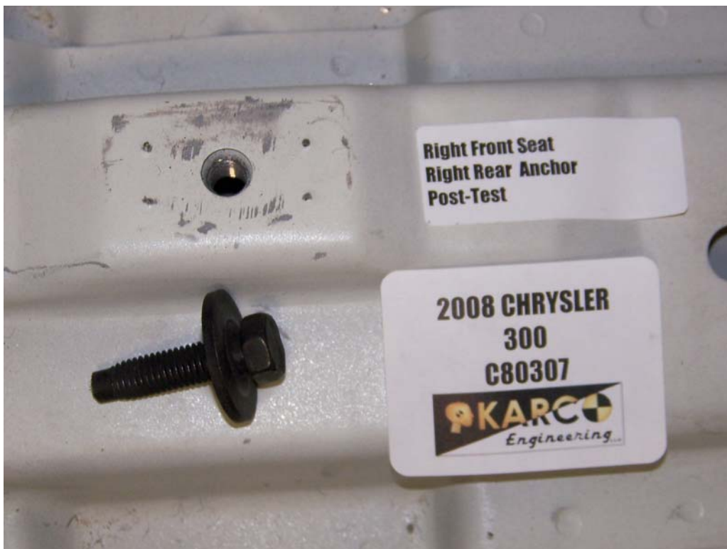
FIGURE 76. Floor Pan Anchor, P2, Post-Test
