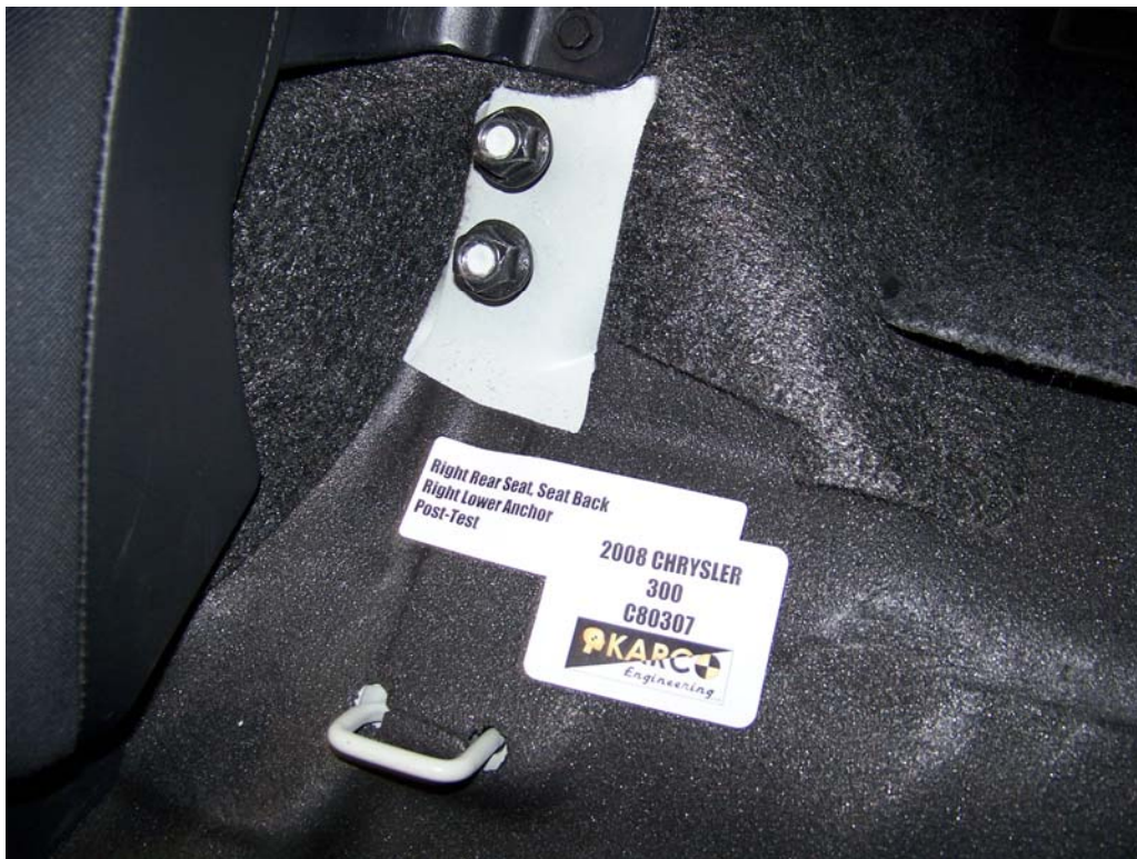
FIGURE 114. Floor Pan Anchor, P3, Post-Test
