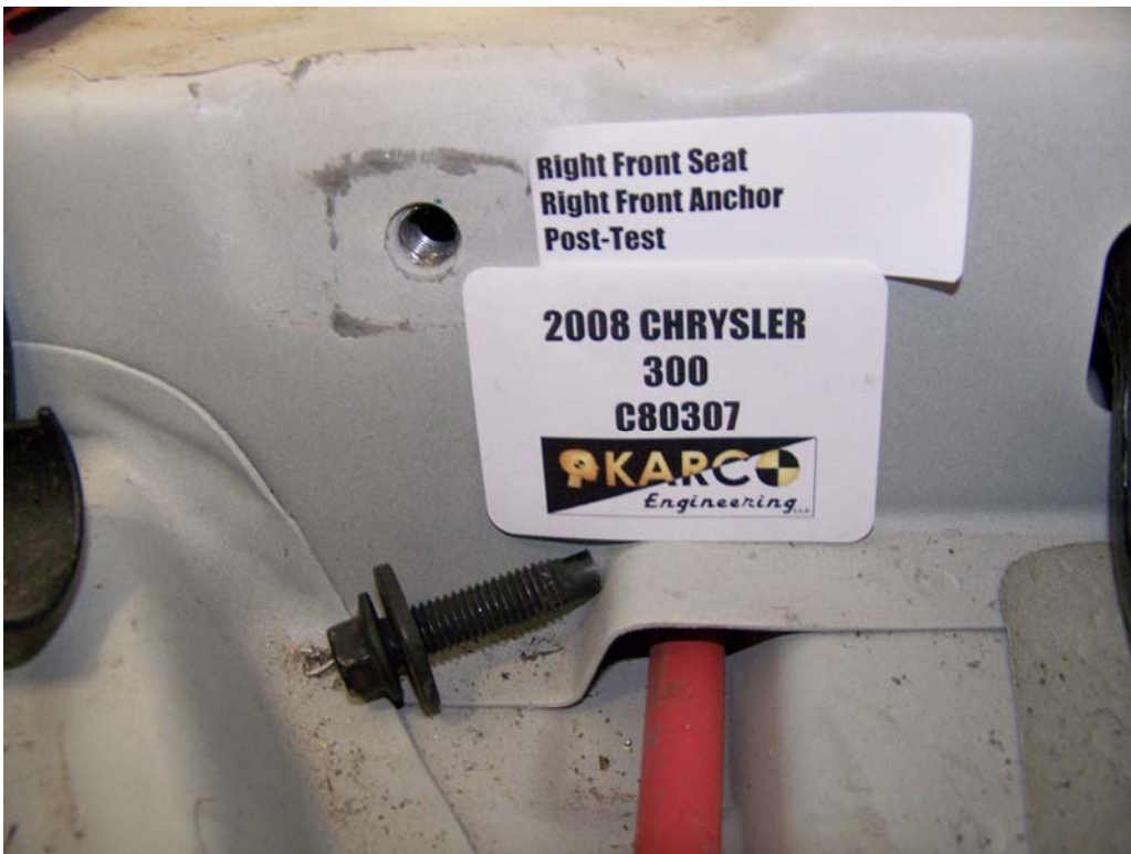
FIGURE 72. Floor Pan Anchor, P2, Post-Test
