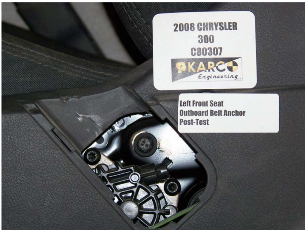
FIGURE 60. Belt Anchor, P1, Post-Test
