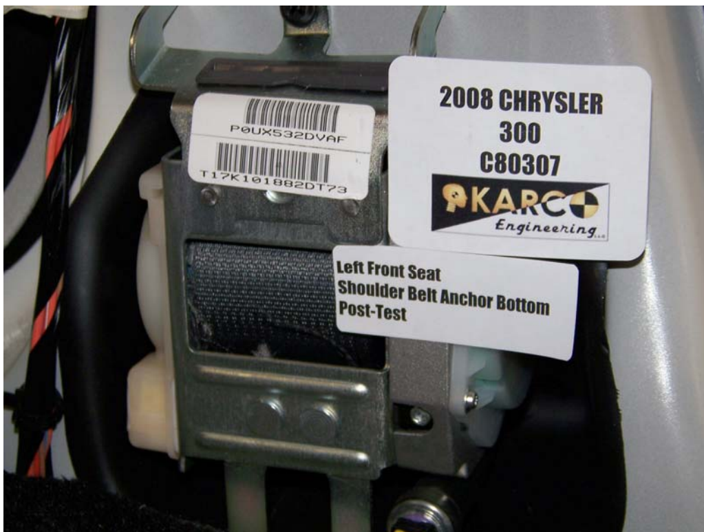
FIGURE 58. Shoulder Belt Anchor, P1, Post-Test
