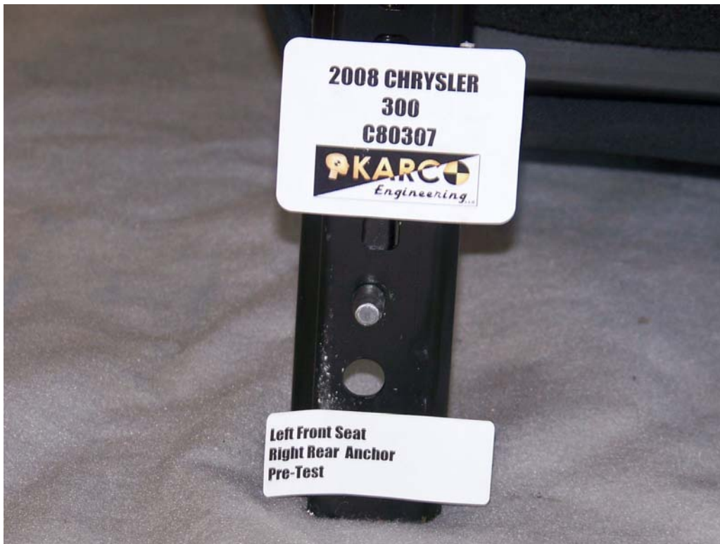
FIGURE 49. Seat Anchor, P1, Pre-Test
