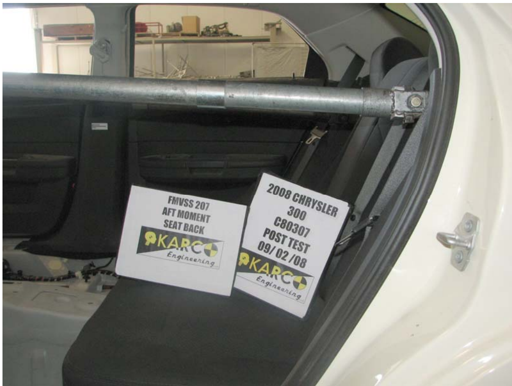
FIGURE 28. Aft Moment Seat Back, P4, Post-Test
