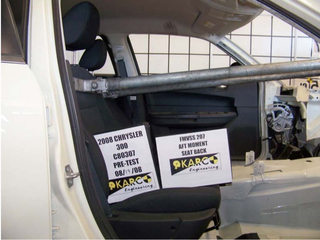
FIGURE 13. Aft Moment on Seat Back, P2, Pre-Test
