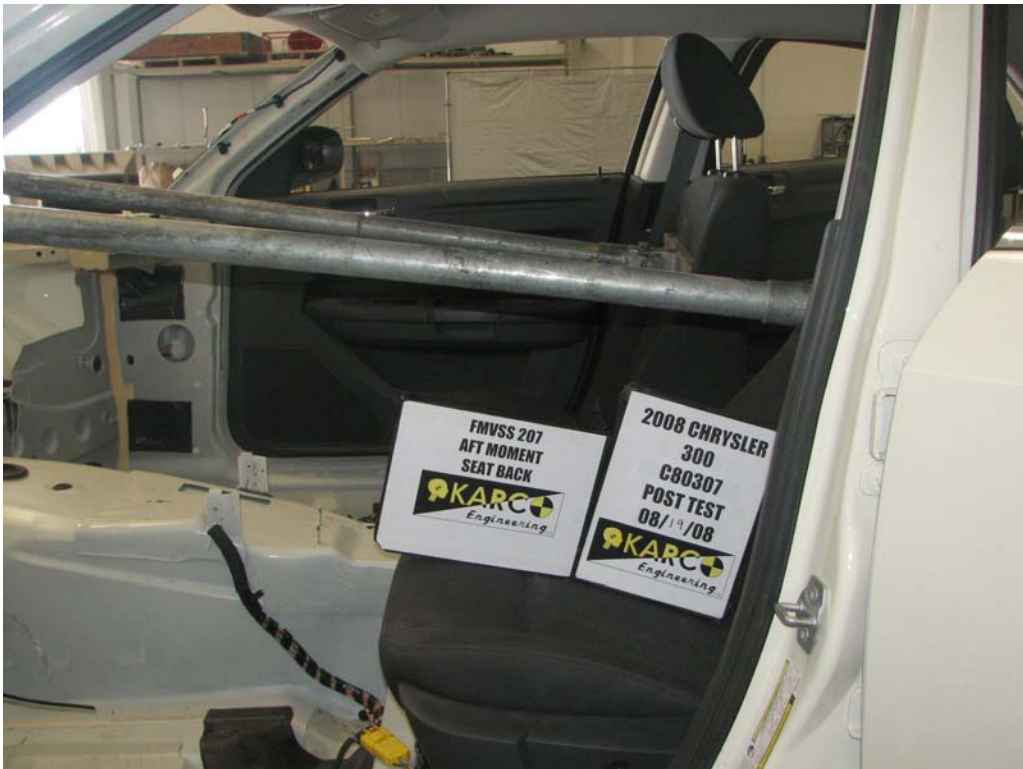
FIGURE 12. Aft Moment on Seat Back, P1, Post-Test
