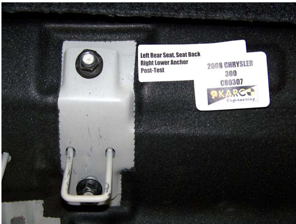
FIGURE 104. Floor Pan Anchor, P4, Post-Test
