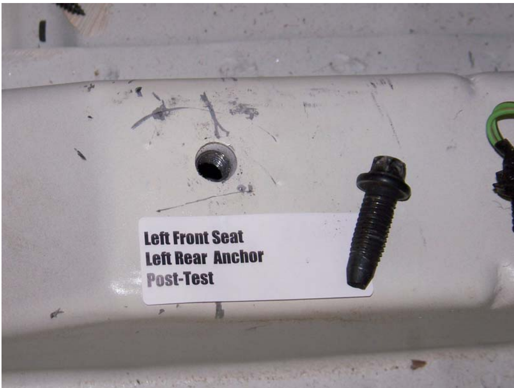
FIGURE 52. Floor Pan Anchor, P1, Post-Test
