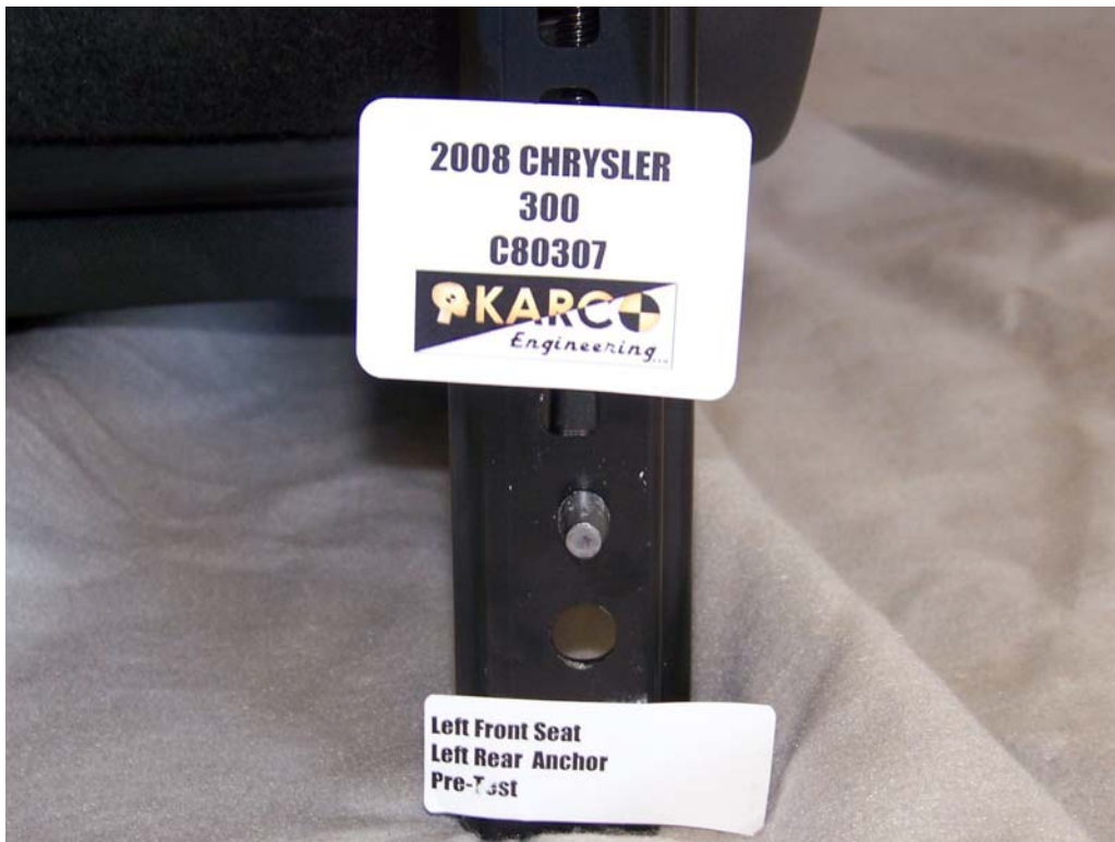
FIGURE 53. Seat Anchor, P1, Pre-Test
