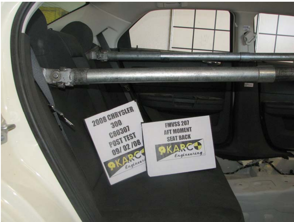
FIGURE 30. Aft Moment on Seat Back, P3, Post-Test
