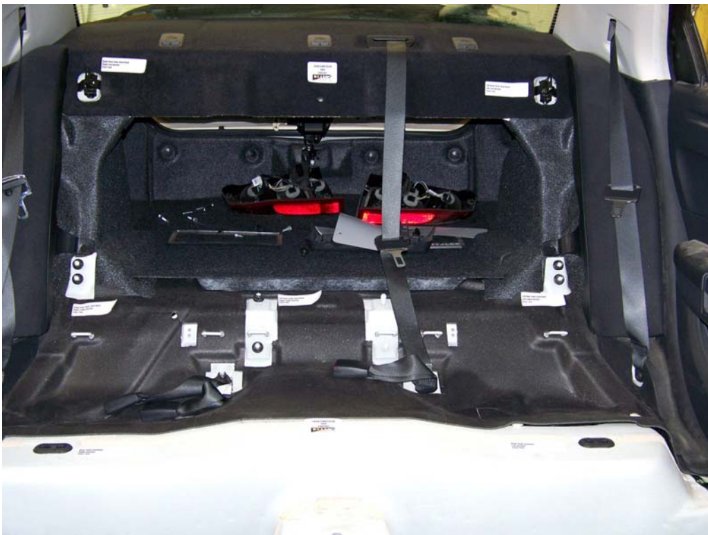
FIGURE 92. Floor Pan Anchors, P3 & P4, Post-Test
