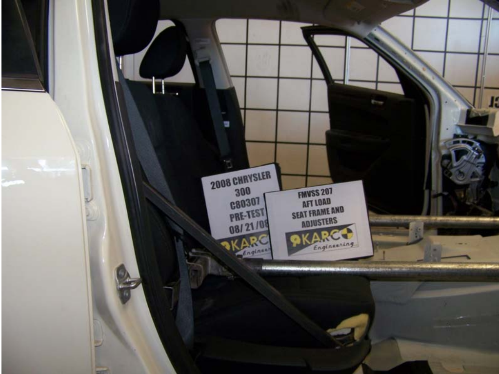
FIGURE 21. Aft Load on Seat Frame and Adjusters, P2, Pre-Test
