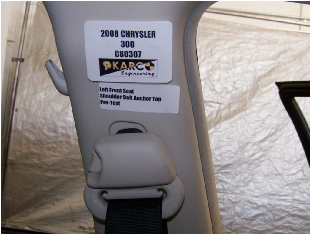
FIGURE 55. Shoulder Belt Anchor, P1, Pre-Test
