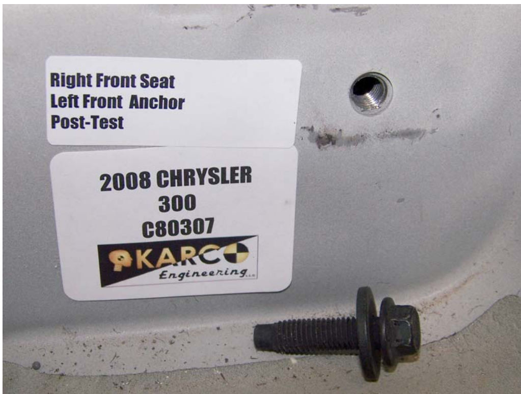
FIGURE 68. Floor Pan Anchor, P2, Post-Test
