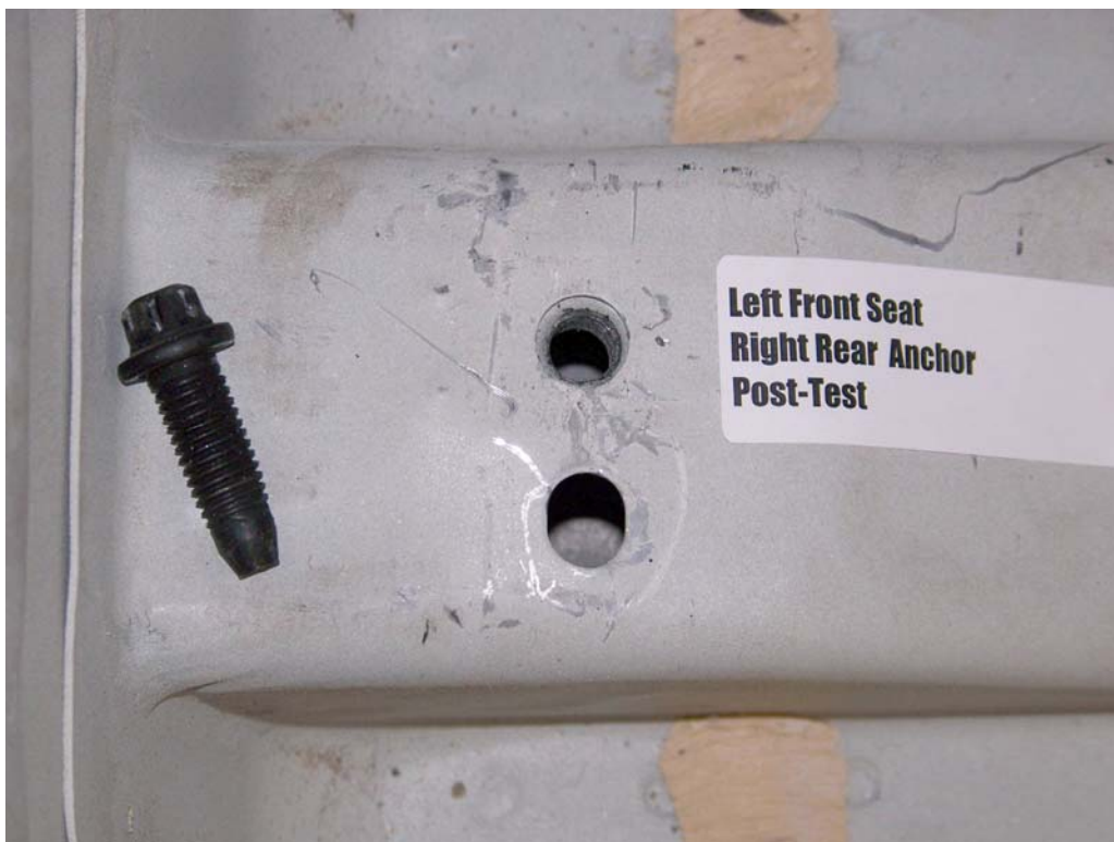
FIGURE 48. Floor Pan Anchor, P1, Post-Test
