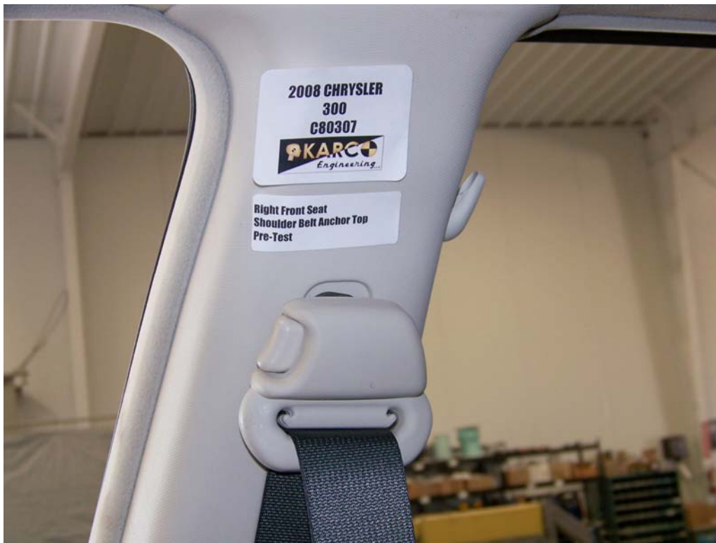
FIGURE 83. Shoulder Belt Anchor, P2, Pre-Test
