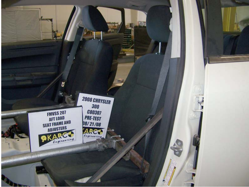
FIGURE 19. Aft Load on Seat Frame and Adjusters, P1, Pre-Test
