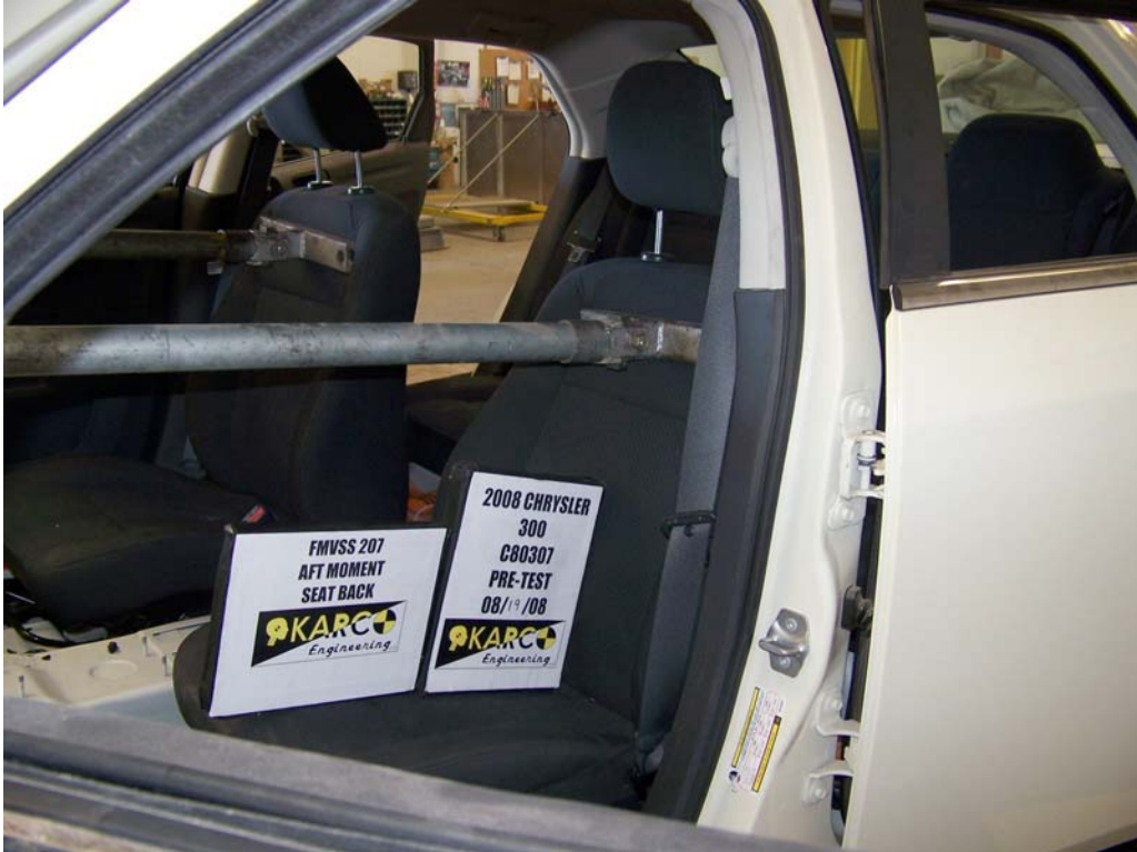
FIGURE 11. Aft Moment on Seat Back, P1, Pre-Test
