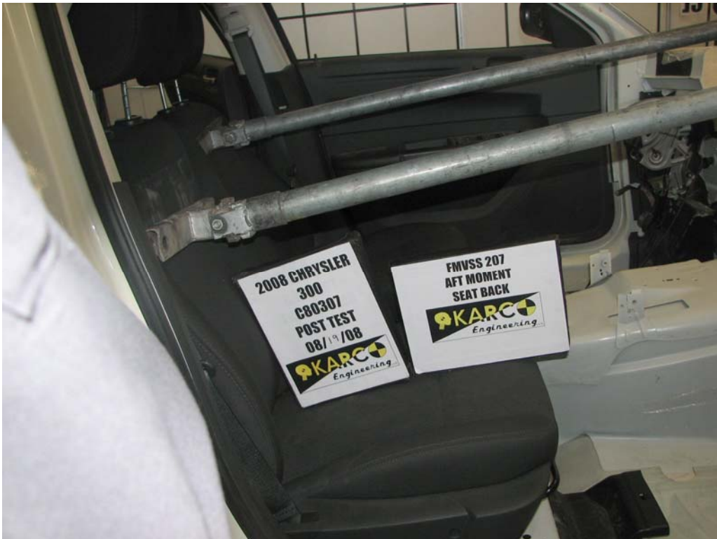
FIGURE 14. Aft Moment on Seat Back, P2, Post-Test
