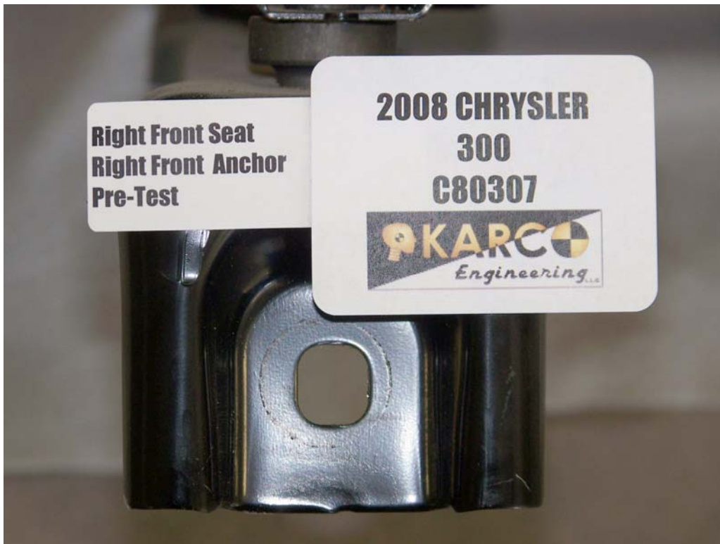
FIGURE 73. Seat Anchor, P2 , Pre-Test
