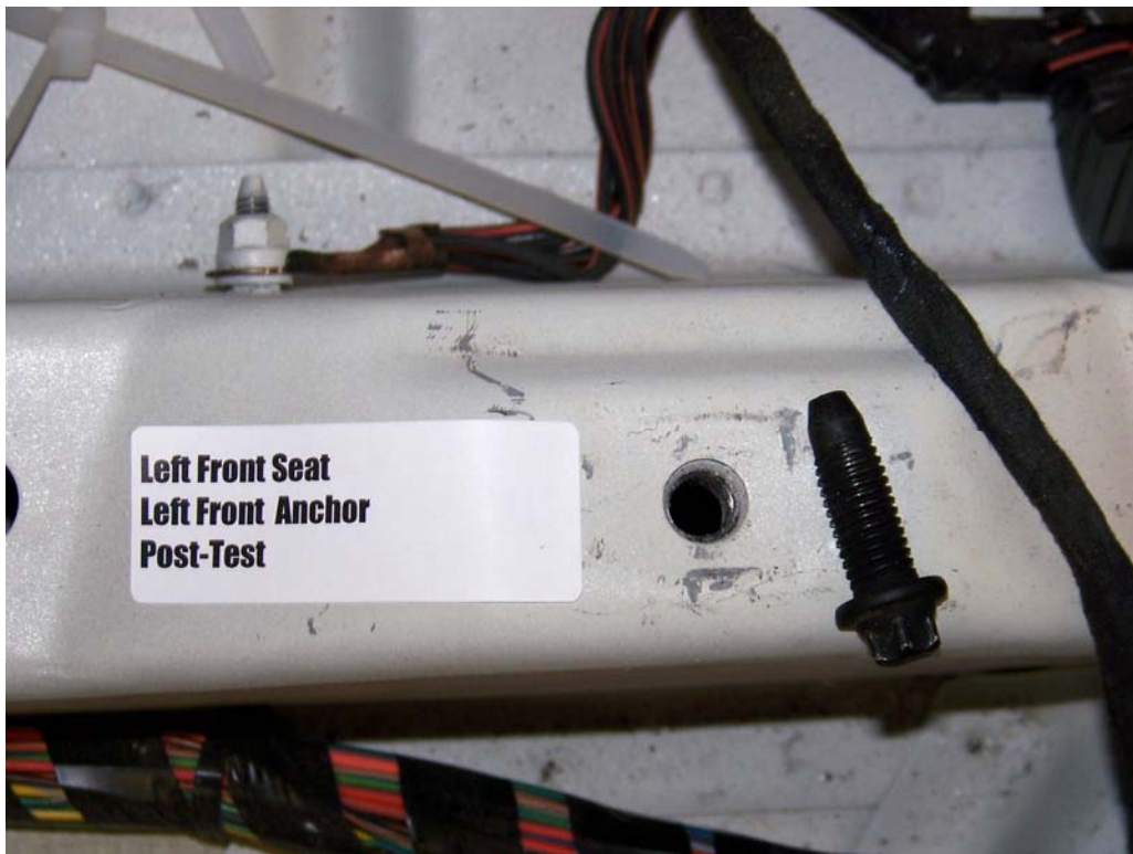
FIGURE 40. Floor Pan Anchor, P1, Post-Test
