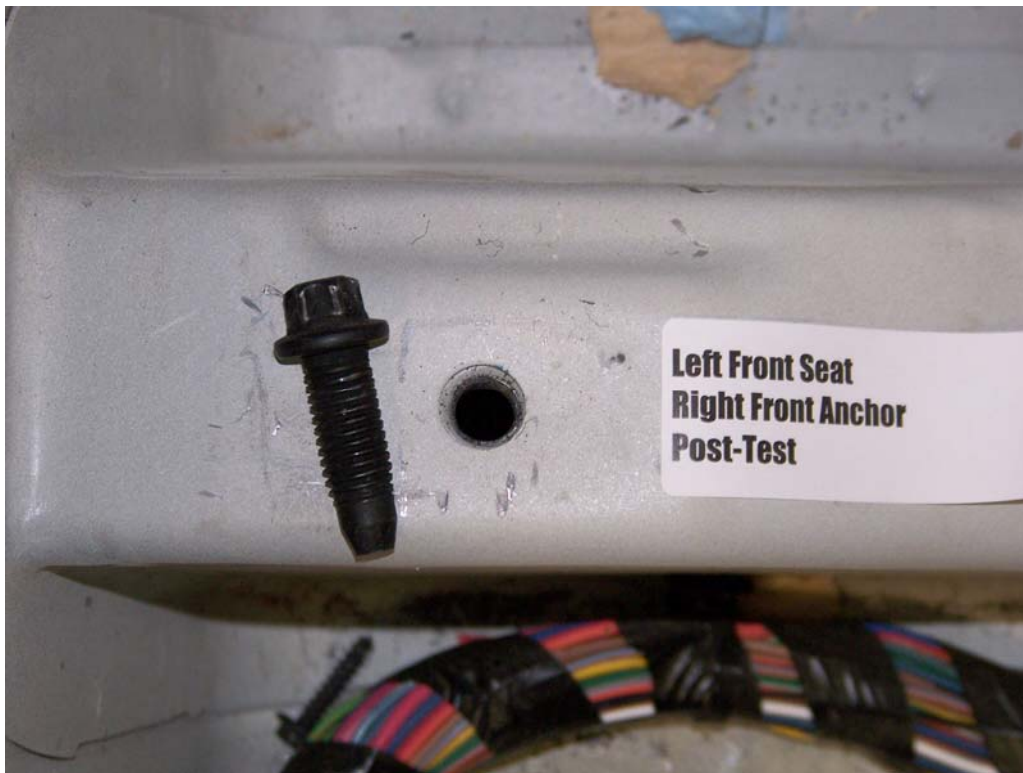
FIGURE 44. Floor Pan Anchor, P1, Post-Test
