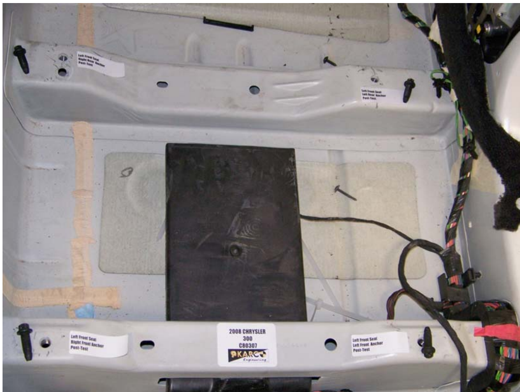
FIGURE 36. Floor Pan Anchors, P1 Overall, Post-Test
