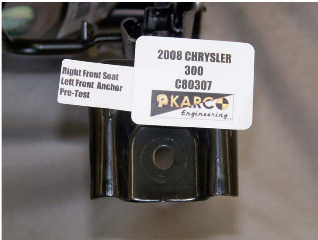
FIGURE 69. Seat Anchor, P2, Pre-Test
