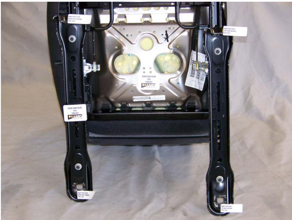
FIGURE 66. Seat Anchors, P2 Overall, Post-Test
