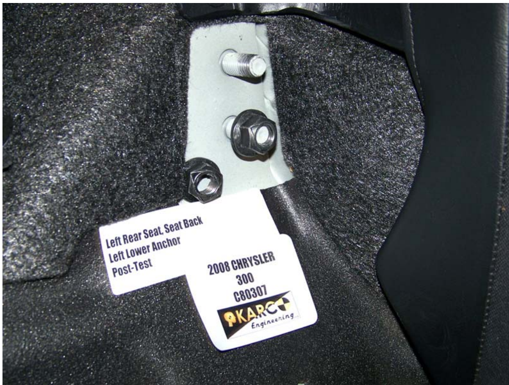
FIGURE 100. Floor Pan Anchor, P4, Post-Test
