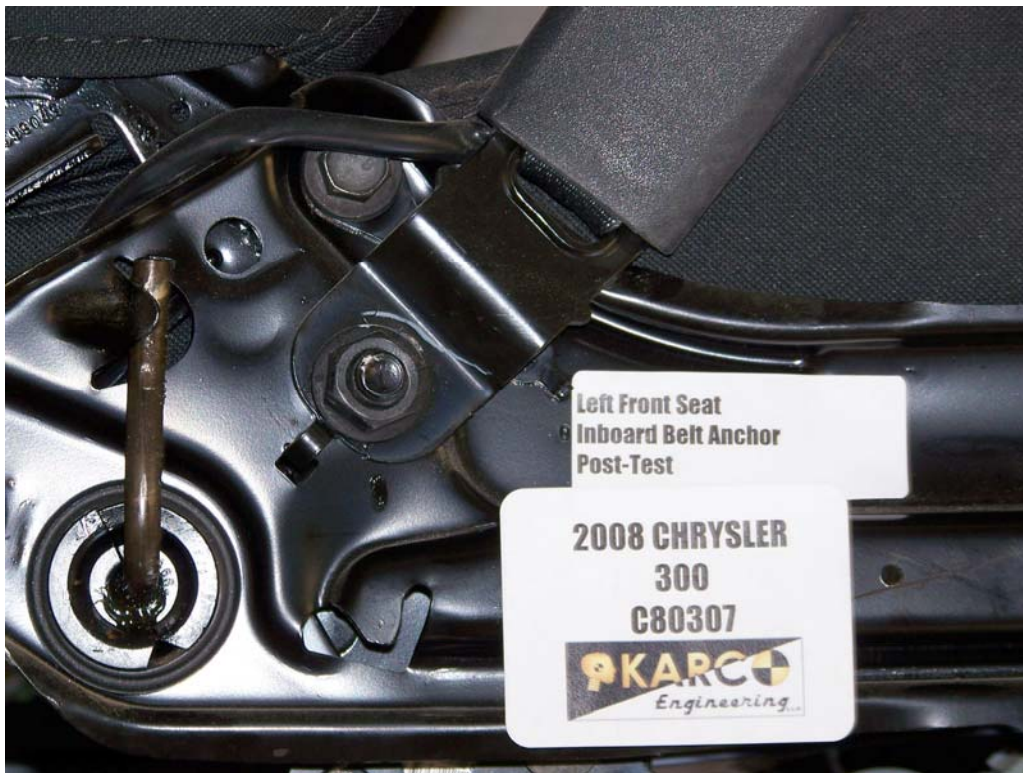
FIGURE 62. Belt Anchor, P1, Post-Test
