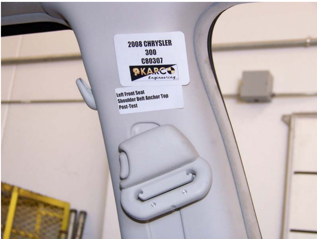
FIGURE 56. Shoulder Belt Anchor, P1, Post-Test
