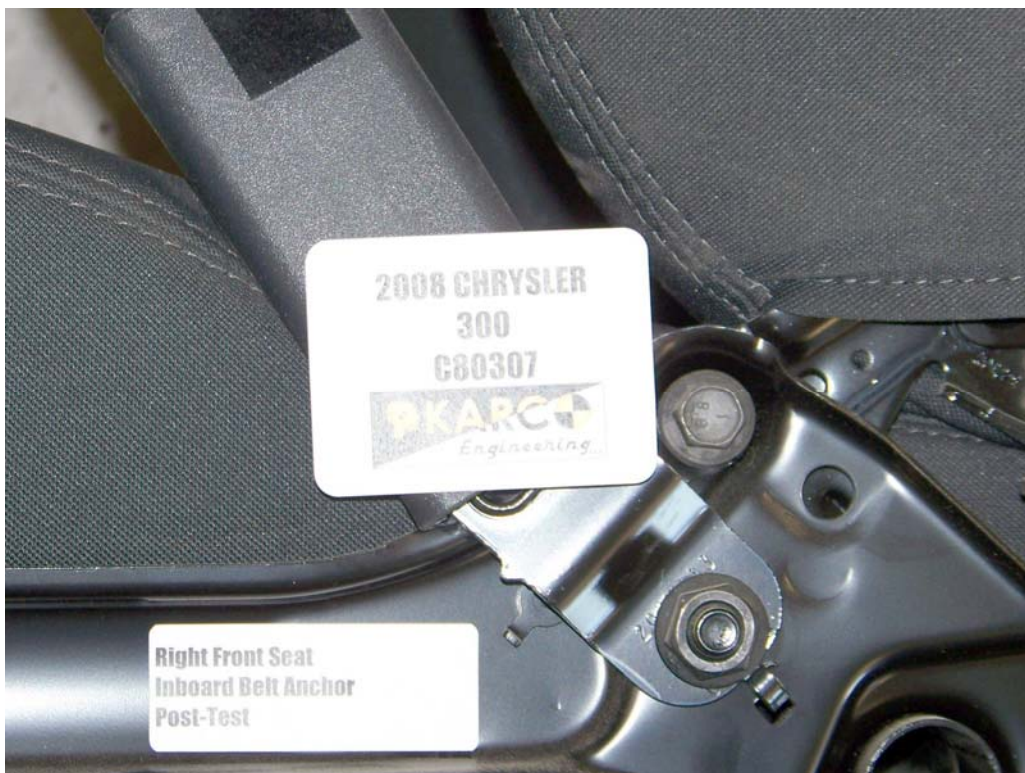
FIGURE 90. Belt Anchor, P2, Post-Test
