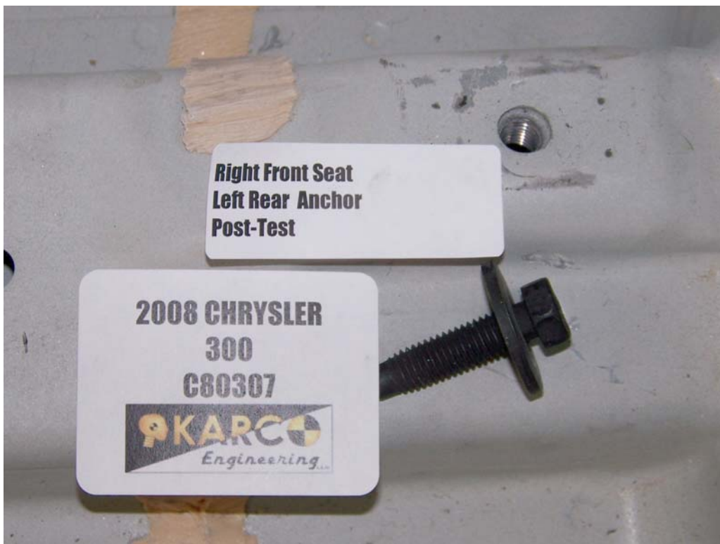
FIGURE 80. Floor Pan Anchor, P2, Post-Test
