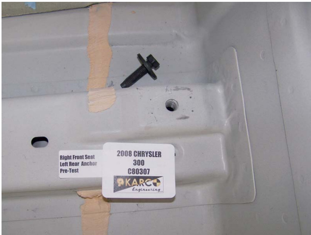
FIGURE 79. Floor Pan Anchor, P2, Pre-Test
