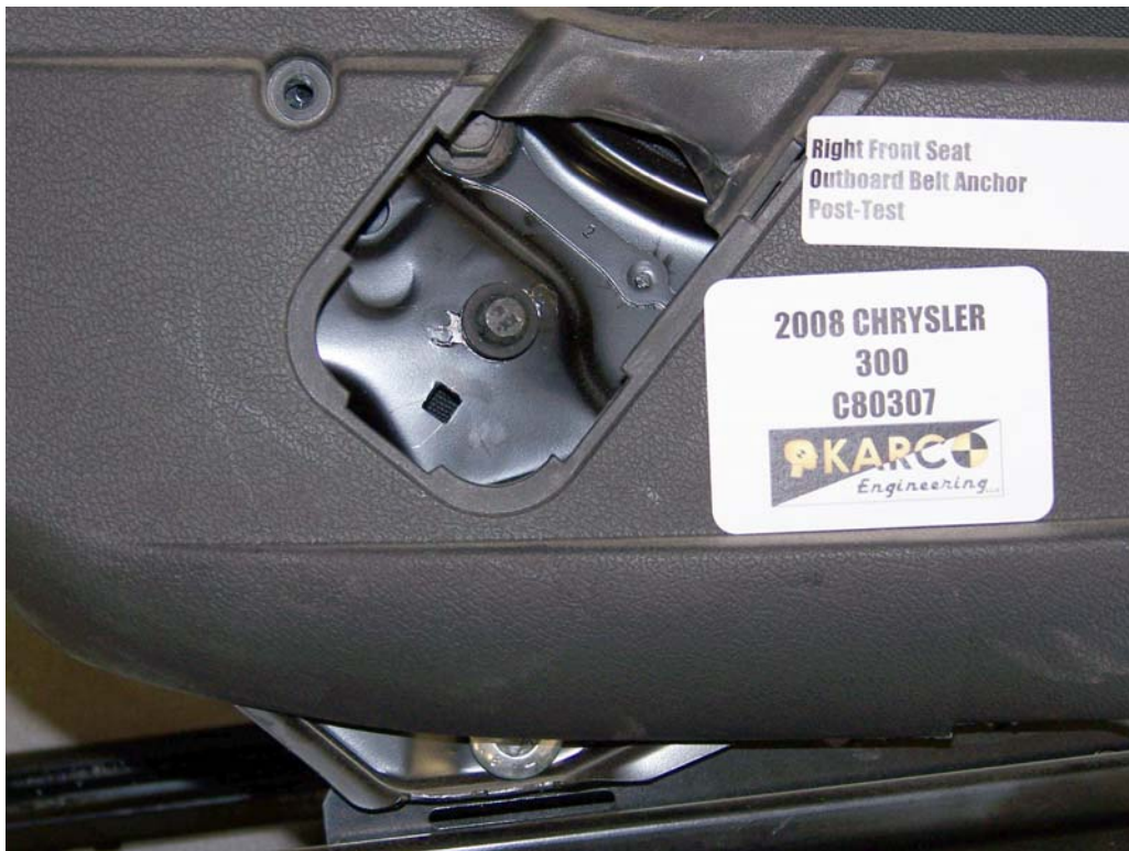
FIGURE 88. Belt Anchor, P2, Post-Test
