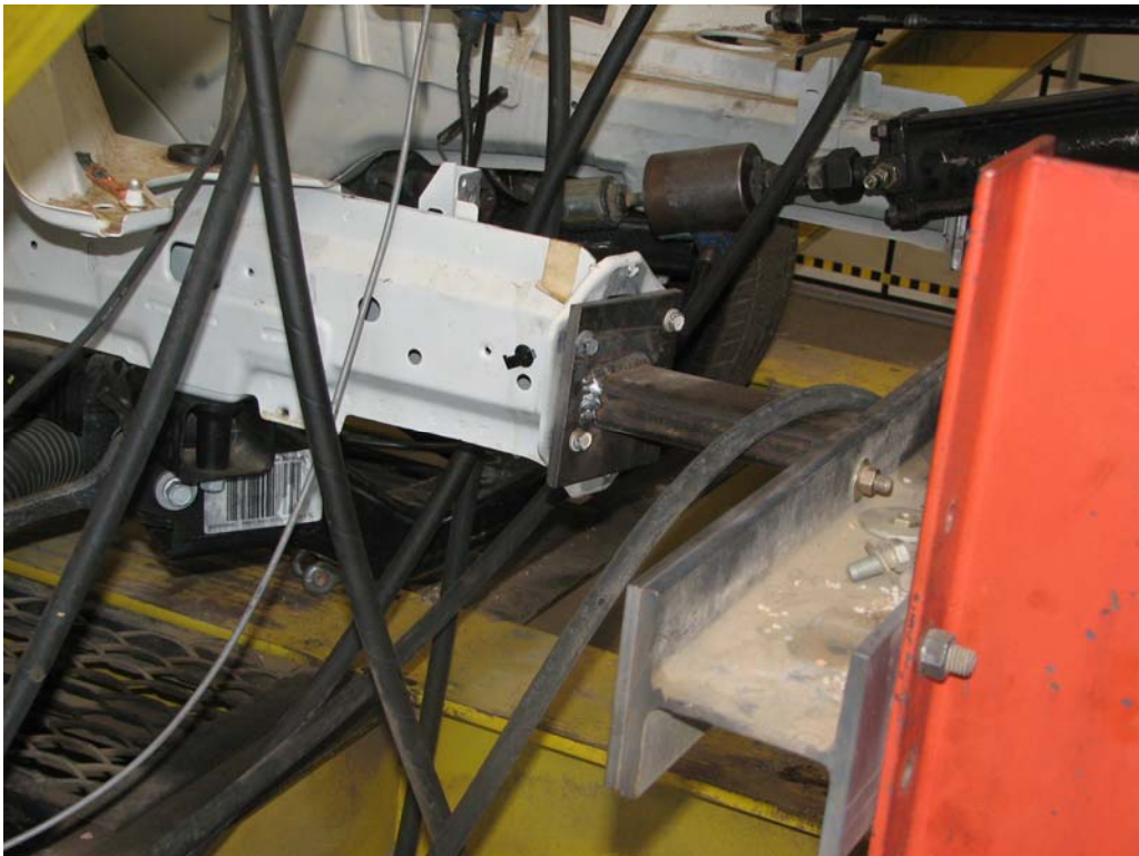
FIGURE 10. Vehicle Mounted in Test Fixture
