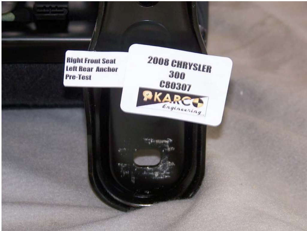
FIGURE 81. Seat Anchor, P2, Pre-Test
